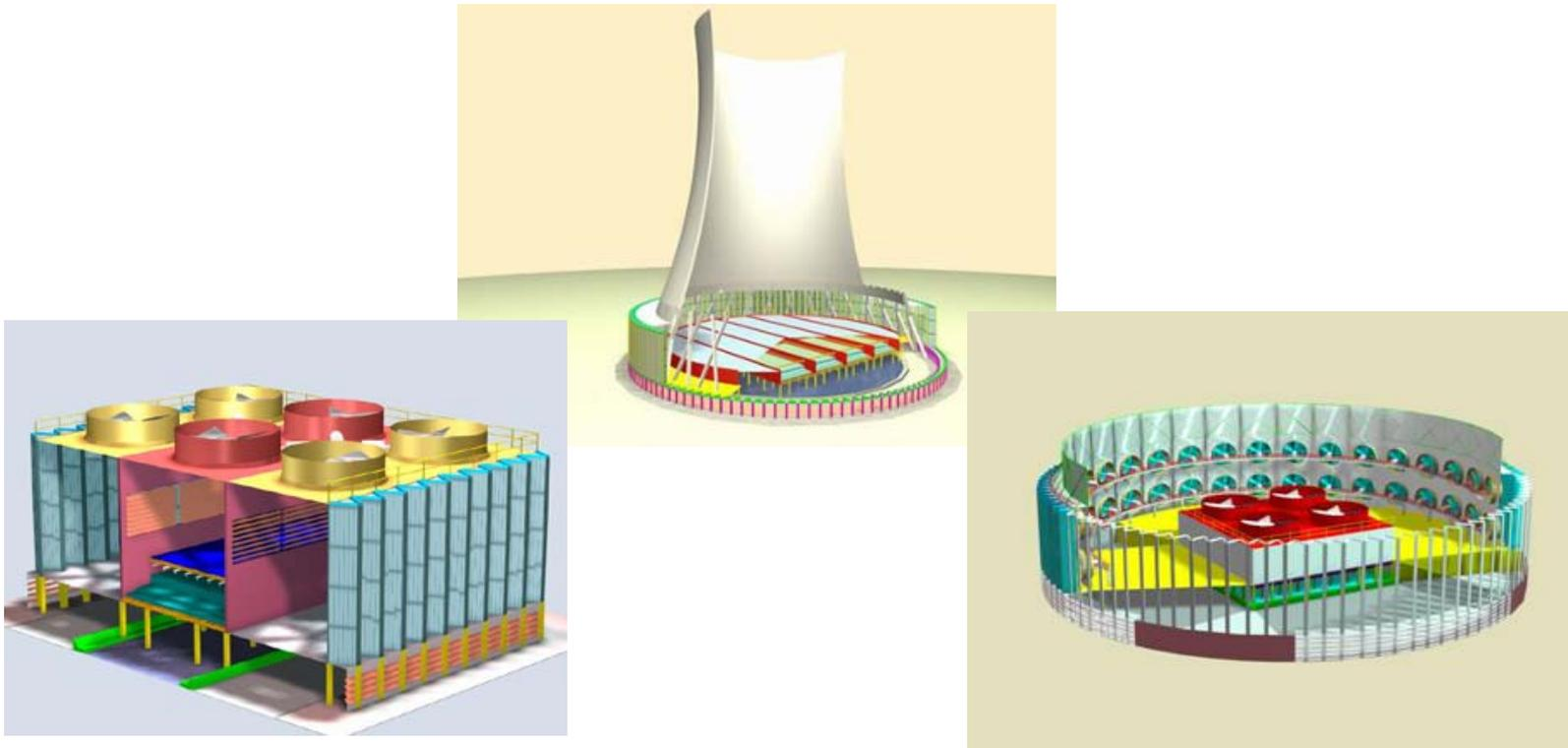
Conceptual designs for wet assisted HELLER Systems locating the assisting cells in the main dry cooling tower
