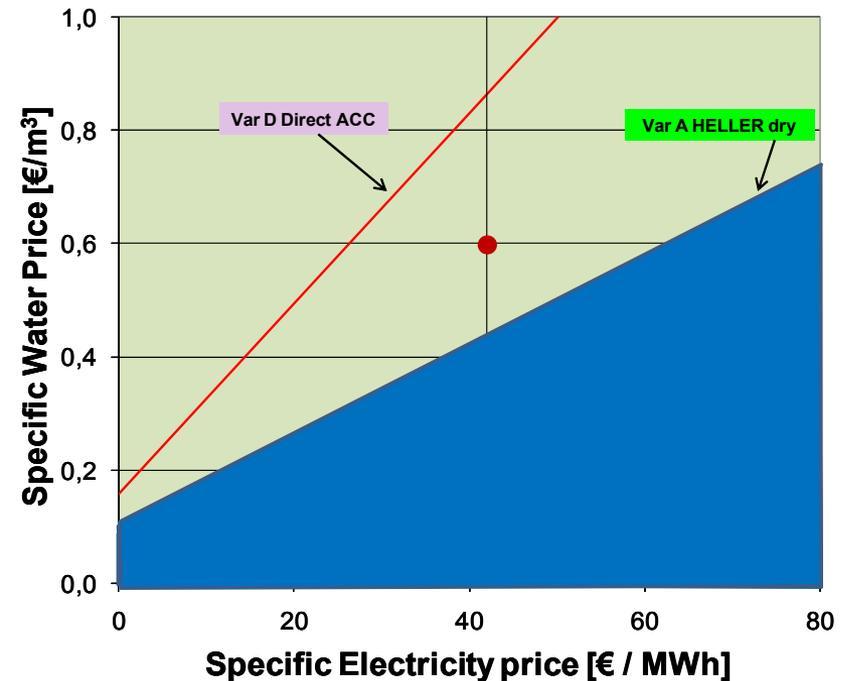
➤ The all-dry HELLER System (var. A) is competitive against wet cooling (var. E) - at an assumed water price of 0.6 €/m<sup>3</sup> – up to 63.5 €/MWh electricity selling price.
