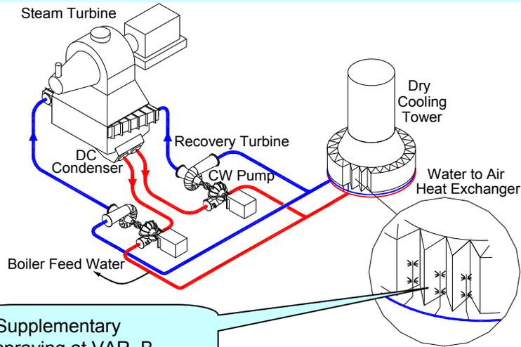
**Var.C.: HELLER System with Assisting Wet Cells**
