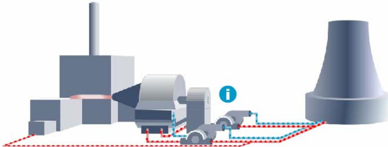
HELLER System is an indirect dry cooling plant. The power plant waste heat is initially exchanged in a condenser (preferably a direct contact one) to a closed cooling water circuit. The heat absorbed by the water is rejected to ambient air in fin tube type heat exchangers. Air moving can be either by natural or mechanical draft.
