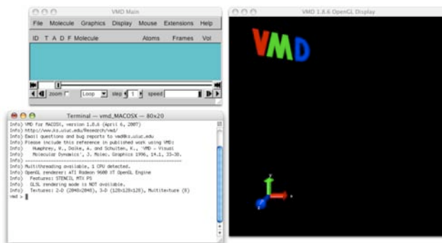
Figure 2: The VMD Main window, the OpenGL Display window, and the VMD Console window.
