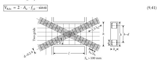
Figure 9.29 Arrangement of reinforcement in a coupling beam.
