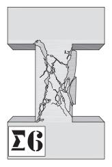
Figure 8.58 Premature explosive cleavage shear fracture of a short column. (Adapted from Tegos, I. 1984. Contribution to the study and improvement of earthquake-resistant mechanical properties of low slenderness structural elements. PhD thesis, Aristotle University of Thessaloniki (in Greek).)
