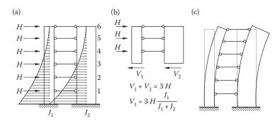
Figure 4.21 Action effects of shear (ductile) wall system under lateral loading (a) M – diagram; (b) equilibrium between shear and lateral loads; (c) storey displacements.
