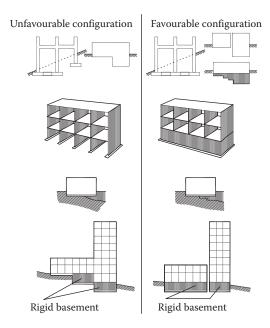
Figure 4.18 Unfavourable and favourable configuration of the foundation and the basement.
