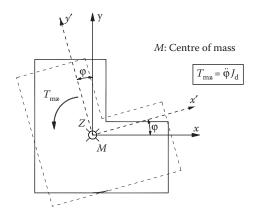
Figure 2.43 Torsional excitation of a pseudospatial single-storey system activated by a torque  $T_{mz}(t)$ .
