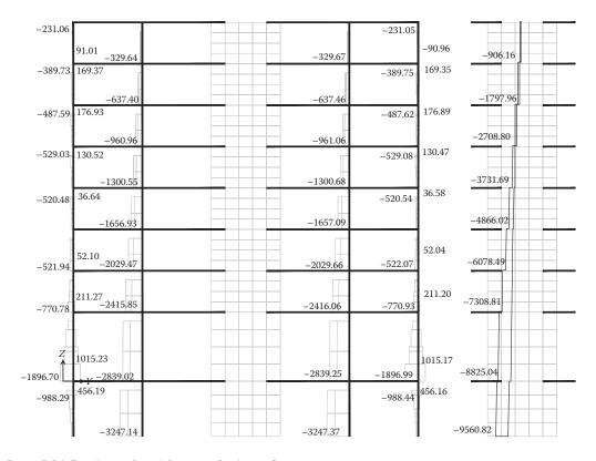
Figure 5.54 Envelope of axial forces - Grid axis C.
