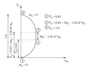
Figure 8.66  $\overline{\nu}_{\rm d}$  –  $v_{\rm Rd}$  interaction diagram.
