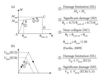
Figure 14.19 Safety verifications for primary elements: (a) ductile elements; (b) brittle elements.
