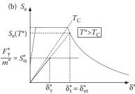
Figure 14.4 Determination of the target displacement for the equivalent SDOF system: (a) short period; (b) medium and long period.
