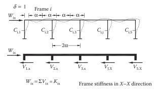
Figure 2.40 Definition of the stiffness  $K_{ix}$  of a frame i parallel to the x-x direction.
