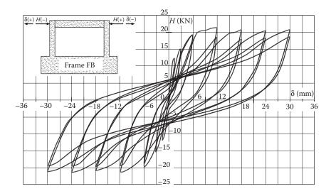
Figure 8.87 Lateral load-displacement loops. Bare frame FB. (Adapted from Stylianidis, K. 2012. Journal of O.C.B.T., 6, 194-212.)
