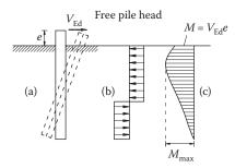
Figure 10.13 Short pile response to V<sub>Ed</sub> loading in cohesive soil: (a) load pattern—deflections; (b) soil reactions; (c) pile bending moments.
