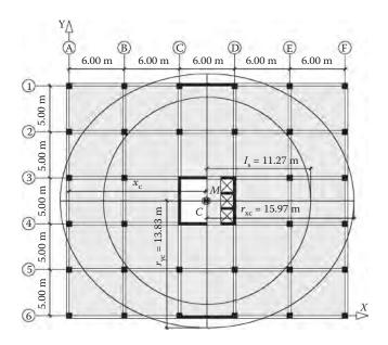
Figure 5.46 Definition of torsional rigidity.
