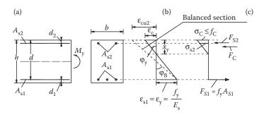
Figure 8.14 Cross section at yield: (a) geometry; (b) deformation pattern; (c) internal forces.
