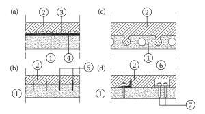
Figure 15.38 Details of connection of a new layer to the old concrete on a slab: (a) connection of new to old concrete using epoxy resin; (b) connection using epoxy bolts; (c) connection using existing voids of a voided slab; (d) connection using angle profiles; I = existing slab; 2 = new slab; 3 = sand corner; 4 = epoxy resin; 5 = epoxied bolts; 6 = angle profile; 7 = anchor bolts or shoot nails.
