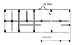
Figure 13.13 Example of 'unclear' structural layout.
