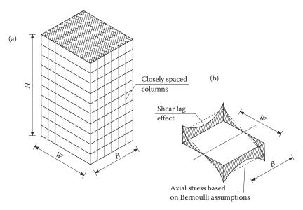
Figure 4.30 Framed system: (a) perspective view; (b) stress distribution under lateral loads. (Adapted from Elnashai, A.S. and Di Sarno, L. 2008. Fundamentals of Earthquake Engineering, Wiley, West Sussex, UK.)
