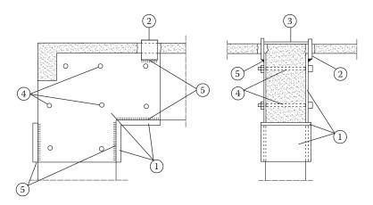
Figure 15.32 Bonded metal plates on a joint: I = steel plate; 2 = steel plate; 3 = steel strap; 4 = prestressed bolts; 5 = welding.
