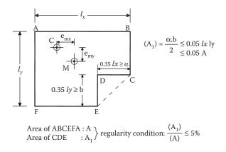
Figure 5.1 Condition of regularity at the re-entrant corner.
