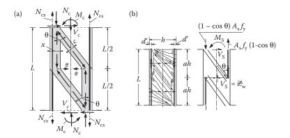
Figure 8.65 (a) The diagonal parallelogram strut model under compression; (b) the truss model with variable inclination struts.
