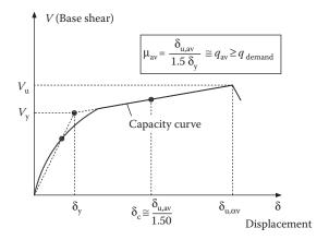
Figure 14.17 Determination of the q-factor value using the push-over capacity curve.
