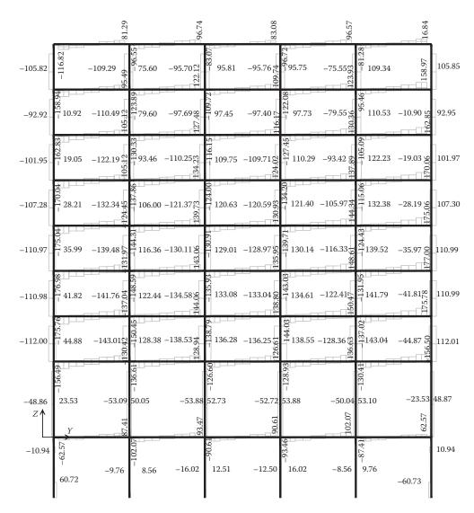
Figure 5.52 Envelope of shear forces - Grid axis B.
