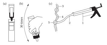
Figure 15.4 Procedure for the application of resin injections: (a) mixing of resin with the hardening agent; (b) shaking of the mixture for it to become homogeneous; (c) application of the resin injection: I = injection gun, 2 = plastic hose, 3 = crack, 4 = sealer, 5 = nipples.
