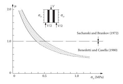
Figure 15.14 Friction coefficients for masonry as a function of the average normal stress.
