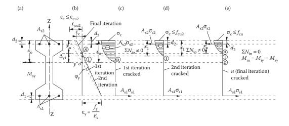
Figure 8.19 Cross section at yield stage (a) cross section; (b) deformation pattern at successive iteration steps 0.1, n; (c) internal forces of step (1); (d) internal forces of step (2); (e) internal forces of final step (n).
