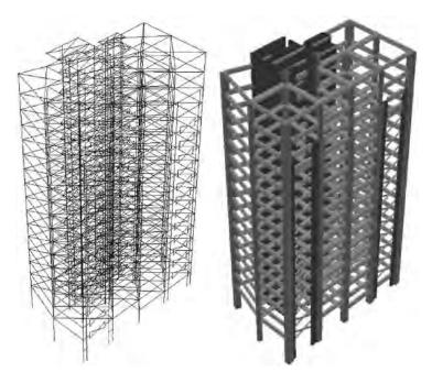
Figure 5.67 Finite element model of the 16-storey building.
