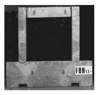
Figure 8.83 Failure modes of bare frame FBN<sub>I, I</sub>. with axial load on the columns. (Adapted from Stylianidis, K. 2012. Journal of O.C.B.T., 6, 194-212.)
