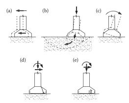
Figure 10.17 Modes of failure in pad foundations: (a) sliding failure; (b) soil-bearing capacity failure; (c) overturning; (d) shear failure in footing; (e) bending failure in footing. (Adapted from Booth, E. and Key, D. 2006. Earthquake Design Practice for Buildings. Thomas Telford Ltd.)
