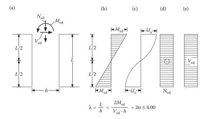
Figure 8.57 Squat column: M, N, V deflection diagrams; (a) geometry; (b) bending moments; (c) deflections; (d) axial forces; (e) shear forces.
