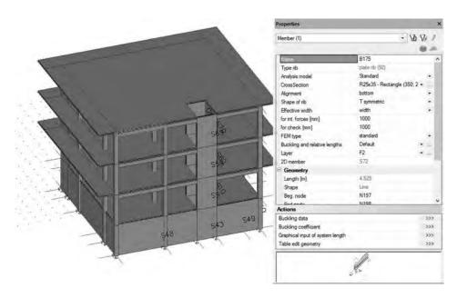
Figure 5.18 Modelling of ribs with 1-dimension finite element (I-DFE) and of effective flange width from slab 2-dimension finite element(2-DFE).
