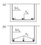
Figure 8.39 Arrangement of slicing bars in relation to the transverse reinforcement: (a) in a plane parallel to the bottom flange of the beams; (b) in planes vertical to the bottom flange.
