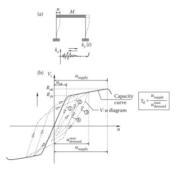
Figure 3.3 Displacement-based design based on inelastic dynamic analysis. (a) The structural system under seismic excitation; (b)  $V_i - U_i$  curve for seismic loads and capacity curve of the structure.
