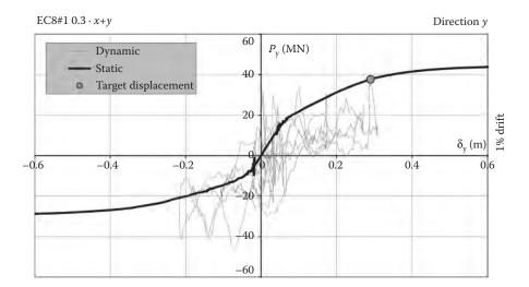
Figure 5.72 Global  $P-\delta$  comparison between static and dynamic analysis for the EC8#1 0.3 · x+y excitation.
