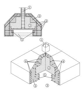
Figure 15.42 Strengthening of a footing without strengthening of the column: I = existing column; 2 = existing foundation; 3 = added concrete; 4 = added reinforcement; 5 = steel profile.
