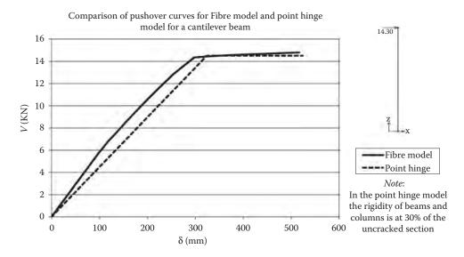
Figure 5.60 Pushover curves from point hinge and fibre model.
