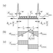
Figure 15.50 Intermediate crack-induced debonding: (a) stress-displacement pattern; (b) assumption for axial stress-strain distribution along the FRP laminate axis; (c) assumption for bond stress distribution along the contact surface.
