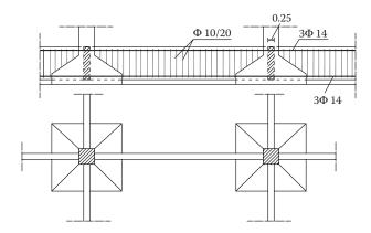
Figure 10.6 Independent footings with a tie-beams grillage.
