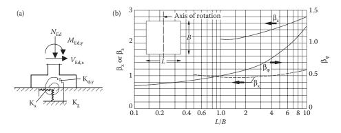
Figure 10.7 Load effects on a footing and stiffness simulation of the ground by elastic springs: (a) structural model; (b) coefficients  $\beta_x$ ,  $\beta_z$  and  $\beta_\phi$ , for estimating spring stiffness of rectangular footings. (From Dowrick, D. 2005. Earthquake Risk Reduction. Copyright Wiley-VCH Verlag GmbH & Co. KGaA. Reproduced with permission.)
