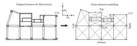
Figure 5.66 Typical storey plan view and modelling.
