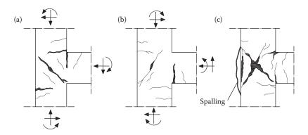
Figure 11.24 Failure of exterior joint in a multi-storey building: (a) moments inducing compression at the lower fibre of the beam; (b) moments inducing compression at the upper fibre of the beam; (c) cyclic bending moment loading.
