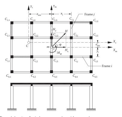
Figure 2.39 Plan and elevation of a single-storey pseudospatial structural system.
