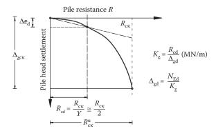
Figure 10.12 Determination of the axial spring stiffness of a pile from an  $R - \Delta z$  diagram.
