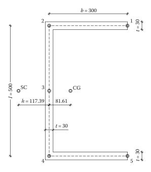
Figure 9.55 Centre of gravity (CG) and shear centre (SC) position.
