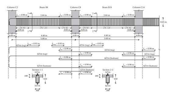
Figure 8.105 Flexural and shear reinforcement of beams 8 and 19.
