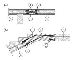
Figure 15.36 Local repair through the thickness of a slab: (a) repair in the span; (b) repair on the connection of a stair to the slab; I = added reinforcement; 2 = welding; 3 = added concrete; 4 = existing slab.
