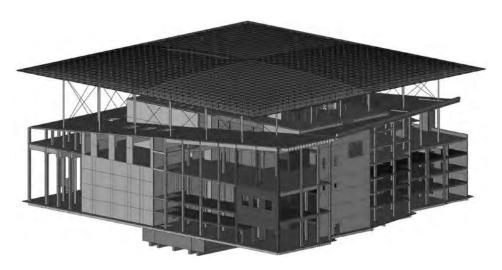
Figure 5.17 BIM application for the Athens Opera House (SNFCC) using Nemetschek Scia Engineer.
