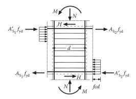
Figure 15.33 Schematic representation of the internal forces in a joint.
