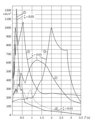
Figure 2.11 Characteristic acceleration spectra of strong earthquakes: (1) Bucharest earthquake 4.3.1977 N-S; (2) El Centro earthquake 18.5.1940 N-S; (3) Mexico City earthquake 19.9.1985 E-W SCI; (4) Thessaloniki earthquake 20.6.1988 E-W 'City' hotel; (5) Athens earthquake 07.09.1999.
