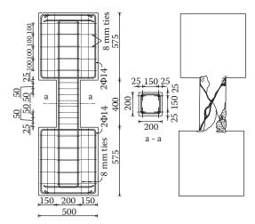
Figure 8.59 Conventional reinforcement of short columns against shear (close spaced ties).
