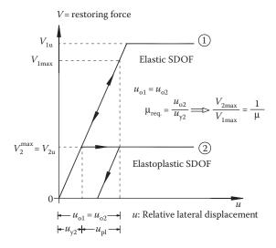
Figure 2.26 An alternative quantitative relation between elastic and elastoplastic response in an SDOF system.
