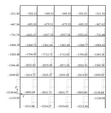
Figure 5.51 Envelope of axial forces - Grid axis B.
