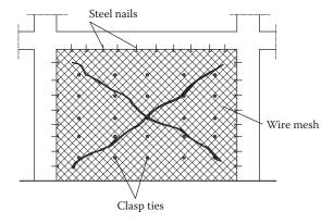
Figure 15.44 Repair of a seriously damaged infill masonry wall.
