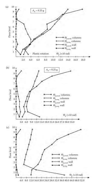
Figure 5.15 Required (demand) and available (supply) rotational capacities in a 10-storey dual structure designed for different ductility levels: (a) DCL; (b) DCM; (c) DCH. (From Penelis, G.G. and Kappos, A.J. 1997. Earthquake-Resistant Concrete Structures. SPON E&FN (Chapman & Hall), London.)
