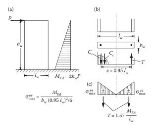
Figure 9.37 (a) Loading pattern of an orthogonal wall and bending moment diagram; (b) dimensioning of the wall as a linear member; (c) dimensioning of the wall using FEM method.
