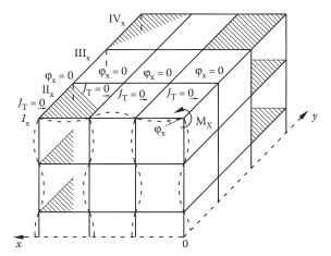
Figure 2.38 Pseudospatial system with parallel plane frames with no strain interaction between them due to the zero torsional stiffness of the connecting beams.
