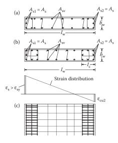
Figure 9.9 Dimensioning of slender ductile walls to bending with axial force: (a) main reinforcement  $A_s$  concentrated at the boundaries; (b) main reinforcement  $A_s$  concentrated in confined boundary elements; (c) concept of plane strain distribution.
