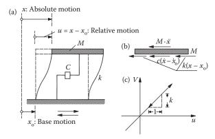
Figure 2.2 Single-degree-of freedom (SDOF) system excited by the base motion: (a) response of the system; (b) dynamic equilibrium condition; (c) shear force versus relative displacement diagram for the columns.
