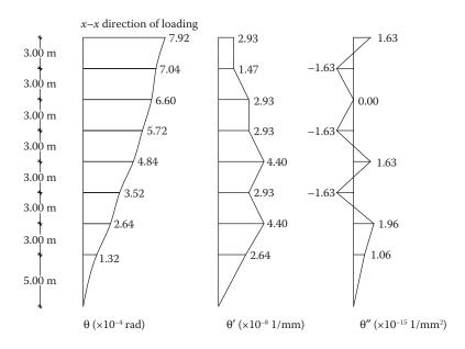
Figure 9.57 Rotation angle,  $\theta_i$ ,  $\theta_i^{\prime}$  and  $\theta_i^{\prime\prime}$  profile along building height for the x-x direction of loading.
