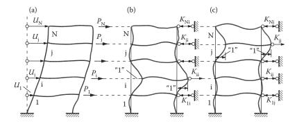
Figure 2.34 Determination of the vectors of the stiffness matrix  $K(K_i \text{ and } K_i)$ .
