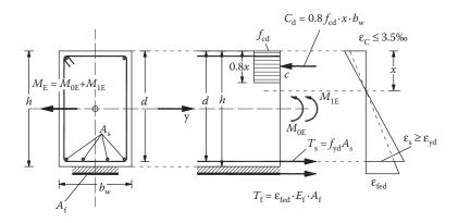
Figure 15.46 Strengthening of a beam under flexure using FRP laminates.
