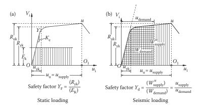
Figure 3.2 The main concept for safety verifications for (a) static loads, and (b) seismic loads.
