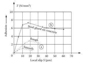
Figure 15.15 Constitutive law of adhesion: (a) concrete-to-concrete through bonding agent (Hanson, 1960); (b) steel sheets glued to concrete by means of epoxy resin (Ladner and Weber, 1981).
