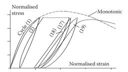
Figure 7.5  $\sigma$ - $\epsilon$  diagram of concrete under cyclic uniaxial compression. (Adapted from Karsan, I.D. and Jirsa, J.O. 1969. Journal of the Structural. Division, ASCE 95(ST 12), 2543-2563.)
