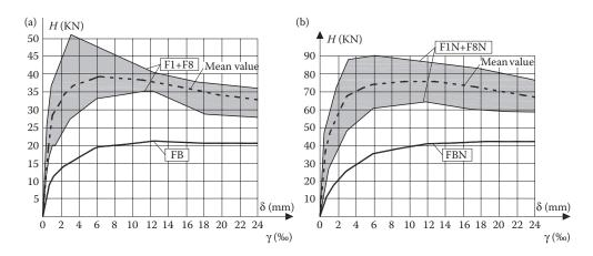
Figure 8.89 Program #1. Lateral load—displacement envelopes: (a) models without axial force; (b) models with axial force. First cycles only. (Adapted from Stylianidis, K. 2012. Journal of O.C.B.T., 6, 194–212.)
