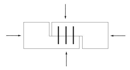
Figure 15.16 Clamping effect of steel across interfaces.
