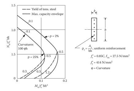
Figure 9.8 Axial load-moment interaction curves for rectangular uniformly reinforced concrete walls. (After Salse and Fintel, 1973; From Dowrick, D. 2005. Earthquake Risk Reduction. Copyright Wiley-VCH Verlag GmbH & Co. KGaA. Reproduced with permission.)
