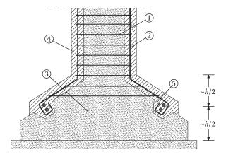
Figure 15.39 The end of a column jacket in the footing:  $I = \text{new ties } \Phi 12/100 \text{ mm}$ ; 2 = longitudinal reinforcing bars; 3 = existing concrete; 4 = added concrete; 5 = dowel in old concrete.
