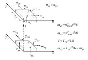
Figure 9.36 Notation for internal forces of a 'disk' and a 'shell'.
