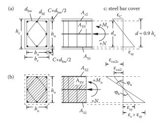
Figure 8.52 Confinement for a quantified local ductility in the case of columns: (a) notations of the cross section; (b) notation of the confined core.
