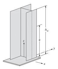
Figure 9.41 H-section core. (Adapted from Taranath, B.S. 2010. Reinforced Concrete Design of Tall Buildings, CRC Press (Taylor & Francis Group).)
