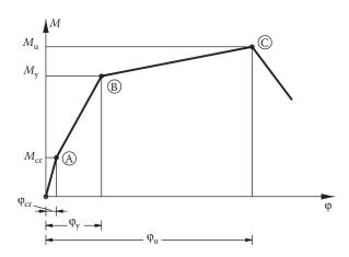
Figure 8.12 M-φ diagram for normally reinforced cross section.
