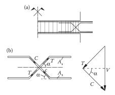
Figure 8.36 X-shaped type of reinforcement for beams with high shear: (a) arrangement of shear reinforcement; (b) design of the x-shaped diagonal reinforcement.
