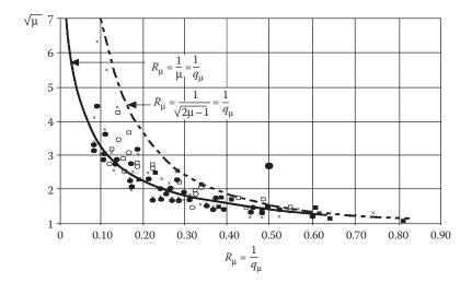
Figure 2.28 Force reduction factor  $R_u$  or  $(I/q_u)$  versus  $\sqrt{\mu}$ .
