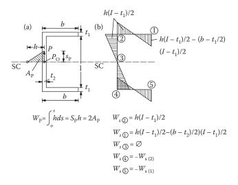
Figure 9.46 Determination of the principal warping ordinate w(s): (a) definition of w(s); (b) w(s) diagram of a C section.
