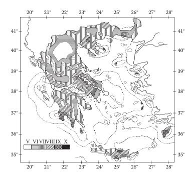
Figure 3.12 Maximum observed intensities in Greece between 1700 and 1981 on the MM scale.
