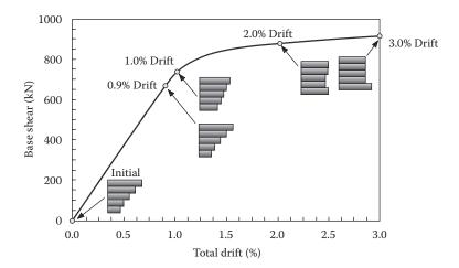
Figure 14.2 Changes of the distribution of an inertially framed building (adaptive force distribution). (From Elnashai, A.S. and Di Sarno, L. 2008. Fundamentals of Earthquake Engineering. Copyright Wiley-VCH Verlag GmbH & Co. KGaA. Reproduced with permission.)
