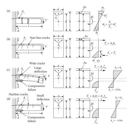
Figure 8.10 Successive steps of loading to failure of a beam under flexure: (a) stage I (uncracked); (b) stage II (cracked tensile zone); (c) failure due to steel yield (normally reinforced beam); (d) failure due to compression failure of concrete before steel yield (over-reinforced beam).
