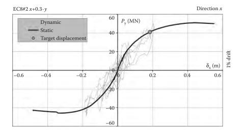
Figure 5.71 Global  $P-\delta$  comparison between static and dynamic analysis for the EC8#2  $x+0.3 \cdot y$  excitation.
