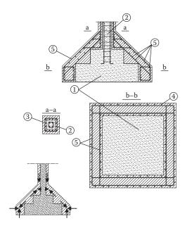
Figure 15.41 Strengthening of footing – column: I = existing foundation; 2 = existing column; 3 = reinforced jacket; 4 = added concrete; 5 = added reinforcement.
