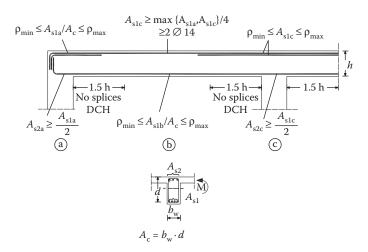
Figure 8.34 Arrangement of longitudinal reinforcement in earthquake-resistant R/C beams.
