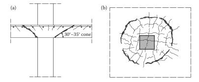
Figure 11.29 Damage at a slab-to-column connection: (a) section; (b) top side of the slab.
