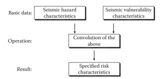
Figure 16.1 Evaluation of specific seismic risk.
