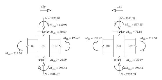
Figure 8.101 Capacity design moments for column C8.
