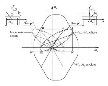
Figure 5.43 Choice of the proper ellipse (group I or group II) in regard to the position of the gravity load effects vector  $\overline{r_0}$  in the quarters of the capacity envelope of a unisymmetric cross-section.
