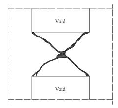
Figure 11.22 Shear failure of a shear wall coupling beam.
