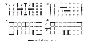
Figure 15.56 Addition of new R/C walls inside a frame or skeleton structure: (a), (b), (c) favourable layout (symmetric); (d) unfavourable layout (eccentric walls).
