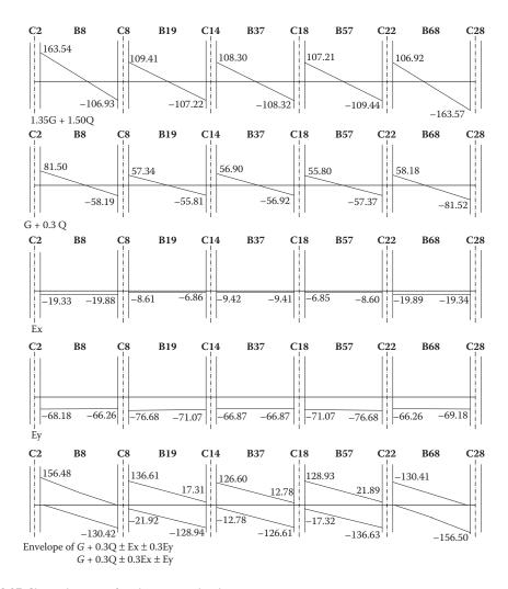
Figure 8.97 Shear diagrams for the various loading cases.
