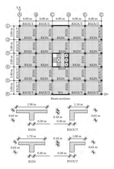
Figure 5.48 Beam sections and effective widths.
