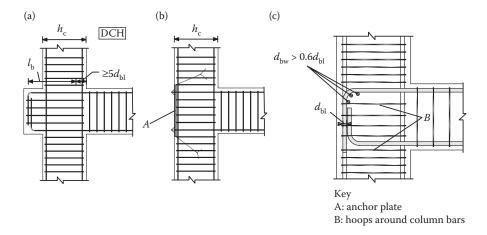
Figure 8.38 Additional measures for anchorage in exterior beam—column joints: (a) beam extension; (b) anchorage plate; (c) bonds and transverse reinforcement. (Adapted from E.C.8-I/EN1998-1. 2004. Design of Structures for Earthquake Resistance: General Rules, Seismic Actions and Rules for Buildings. CEN, Brussels, Belgium.)
