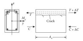
Figure 7.27 Longitudinal cracks due to bonding failure in the case of deformed steel rebars.
