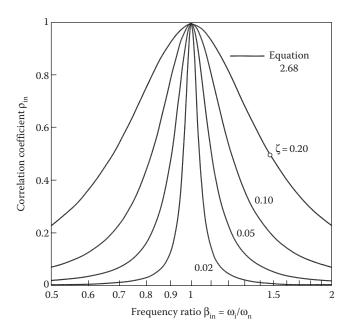
Figure 2.36 Variation of correlation coefficient p<sub>in</sub> given by Equation 2.68. (Adapted from Chopra, A.K. 2001. Dynamics of Structures: Theory and Application in Earthquake Engineering, 2nd Edition. Prentice-Hall, New Jersey.)
