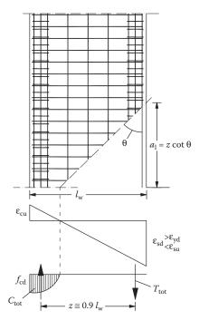
Figure 6.9 Tension  $T_{\rm tot}$  shift mechanism in slender ductile walls.
