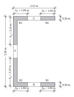
Figure 9.53 Definition of boundary elements.
