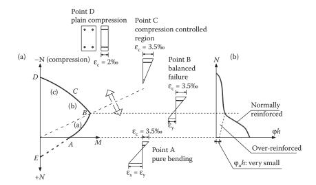
Figure 8.40 (a) M-N interaction diagram for an orthogonal symmetrically reinforced cross section of a column and relevant strain patterns; (b) qualitative presentation of ductility capacity in relation to N. (Adapted from Zararis, P. 2002. Design Methods of Reinforced Concrete (in Greek). Kyriakides Bros. Ltd, Thessaloniki.)
