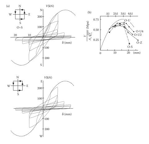
Figure 8.54 Square-like cyclic loading of columns: (a) hysteresis loops in each direction; (b) envelope of the resultant action. (Adapted from Jirsa, J.O., Maruyama, K. and Ramirez, H. 1980. The influence of load history on the shear behaviour of short RG columns. Proceedings of the 7th World Conference on Earthquake Engineering, Istanbul, 6, 339–146.)
