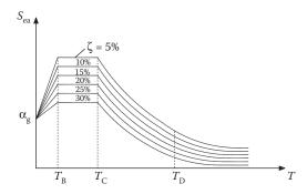
Figure 14.6 Family of demand spectra in standard S<sub>ea</sub> versus T format.
