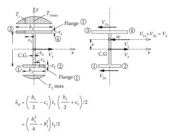
Figure 9.43 Shear diagrams due to  $V_X$ . The meaning of shear centre SC.
