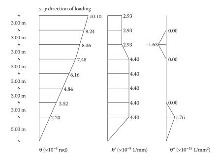
Figure 9.58 Rotation angle,  $\theta_i$ ,  $\theta_i'$  and  $\theta_i''$  profile along building height for the y-y direction of loading.
