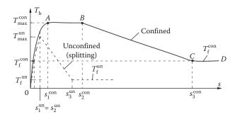
Figure 7.30 Idealised diagram of  $\tau_b$  – s according to Model Code 1990. (Adapted from CEB 1993. CEB-FIP Model Code 1990, Bulletin d'Information, CEB, 213/214, Lausanne.)
