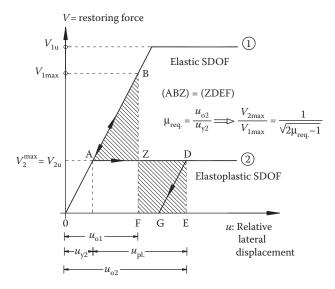
Figure 2.24 Quantitative relation between elastic and elastoplastic response of an SDOF system to an earthquake.
