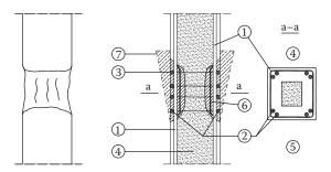
Figure 15.18 Column repair in the case of superficial damage: I = existing reinforcement; 2 = added new reinforcement; 3 = added new ties; 4 = existing concrete; 5 = new concrete; 6 = welding; 7 = temporary cast form.
