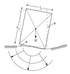
Figure 9.33 Rocking of large, lightly reinforced walls.
