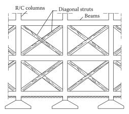
Figure 12.12 Bracing with diagonal struts.
