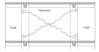
Figure 11.10 Damage in columns in contact with masonry on one side only.
