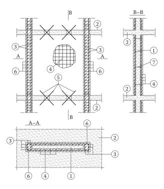
Figure 15.35 General arrangement for the strengthening of a wall: I = existing wall; 2 = existing slab; 3 = added longitudinal reinforcement; 4 = added wire fabric; 5 = diagonal connecting bars; 6 = added ties, 7 = connecting ties.
