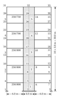
Figure 5.14 Ten-storey dual R/C system designed to EC8. (From Penelis, G.G. and Kappos, A.J. 1997. Earthquake-Resistant Concrete Structures. SPON E&FN (Chapman & Hall), London.)
