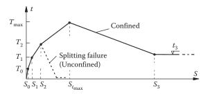
Figure 7.29 Idealised diagram of τ<sub>b</sub> – s. (Adapted from Eligehausen, R., Popov, E.P. and Bertero, V.V. 1983. Local bond stress-slip relationships of deformed bars under generalized excitations. Report EERC-83/23, Univ. of California, Berkeley; Penelis, G.G. and Kappos, A.J. 1997. Earthquake-Resistant Concrete Structures. SPON E&FN (Chapman & Hall), London.)
