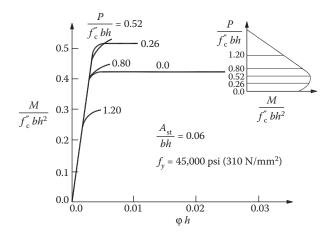
Figure 8.45 Moment—curvature curves for column sections at various levels of axial load. (From Park, R.andPaulay, T. 1975. Reinforced Concrete Structures. Copyright Wiley-VCHVerlag GmbH&Co. KGaA. Reproduced with permission.)
