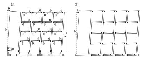
Figure 10.3 Dissipative mechanisms accepted by the Code: (a) dissipative superstructure—non-dissipative foundation mechanism (recomented); (b) dissipative superstructure—dissipative foundations mechanism. (With kind permission from Springer Science+Business Media: Fardis, M.N. 2009. Seismic Design, Assessment and Retrofitting of Concrete Buildings.)
