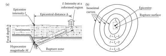
Figure 3.11 Terminology related to earthquakes (a) generation and propagation; (b) isoseismic curves.
