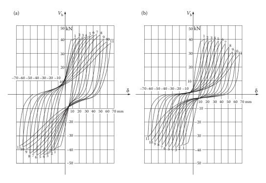
Figure 8.82 Hysteresis loops for exterior beam-column joints: (a) with x-shaped bars; (b) with conventional reinforcement.
