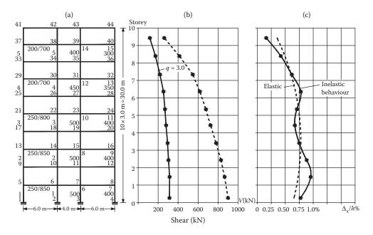
Figure 3.6 Comparison of shear forces and drifts ratios (interstorey deflections/storey height) of inelastic and elastic response at a typical ten-storey building: (a) structural system; (b) shear forces; (c) drift-ratios. (Adapted from Penelis, G.G. and Kappos, A.J. 1997. Earthquake-Resistant Concrete Structures. SPON E&FN (Chapman & Hall), London.)
