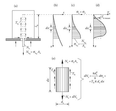
Figure 7.25 Bond shear stress distribution at the pull-out test: (a) experimental layout; (b) rebar slip; (c) tensile stresses at rebar; (d) bond stresses; (e) stress pattern at a differential element dx of the rebar.
