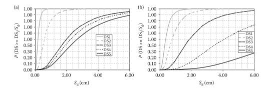
Figure 16.9  $S_d$ -based fragility curves for medium-rise infilled frames, low (a) and high (b) code design. (With kind permission from Springer Science+Business Media: Kappos, A. et al. 2006b. A hybrid method for the vulnerability assessment of R/C and URM buildings. Bulletin of Earthquake Engineering, 4, 391–413.)
