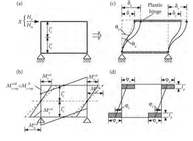
Figure 5.10 Moment—curvature displacement diagrams for R/C frames with strong beams—weak columns:
