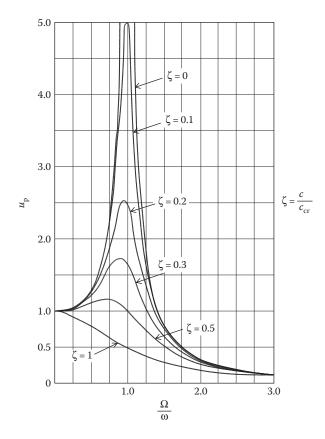
Figure 2.7 Maximum relative displacement  $u_p$  of an SDOF system activated by a sinusoidal forced vibration diagram of  $u_p$  versus natural frequencies ratio  $\Omega/\omega$  for various values of  $\zeta$  (critical damping ratio). (From Biggs, J.M. 1964. Introduction to Structural Dynamics. McGraw-Hill, New York. With permission.)
