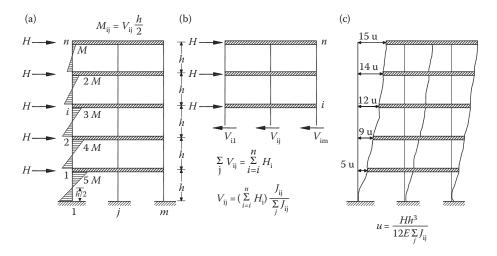
Figure 4.19 Action effects on shear frames under lateral loading; (a) M – diagram; (b) equilibrium between shear and lateral loads; (c) storey displacements.
