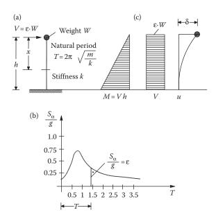
Figure 2.13 Transition from the dynamic to static response: (a) an SDOF system; (b) acceleration response spectrum; (c) maximum response of the structure.
