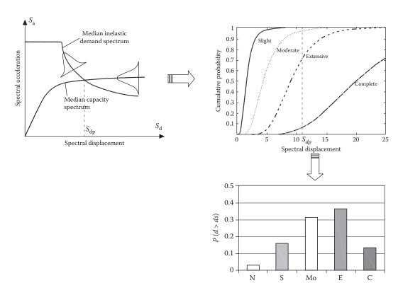
Figure 16.17 Damage estimate process. N, none; Mi, minor; Mo, moderate; S, severe; C, collapse. (With kind permission from Springer Science+Business Media: Erdik et al., 2010.)
