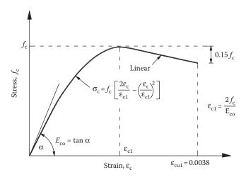
Figure 7.2 Idealised stress-strain curve for concrete under uniaxial compression. (Adapted from Park, R. and Paulay, T. 1975. Reinforced Concrete Structures. Copyright Wiley-VCH Verlag GmbH & Co. KGaA. Reproduced with permission.)
