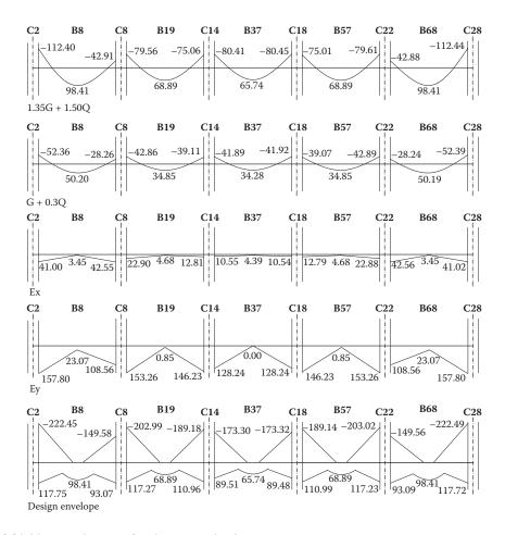
Figure 8.96 Moment diagrams for the various loading cases.
