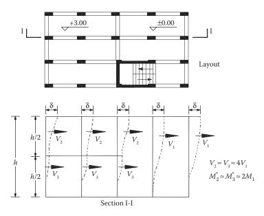
Figure 4.9 Concentration of large shear forces on short mezzanine columns.
