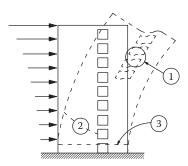
Figure 9.28 Critical areas of behaviour in coupled shear walls. (Adapted from Park, R. and Paulay, T. 1975. Reinforced Concrete Structures. J. Wiley & Sons, New York.)
