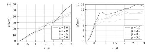
Figure 2.32 Inelastic displacement response spectra for mean alluvial ground layers in the United States (a) and in Greece (b). (Adapted from Kappos, A.J. and Kyriakakis, P. 2001. Soil Dynamics and Earthquake Engineering, 20, 111–123.)
