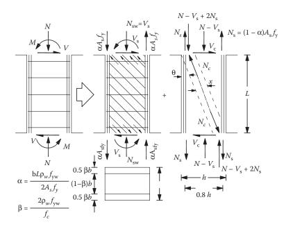
Figure 8.62 The superposition of two mechanical models (truss mechanism + diagonal strut mechanism [with tensile chords]) according to Shohara and Kato (1981) for shear design of short columns. (Adapted from Tegos, I. 1984. Contribution to the study and improvement of earthquake-resistant mechanical properties of low slenderness structural elements, PhD thesis, Aristotle University of Thessaloniki (in Greek).)
