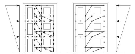
Figure 9.34 A strut-and-tie model for the shear design of a large, lightly reinforced wall.
