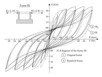
Figure 15.17 H- $\delta$  diagram of the original frame and then when repaired with epoxy resin injections.
