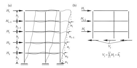
Figure 4.26 Displacement patterns of a plane frame under lateral loading (a) notation; (b) equilibrium of horizontal forces.
