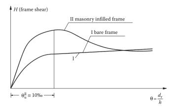
Figure 6.14  $H - \theta$  diagram of a masonry-infilled frame.
