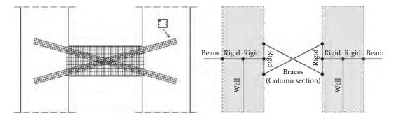
Figure 5.68 Finite element model for the short spandrels of the 16-storey building.
