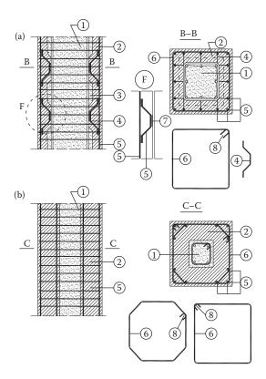
Figure 15.23 Connection of the old to the new reinforcement of the jacket: (a) protection of new bar against buckling with welding; (b) protection of new bars against welding with octagonal ties. I = existing column; 2 = jacket; 3 = key; 4 = bent bars; 5 = added reinforcement; 6 = ties; 7 = welding; 8 = alternating corners.
