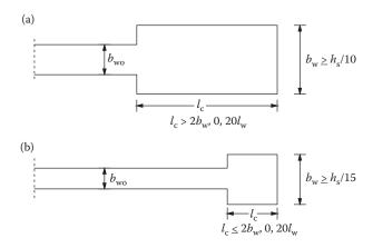
Figure 9.4 (a, b) Minimum thickness of confined boundary elements. (Adapted from E.C.8-1/EN1998-1. 2004. Design of Structures for Earthquake Resistance: General Rules, Seismic Actions and Rules for Buildings. CEN, Brussels, Belgium.)
