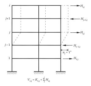
Figure 4.27 Structural interpretation of the elements of matrix K.
