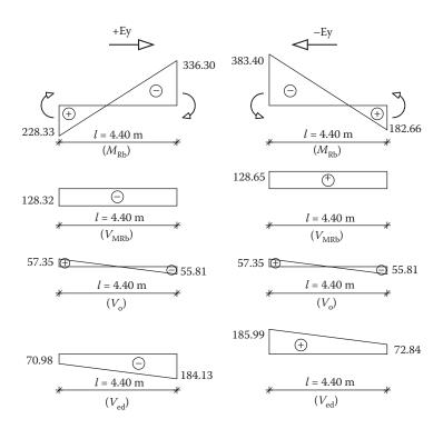
Figure 8.104 Design shear forces of beam 19.
