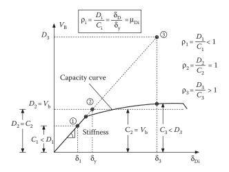
Figure 14.16 Concept for the lateral force elastic analysis.
