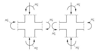
Figure 6.4 Strong columns-weak beams.
