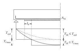
Figure 15.47 Graphic representation of the plate-end extension to avoid plate-end debonding.
