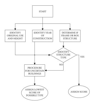
Figure 13.3 Flow chart for the RVSP identification procedure. (From FEMA-154/1988. Rapid Visual Screening of Buildings for Potential Seismic Hazards: A Handbook. Federal Emergency Management Agency, Washington, DC. With permission.)
