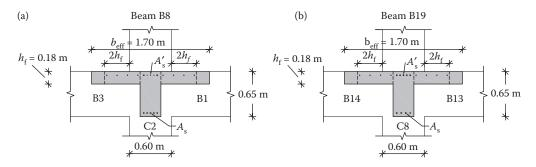
Figure 8.98 Slab effective width of the (a) external (beam 8) and (b) the internal support (beam 19).
