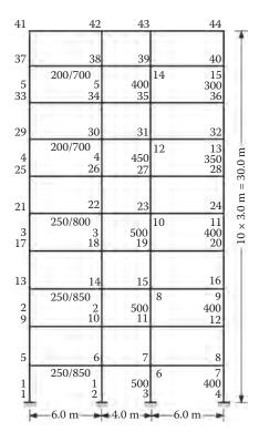
Figure 5.12 Ten-storey R/C frame designed to EC8. (From Penelis, G.G. and Kappos, A.J. 1997. Earthquake-Resistant Concrete Structures. SPON E&FN (Chapman & Hall), London.)
