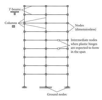
Figure 2.48 Discretisation of a reinforced concrete frame system.
