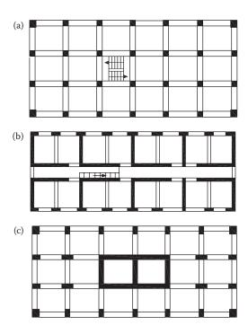
Figure 4.1 Structural systems characterised by simplicity: (a) a typical form of a frame system; (b) a typical configuration of an R/C shear wall system; (c) a dual system with an R/C core and frames.
