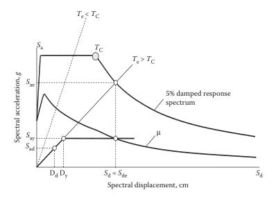
Figure 16.14 Capacity spectrum procedure for bilinear capacity model. (Adapted from RISK-UE W.P. 04, 2003.)
