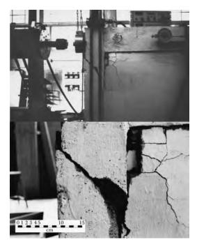
Figure 8.84 Failure mode of the strengthened infilled frame FINR. (Adapted from Stylianidis, K. 2012. Journal of O.C.B.T. 6, 194-212.)
