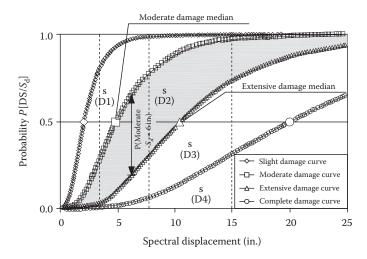
Figure 16.8 Examples of fragility curves – calculation of damage state probability. (From FEMA/HAZUS-MH/MRI. 2002. Multi-Hazard Loss Estimation Methodology: Earthquake Model, Federal Emergency Management Agency (FEMA), Washington, DC. With permission.)
