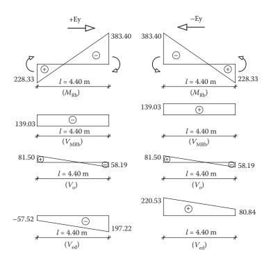
Figure 8.103 Design shear forces of beam 8.
