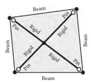
Figure 5.22 Rigid diaphragm modelling (plan view).
