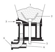
Figure 15.3 The principle of functioning of a shotcreting machine: I = wet material supply; 2 = mixer; 3 = compressed air; 4 = material exit under compression; 5 = rotor; 6 = compressed air.
