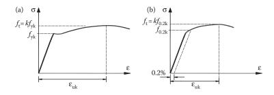
Figure 7.10 Stress-strain diagrams of typical reinforcing steel: (a) hot-rolled steel; (b) cold-rolled steel. (Adapted from EC2-I-I/EN1992-I-I. 2004. Design of Concrete Structures—Part I-I: General Rules and Rules for Buildings. BSI, CEN, Brussels, Belgium.)
