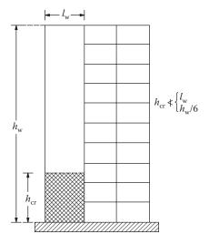
Figure 9.14 Determination of the wall critical region.
