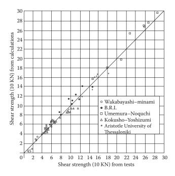
Figure 8.70 Correlation of shear strength results based on tests and on various analytical considerations. (Adapted from Tegos, I. 1984. Contribution to the study and improvement of earthquake-resistant mechanical properties of low slenderness structural elements. PhD thesis, Aristotle University of Thessaloniki (in Greek).)
