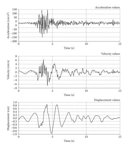
Figure 2.3 Accelerogram of the Athens earthquake of 7 September 1999 (N-S): components and derived diagrams of velocity and displacement. (Adapted from IESEE (Institute of Engineering Seismology and Earthquake Engineering, Greece) 2003. Strong Motion Data Base of Greece 1978–2003, Thessaloniki, Greece.)
