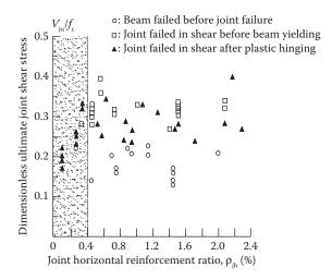
Figure 8.76 Effect of horizontal reinforcement ratio in interior joint ρ<sub>jh</sub> on joint strength. (Adapted from Kitayama, K., Otani, S. and Aoyama, H. 1991. Development of Design Criteria for R/C Interior Beam-Column Joints. ACI Special Publication SP123, American Concrete Institute, Detroit, Michigan, 97–124.)
