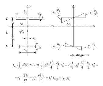
Figure 9.47 Determination of the principal warping moment of inertia Jw of an I section with unequal flanges.
