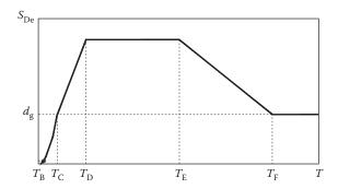
Figure 3.20 Elastic displacement response spectra. (From E.C.8-1/EN1998-1. 2004. Design of Structures for Earthquake Resistance: General Rules, Seismic Actions and Rules for Buildings. CEN, Brussels, Belgium. With permission of the British Standards Institution (BSI, CEN).)
