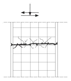
Figure 11.12 Shear wall damage at a construction joint.
