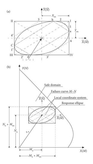
Figure 5.39 Response ellipse and failure envelope: (a) various simplified approaches to the problem; (b) response ellipse in the safe domain of the envelope (bending design).
