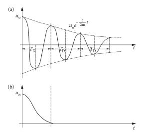
Figure 2.5 Free vibration with damping: (a) initial relative displacement u<sub>o</sub>; (b) initial displacement in case of critical damping. (From Biggs, J.M. 1964. Introduction to Structural Dynamics. McGraw-Hill, New York. With permission.)
