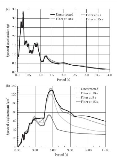
Figure 2.14 The 1978 Tabas (Iran) record filtered at 5, 10 and 15 s cutoff as well as baseline correction only:
