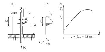
Figure 7.28 Pull-out test: (a) experimental layout; (b) normalised bond stress  $\tau_b$ ; (c)  $\tau_b - s$  diagram. (RILEM/CEB/FIB. With kind permission from Springer Science+Business Media: Leonhardt, F. and Mönnig, E. 1973. Vorlesungen über Massivbau, 1. Teil.)
