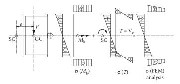
Figure 9.48 Normal stress state of a C section due to pure bending and warping torsion.
