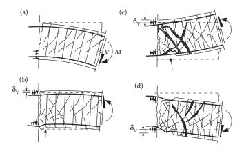
Figure 8.30 Characteristic phases of the response of an R/C beam to reverse cyclic loading: (a) loading downwards; (b) loading upwards up to original position; (c) continuation of the upward loading; (d) reverse loading downwards accompanied with sliding shear.
