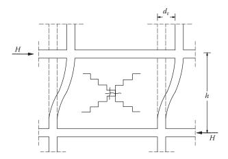
Figure 6.13 Masonry failure with x-shaped cracks due to the R/C frame inter-storey drift d.
