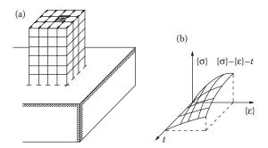
Figure 10.1 Soil–structure interaction analysis inelastic procedures: (a) structural model; (b)  $\{\sigma\}-\{\epsilon\}-t$  relation.
