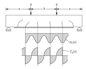
Figure 15.49 Load transfer from the beam to the bonded laminate.
