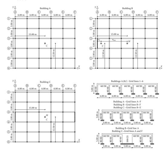
Figure 2.56 Plan view and typical frame arrangements of the buildings.
