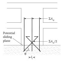
Figure 9.24 Bidiagonal reinforcement in structural walls.
