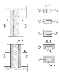
Figure 15.20 R/C column jacketing arrangement: I = existing column; 2 = jacketing concrete.
