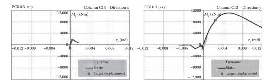
Figure 5.74 Local M-r comparison between static and dynamic analysis for the EC8#2 x+ 0.3  $\cdot$  y excitation.
