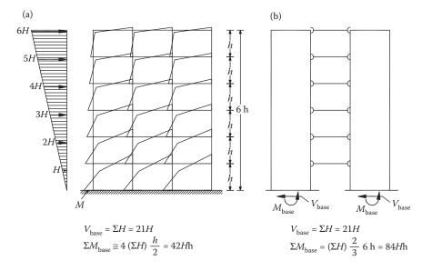
Figure 4.36 Comparison of the response of a frame to the response of a wall system under the same lateral loads: (a) Frame response; (b) wall system response.
