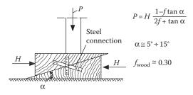
Figure 12.14 Wedging with twin wooden wedges (f is the friction coefficient).
