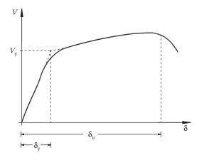
Figure 2.25 Definition of the ductility supply factor.
