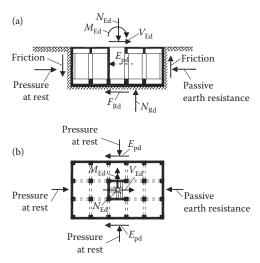
Figure 10.5 Mechanisms for transferring design action effects  $V_{Ed}$ ,  $M_{Ed}$ ,  $N_{Ed}$  to the ground: (a) elevation; (b) plan view.
