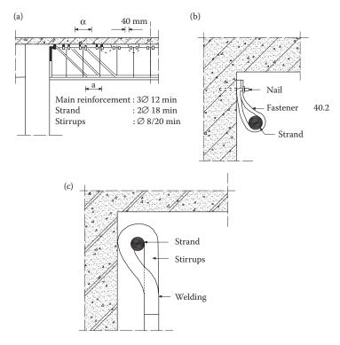
Figure 15.26 Jacket on three sides of a beam: (a) general reinforcement pattern; (b) detail of fixing of the strand; (c) detail of anchoring the ties on the strand.
