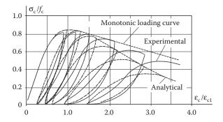
Figure 7.3 Stress-strain diagrams for concrete subjected to repeated uniaxial compression. (Adapted from Karsan, I.D. and Jirsa, J.O. 1969. Journal of the Structural Division, ASCE 95(ST 12), 2543-2563.)
