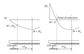
Figure 15.48 Graphic representation of the guidelines for allowable termination points of a three-ply FRP laminate. (a) Simply supported beam; (b) continuous beam. (From ACI 440-2R-02. With permission.)
