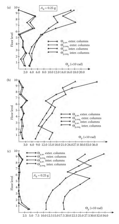
Figure 5.13 Required (demand) available (supply) rotational capacities in 10-storey R/C frame designed for different ductility levels: (a) DCL; (b) DCM; (c) DCH. (From Penelis, G.G. and Kappos, A.J. 1997. Earthquake-Resistant Concrete Structures. SPON E&FN (Chapman & Hall), London.)
