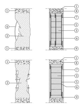
Figure 15.19 Repair of a seriously damaged column: I = existing undamaged concrete; 2 = existing damaged concrete; 3 = new concrete; 4 = buckled reinforcement; 5 = added new reinforcement; 6 = added new ties; 7 = welding; 8 = existing ties; 9 = existing reinforcement.
