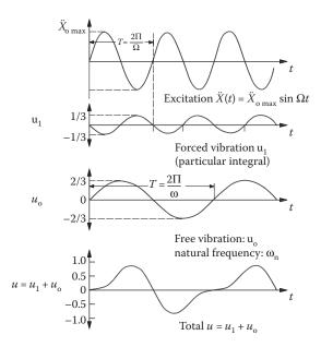
Figure 2.6 Forced vibration of an SDOF system excited by a sinusoidal base acceleration for  $\Omega/\omega = 2$ .
