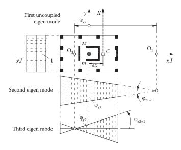
Figure 2.46 Eigen modes of vibration of a single-storey pseudospatial structure, symmetric about the x-x axis.
