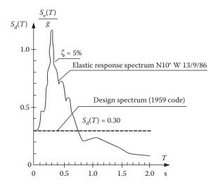
Figure 11.38 The Kalamata, Greece, earthquake of 13 September 1986: comparison of the elastic response spectrum with the design spectrum.
