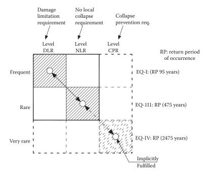
Figure 3.24 Matrix coupling of three performance levels with three levels of seismic excitation for new buildings according to EC8-I/2004.
