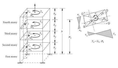
Figure 4.28 Determination of the 'plasmatic' axial of centre of stiffness C.
