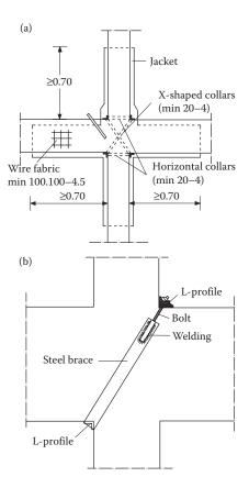
Figure 15.30 Strengthening of a joint with prestressed collars: (a) general arrangement of the strengthening; (b) detail of the prestressed collar.
