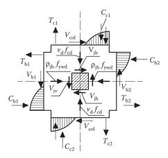
Figure 8.78 The homogeneous stress field in the joint. (Adapted from E.C.8-I/EN1998-1. 2004. Design of Structures for Earthquake Resistance: General Rules, Seismic Actions and Rules for Buildings. CEN, Brussels, Belgium.)
