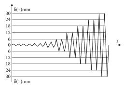
Figure 7.6 Loading program (two cycles per step) for testing of infilled R/C frames. (Adapted from Stylianidis, K. 2012. The Open Construction and Building Technology Journal, 6, 194–212.)
