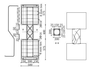
Figure 8.61 Rhombic reinforcement and ties of short columns against shear.
