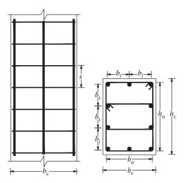
Figure 7.23 Confinement of concrete orthogonal cross-section with hoops.
