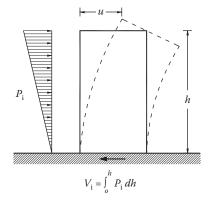
Figure 3.1 Lateral load  $P_i$  of a building developing base shear  $V_i$  and respective top horizontal displacement u.
