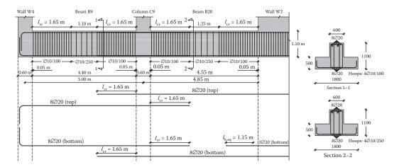
Figure 10.23 Flexural and shear reinforcement of foundation beams 9 and 20.
