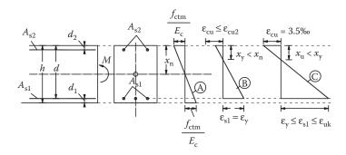
Figure 8.13 Deformation pattern of a cross section: (A) cracking; (B) yield; (C) failure.
