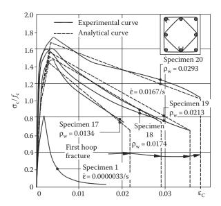
Figure 7.18 Stress-strain diagrams for concrete confined by different numbers of hoops. (Adapted from Scott, B.D., Park, R. and Priestley, M.J.N. 1982. ACI Structural Journal, Vol. 79(1), 13-27.)
