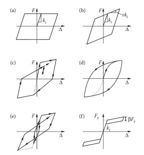
Figure 2.21 Hysteresis rules considered in inelastic time-history analysis. (a) Elastolastic (EPP); (b) bilinear, r = 0.2 (BI); (c) modified clough model; (d) Ramberg-Osgood model; (e) trilinear stiffness-degrading; (f) flag shaped (FS).
