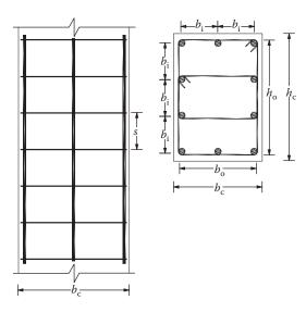
Figure 8.49 Confinement of concrete core.
