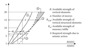
Figure 11.47 Explanation of the seismic vulnerability of high-rise buildings: (I) shear-strength curve of vertical structural elements; (2) additional strength due to masonry, constant for all floors; (3) required shear strength (seismic action), almost proportional to R<sub>STR</sub>; (4) shaded area—buildings with damage.
