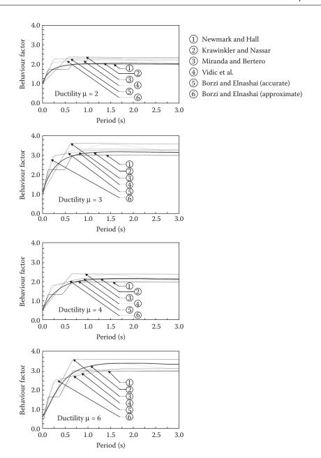
Figure 2.27 Comparison of (demand) derived by using different expressions for elastic—perfectly plastic systems on rock site; values of ductility μ: 2, 3, 4 and 6. (From Elnashai, A.S. and Di Sarno, L. Fundamentals of Earthquake Engineering, 2008. Copyright Wiley-VCH Verlag GmbH & Co. KGaA. Reproduced with permission.)
