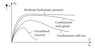
Figure 7.17 Stress-strain diagrams for various types of confinement.
