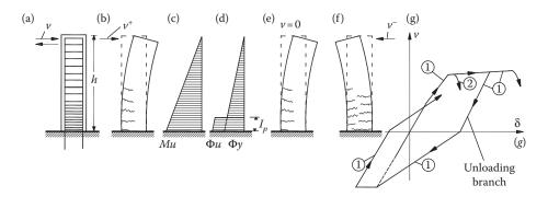
Figure 2.29 Inelastic response of a cantilever R/C beam under cyclic loading: (a) arrangement of cantilever loading; (b) loading with  $V^+$  beyond yielding; (c) ultimate failure moment diagram; (d) distribution of curvature  $\phi$ -plastic hinge zone  $I_p$ ; (e) unloading V=0; (f) loading with  $V^-$  beyond yielding; (g)  $V-\delta$  diagram for normally reinforced (1) and over-reinforced (2) cantilever.
