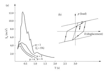
Figure 2.31 (a) Inelastic spectra of the Kalamata (1986), Greece, earthquake components N10°W, for various ductility factors μ; (b) Clough-Riddel-Newmark hysteresis model.
