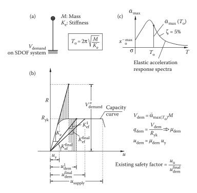
Figure 3.4 Displacement-based design based on inelastic static analysis (a push-over analysis). (a) Structural system; (b) capacity design curve and successive steps for the determination of u demand; (c) elastic acceleration response spectrum.
