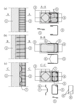
Figure 15.22 One-sided strengthening of a column: (a) use of hooks for reinforcement connection; (b) use of welding of ties for reinforcement connection; (c) use of welded bent bars for reinforcement connection. I-existing column; 2 = jacket; 3 = existing reinforcement; 4 = added longitudinal reinforcement; 5 = added ties; 6 = welding; 7 = bent bars; 8 = metal plate.
