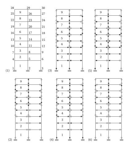
Figure 2.55 Frame system GRFR8: (1) numbering of nodes and floors. Formation of plastic hinges during an excitation from the following earthquakes: (2) El Centro x I; (3) Pacoima x I; (4) El Centro x 1.5 (5) Thessaloniki x 2.6; (6) El Centro x 0.75.
