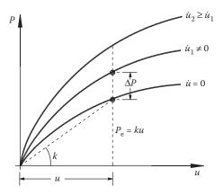
Figure 2.17 Qualitative diagrams of the axial force P versus normal strain u for various loading rates.
