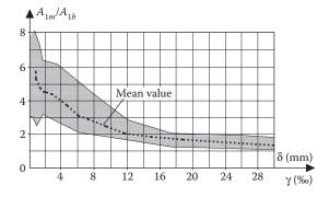
Figure 8.92 Program #2. Mean value and scatter of the ratio of infilled frames to bare frames energy dissipation A<sub>1 m</sub>/A<sub>1b</sub>. (Adapted from Stylianidis, K. 2012. *Journal of O.C.B.T.*, 6, 194–212.)
