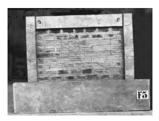
Figure 8.86 Failure mode of the infilled frame F5. (Adapted from Stylianidis, K. 2012. Journal of O.C.B.T., 6, 194-212.)
