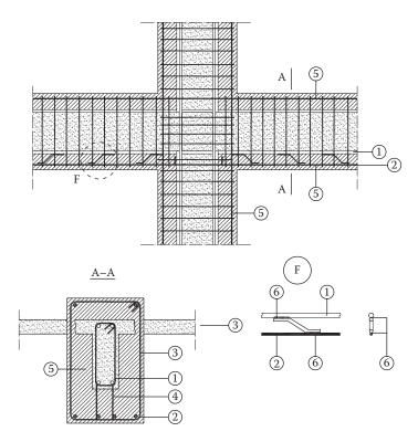
Figure 15.25 Jacket on four sides of a beam: I = existing reinforcement; 2 = added longitudinal reinforcement; 3 = added stirrups; 4 = welded connecting bar; 5 = concrete jacket; 6 = welding.
