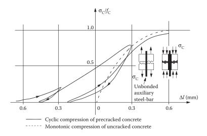
Figure 15.12 Monotonic and cyclic compression of cracked concrete.
