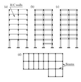
Figure 13.12 Examples of 'acceptable' structural layout.
