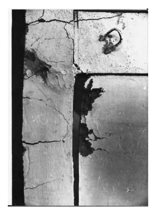
Figure 8.94 Separation of the infill from the frame; local crushing of the infill corners of frame F4R. (Adapted from Stylianidis, K. 2012. Journal of O.C.B.T., 6, 194–212.)
