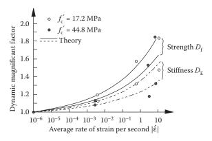
Figure 7.4 Dynamic magnification factors D<sub>f</sub> and D<sub>E</sub> to allow for strain rate effects on strength and stiffness. (From Priestley, M.J.N. and Wood, J.H. 1977. Behaviour of a complex prototype box girder bridge. Proceedings of the RILEM International Symposium on Testing In-Situ of Concrete Structures, Budapest, I, 140–153. Copyright Wiley-VCH Verlag GmbH & Co. KGaA. Reproduced with permission.)
