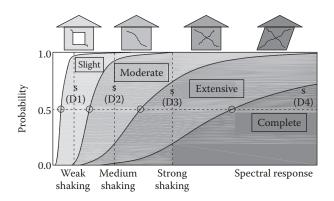
Figure 16.7 Examples of fragility curves for slight, moderate, extensive and complete damage. (From FEMA/HAZUS-MH/MRI. 2002. Multi-Hazard Loss Estimation Methodology: Earthquake Model, Federal Emergency Management Agency (FEMA), Washington, DC. With permission.)
