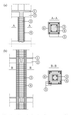
Figure 15.21 Column jackets: (a) jacket along the height of one storey; (b) jacket extended to the upper and lower storey; I = slab, 2 = beam, 3 = existing column, 4 = jacket, 5 = added longitudinal reinforcement, 6 = added ties.
