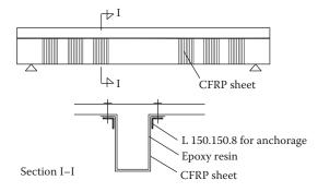
Figure 15.10 Strengthening of a T beam against shear by applying CFRP sheets.
