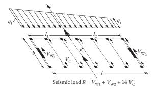
Figure 9.51 Determination of diaphragm loading due to seismic action.
