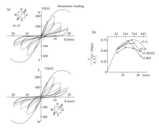
Figure 8.53 Diagonal cyclic loading of columns: (a) hysteresis loops in each direction; (b) envelope of the resultant action. (Adapted from Jirsa, J.O., Maruyama, K. and Ramirez, H. 1980. The influence of load history on the shear behaviour of short RG columns. Proceedings of the 7th World Conference on Earthquake Engineering, Istanbul, 6, 339–146.)
