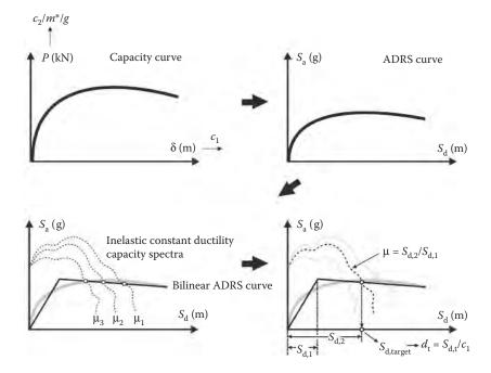
Figure 5.70 Derivation of target displacement from the capacity curve using the ADRS method.
