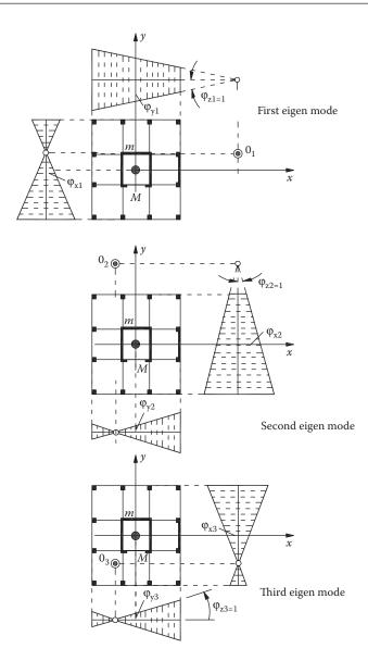
Figure 2.45 The three eigen modes of vibration of a single-storey pseudospatial structure.
