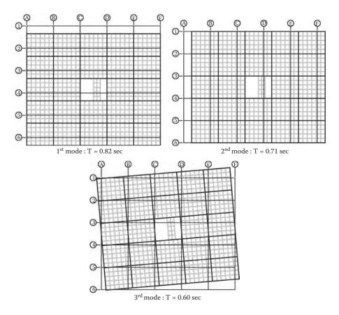
Figure 5.49 Fundamental modes of vibration.
