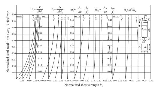
Figure 8.67 Diagrams for the calculation of the shear strength for squat columns ( $\lambda < 4$ ) and  $\omega_s > \alpha^2 \omega_w$ . (Adapted from Tegos, I. 1984. Contribution to the study and improvement of earthquake-resistant mechanical properties of low slenderness structural elements. PhD thesis, Aristotle University of Thessaloniki (in Greek).)
