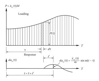
Figure 2.8 Response  $u_0(t)$  of an SDOF system to a differential impulse.
