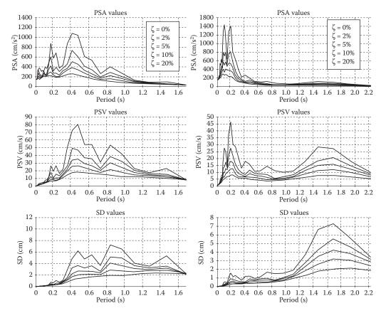
Figure 2.10 Elastic response spectra for 1999 Parnitha (Athens, Greece; right) and for 1978 Thessaloniki (Volvi, Greece; left) earthquakes for various damping values: acceleration (top) velocity (middle) and displacement (bottom). (Adapted from I.E.S.E.E. (Institute of Engineering Seismology and Earthquake Engineering, Greece) 2003. Strong Motion Data Base of Greece 1978–2003, Thessaloniki, Greece.)
