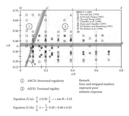
Figure 5.2 Evaluation of the structural regularity and torsional rigidity criteria in a one-storey structure. (Adapted from Cosenza, E., Munfredi, G. and Realfonzo, R. 2000. Torsional effects and regularity conditions in R/C buildings. Proceedings of the 12th World Conference on Earthquake Engineering, Auckland.)
