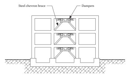
Figure 3.8 Passive energy dissipators (dampers) in a building.
