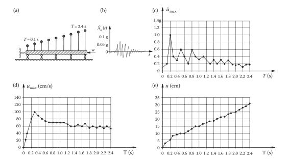
Figure 2.9 Response spectra of SDOF systems: (a) shaking table carrying SDOF systems with t = 0.1-2.4 s; (b) accelerogram; (c) acceleration spectrum; (d) velocity spectrum; (e) displacement spectrum.
