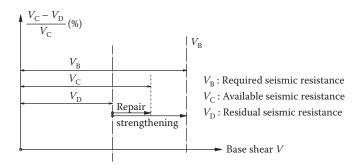
Figure 13.9 Schematic presentation of  $V_B$ ,  $V_C$ ,  $V_D$ .
