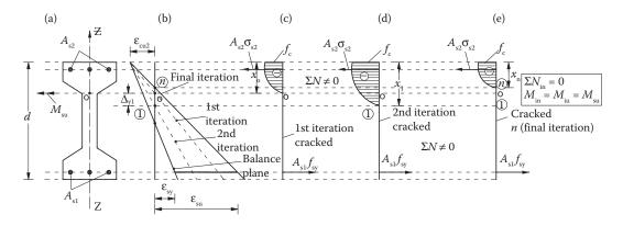
Figure 8.18 Cross section at concrete failure under compression: (a) cross section; (b) deformation pattern at successive iteration cycles 0.1, n; (c) internal forces of iteration (1); (d) internal forces of iteration (2); (e) internal forces of final iteration (n).
