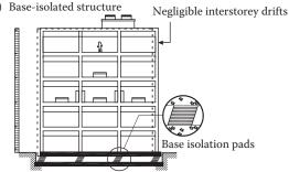
Figure 3.7 Comparative response to seismic action (a) of a conventional earthquake-resistant building; (b) of a building with seismic isolation.
