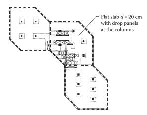
Figure 4.33 One Magnificent Mile; tube system with flat slabs and a hexagonal multicell floor plan. (From König, G. and Liphardt, S. 1990. Hochhäuser aus Stahlbeton, Beton Kalender, Teil II, 457–539. Copyright Wiley-VCH Verlag GmbH & Co. KGaA. Reproduced with permission.)
