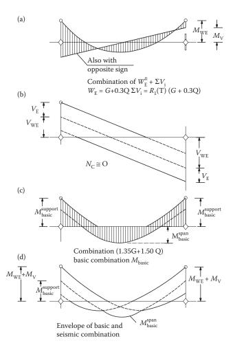
Figure 8.3 Moment diagram of frame beams for various load cases: (a) seismic combination with the corresponding gravity loads; (b) shear diagrams corresponding to load case combination (a); (c) basic load combination (1.35G+1.50Q); (d) Bending moment envelope of basic load combination (c) with seismic load combination (a).
