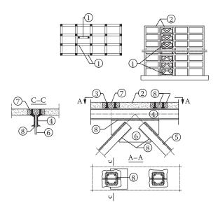
Figure 15.57 Addition of truss systems inside R/C frames: I = added steel truss; 2 = existing structure; 3 = steel dowel; 4 = horizontal steel rod; 5 = diagonal steel rod; 6 = steel joint plate; 7 = added concrete; 8 = welding.
