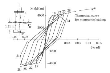
Figure 9.7 Moment-rotation hysteresis loops for slender R/C wall with barbell cross-section subjected to cyclic loading. (Oesterle et al., 1980)
