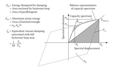
Figure 14.5 Derivation of damping for spectral reduction. (From ATC 40. 1996. Seismic Evaluation and Retrofit of Concrete Buildings. Applied Technology Council, Redwood City, California. With permission.)
