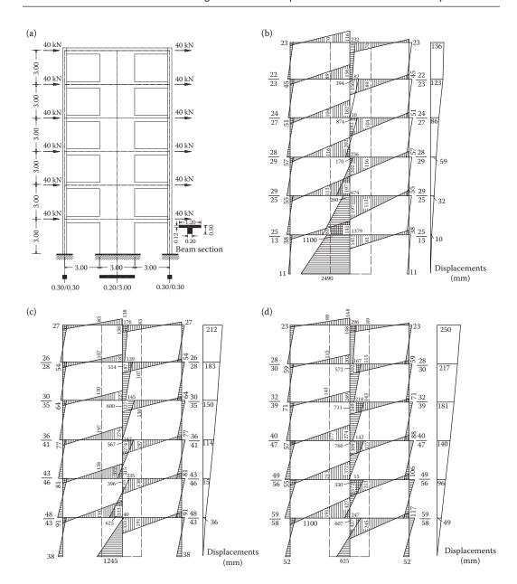
Figure 4.25 Moment diagrams of a dual system under lateral loading for various degrees of wall base restraint. (a) Dual frame—wall structure, (b) wall fully fixed on the ground, (c) wall flexibly supported on the ground (50% fixity) and (d) wall flexibly supported on the ground (25% fixity).
