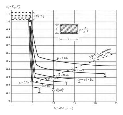
Figure 5.24 Ratio of cracked over uncracked rigidity as a function of reinforcement percentage.
