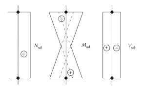
Figure 8.5 M, N, V column diagrams under horizontal seismic and corresponding gravity loads.
