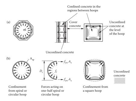
Figure 7.19 Confinement of concrete by circular and square hoops: (a) region confined by hoops; (b) stress pattern due to confinement by hoops. (Adapted from Penelis, G.G. and Kappos, A.J. 1997. Earthquake-Resistant Concrete Structures. SPON E&FN (Chapman & Hall), London.)
