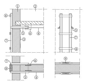
Figure 12.13 Bracing with internal tension ties: I = exterior wall; 2 = interior wall; 3 = crack; 4 = steel tensioner; 5 = angle 50.50.5 mm; 6 = steel plates; 7 = steel profiles; 8 = steel plates; 9 = tensioner coupler.
