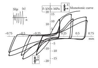
Figure 7.31 Bond stress-slip diagram under cyclic loading with  $f_c = 25$  Mpa. (Adapted from Balázs, G.L. 1989. Bond softening under reversed load cycles. Studie Ricerche, Politecnico di Milano, No. 11, Milano, 503–524.)
