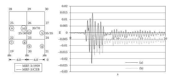
Figure 2.52 Time history of top displacement in a 3-storey frame under the seismic action of 1999 Athens earthquake designed: (a) according to Greek Code of 1959 and (b) according to EC 8-1/2004.
