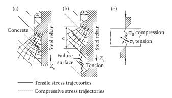
Figure 7.26 Qualitative stress and failure surface distribution of concrete at the ribs of deformed bars: (a) for large rib spacing; (b) for small rib spacing; (c) failure surface at shear (according to E. Morsh). (With kind permission from Springer Science+Business Media: Leonhardt, F. and Mönnig, E. 1973. Vorlesungen uber Massivbau, Erster Teil.)
