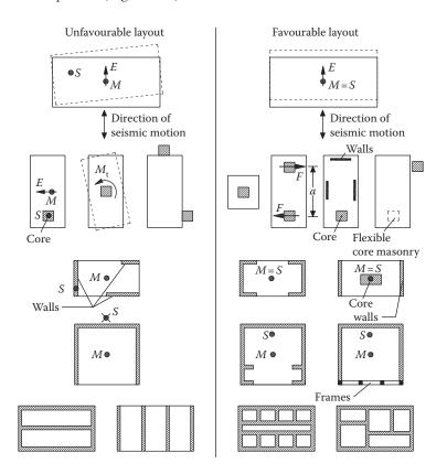
Figure 4.3 Distribution of mass and stiffness in plan.
