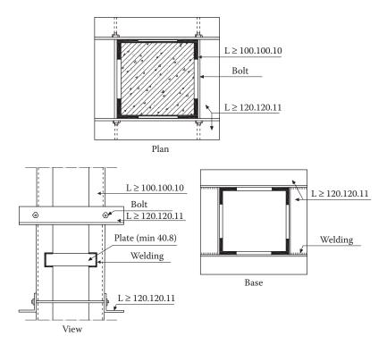
Figure 12.9 Immediate tying of a column with steel profiles.
