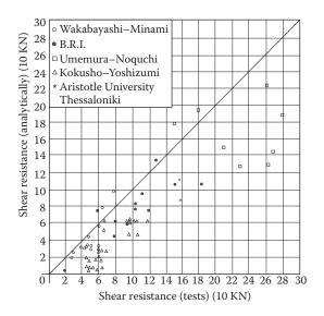
Figure 8.64 Correlation of test results and analytical considerations according the Sohara and Kato method. (Adapted from Tegos, I. 1984. Contribution to the study and improvement of earthquake-resistant mechanical properties of low slenderness structural elements. PhD thesis, Aristotle University of Thessaloniki (in Greek).)
