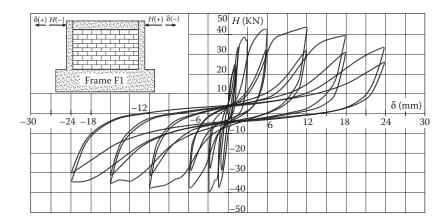
Figure 8.88 Lateral load-displacement loops. Infilled frame FI. (Adapted from Stylianidis, K. 2012. *Journal of O.C.B.T.*, 6, 194–212.)
