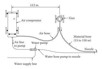
Figure 15.2 Typical arrangement of equipment for shotcreting.
