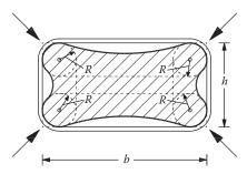
Figure 15.52 Confinement effectiveness factor for orthogonal cross-section depending on rounded corner radius R.
