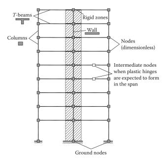
Figure 2.47 Discretisation of a reinforced concrete plane structure.
