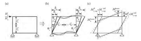
Figure 5.11 Moment-curvature displacement diagrams of R/C frames with strong columns-weak I<sub>v</sub> beams:
