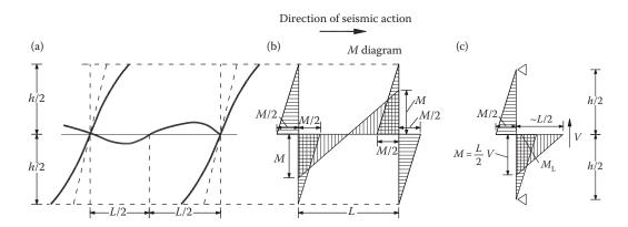
Figure 8.8 Flexural behaviour of a frame sub-assemblage: (a) deformations; (b) moment diagrams; (c) substitute sub-assemblage.
