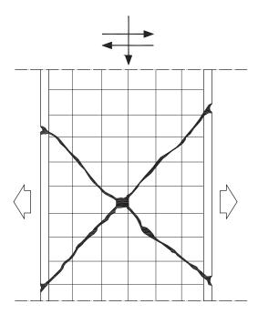
Figure 11.14 Shear wall damage due to shear (X-shaped cracks).
