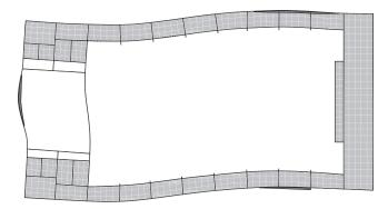
Figure 4.14 Palace—Aliki theaters, Athens, Greece 3rd eigen mode of the structure at the level of balconies (FEM elastic modal spectrum analysis).
