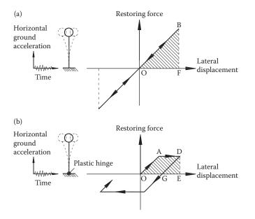
Figure 2.23 Response of SDOF systems to seismic action: (a) elastic response; (b) elastoplastic response.
