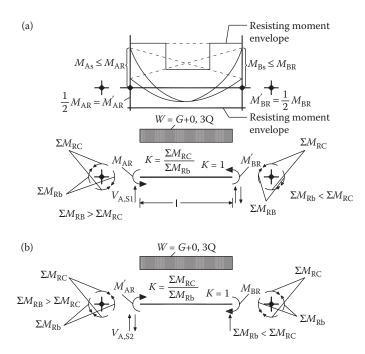
Figure 6.2 Capacity design values of shear forces acting on beams; (a) resisting moment envelope; (b) equilibrium conditions for the determination of shear forces.
