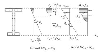
Figure 9.22 Determination of the confinement of a composite cross-section following an iterative step-bystep method.
