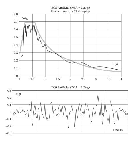
Figure 3.21 Artificial accelerogram for PGA = 0.24 g. (After Sextos, A., Pitilakis, K. and Kappos, A. 2003. Earthquake Engineering and Structural Dynamics, V, 32(4), 607–627.)
