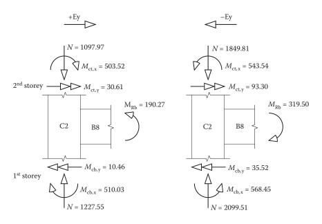
Figure 8.99 Capacity design moments for column C2.
