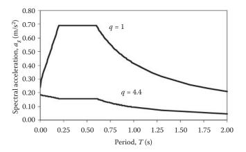
Figure 5.45 Elastic and design response spectrum of EC8-Part I (2004).
