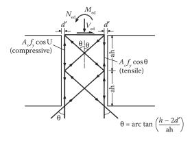
Figure 8.71 The additional mechanism of shear resistance in the case of rhombic reinforcement.
