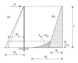
Figure 7.16 Schematic presentation of the reasoning behind the requirement that  $f_t/f_y > 1.0$ : (a) Moment diagrams yield and failure; (b) curvature diagram: plastic rotation  $\theta_{p1} = A_{p1}$ . In conclusion, if there is no degree of strain hardening  $(f_t > f_y)$ , there is no plastic hinge.
