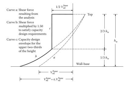
Figure 6.10 Design envelope of the shear forces in the walls of a dual system: Curve a: Shear forces resulting from the analysis. Curve b: Shear forces multiplied by 1.50 to satisfy capacity design requirements. Curve c: Capacity design envelope for the upper 2/3 of the height.
