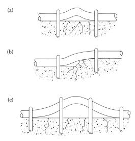
Figure 8.22 Different modes of buckling in reinforcing bars.
