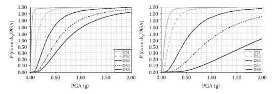
Figure 16.12 Fragility curves (in terms of PGA) for medium-rise dual infilled systems, low (left) and high (right) code design. (With kind permission from Springer Science+Business Media: Kappos, A. et al. 2006b. A hybrid method for the vulnerability assessment of R/C and URM buildings. Bulletin of Earthquake Engineering, 4, 391–413.)
