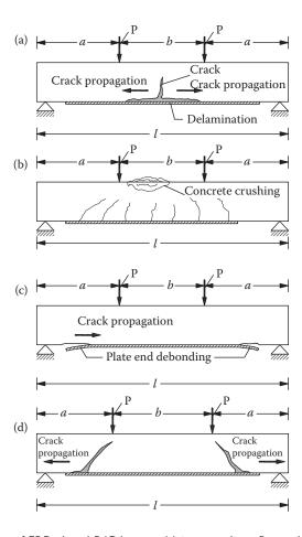
Figure 15.45 Failure modes of FRP-plated R/C beams: (a) intermediate flexural crack-induced delamination; (b) crushing of compressive zone; (c) plate-end debonding; (d) intermediate shear crack-induced debonding.
