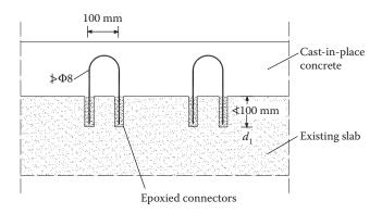
Figure 15.28 Shear connectors between old and new concrete in the compression zone.
