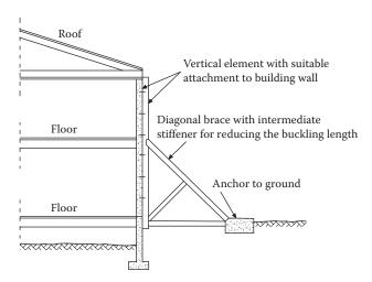
Figure 12.10 Bracing with buttresses.
