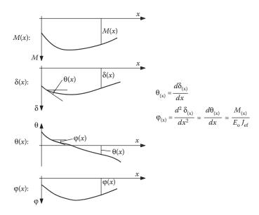
Figure 5.6 Differential relations between bending moment M(x), curvature  $\phi(x)$ , rotation  $\theta(x)$ , and displacement  $\delta(x)$  established first by Mohr.
