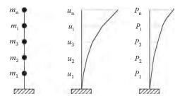
Figure 5.29 Modal deformation of a torsionally insensitive (translational) MDOF system.
