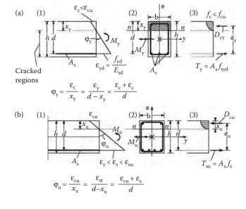
Figure 5.7 (a) Curvature  $\phi_y$  at yield for R/C members under bending: (1) strain pattern at yield plane; (2) cross-section at yield; (3) internal force pattern. (b) Curvature  $\phi_u$  at failure for R/C members under plane bending: (1) strain pattern at failure; (2) cross-section at failure; (3) internal forces at failure.
