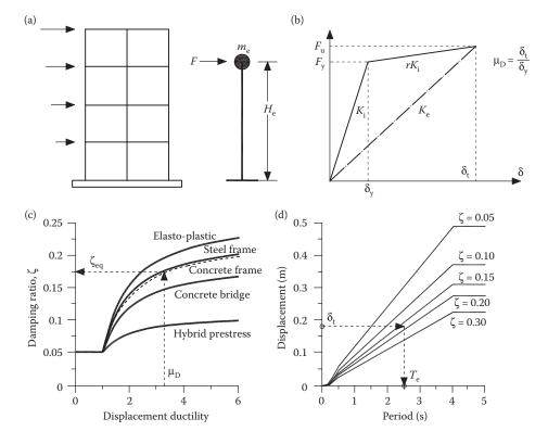
Figure 14.9 Fundamentals of direct displacement-based design. (a) SDOF simulation; (b) Effective stiffness K<sub>C</sub>; (c) Equivalent damping vs. ductility; (d) Design displacement spectra. (From Preistley, M.J., Calvi, G.M. and Kowalsky, M.J. 2007. Displacement-Based Seismic Design of Structures. IUSS Press, Pavia. With permission.)
