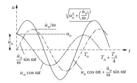
Figure 2.4 Diagram of the free vibration relative displacement of Equation 2.4 for input data: initial displacement  $u = u_o$  and initial velocity  $\dot{u} = \dot{u}_o$ .
