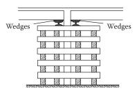
Figure 12.8 Shoring with timber grillage.
