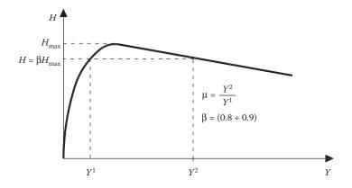
Figure 8.93 Definition of the ductility index. (Adapted from Stylianidis, K. 2012. Journal of O.C.B.T., 6, 194-212.)
