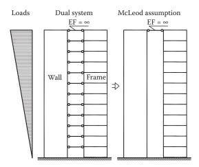
Figure 4.24 Simulation of coupling between frame and shear wall in a dual system with only one coupling bar at the top.
