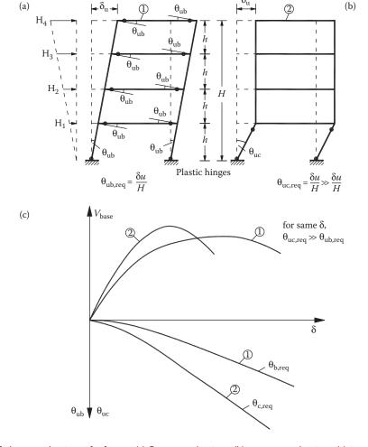
Figure 6.3 Failure mechanism of a frame: (a) Beam mechanism; (b) storey mechanism; (c) interpretation of the vulnerability of a storey mechanism via  $V_{\rm base} - \delta - \theta$  diagram.
