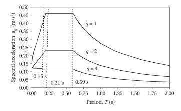
Figure 2.57 Design spectrum of EC8 (2004).
