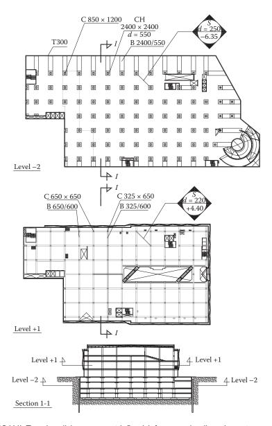
Figure 4.11 VRBANI, Zagreb mall; basements with flat slab frames and walls at the perimeter; frame system at the superstructure with limited shear walls.
