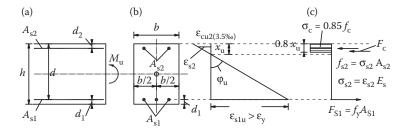
Figure 8.15 Cross section at failure: (a) geometry; (b) deformation pattern; (c) internal forces.
