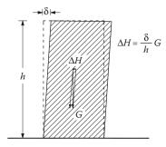
Figure 12.11 Estimate of the horizontal forces due to deviation from the vertical axis.
