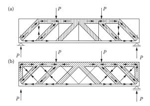
Figure 8.26 Mörsh truss mechanism: (a) stirrups as shear reinforcement; (b) bent-up bars as shear reinforcement.
