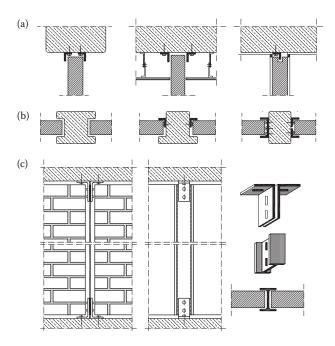
Figure 6.15 Detailing of separation joints between partition walls and R/C frame: (a) upper boundary; (b) lateral boundary; (c) reinforcement for out-of-plane overturning.
