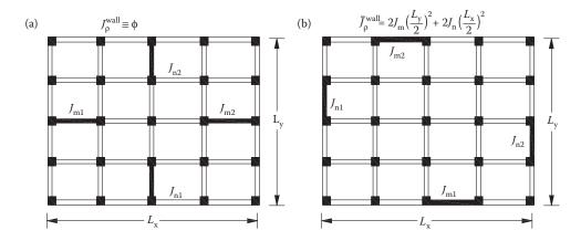
Figure 2.41 Effect of the arrangement of the structural walls on the torsional stiffness of the system: (a) system with low torsional stiffness; (b) system with high torsional stiffness.
