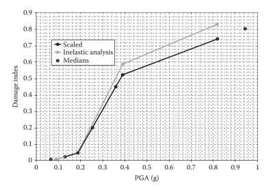
Figure 16.6 PGA – damage index relationship for an R/C building type (moderate height infilled). (With kind permission from Springer Science+Business Media: Kappos, A. et al. 2006b. A hybrid method for the vulnerability assessment of R/C and URM buildings. Bulletin of Earthquake Engineering, 4, 391–413.)
