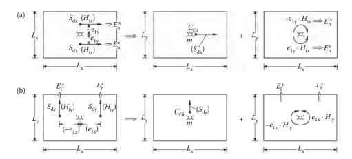
Figure 5.41 Seismic action effects E resulting from a modular response spectrum analysis: (a) seismic action in the x-x direction; (b) seismic action in the y-y direction.
