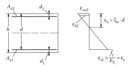
Figure 8.16 Strain pattern for  $\boxtimes_{S2} \ge (f_y/E_S) = \boxtimes_y$ .
