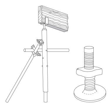
Figure 12.6 Independent industrial-type metal supports.
