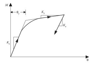
Figure 2.51 Fundamental behaviour of plasticity element (Wilson 2001).
