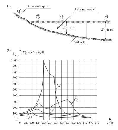
Figure 2.12 Mexico City earthquake 19.9.1985: (a) the ground stratification of Mexico City and (b) acceleration response spectra at points (1), (2), (3) and (4).
