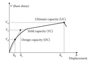
Figure 5.26 Capacity spectrum.
