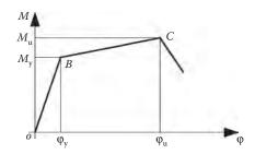
Figure 5.8 Moment-curvature diagram of a ductile R/C member under bending.
