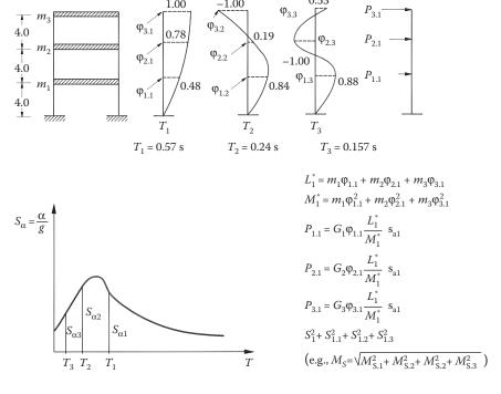
Figure 2.35 A three-storey plane frame analysed according to spectral modal analysis.
