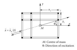
Figure 2.44 Pseudospatial single-storey system excited by an accelerogram  $\ddot{x}_o(t)$  in the direction of angle  $\theta$  with respect to the x-x axis.
