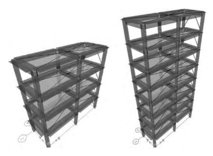
Figure 5.31 Torsionally unrestrained four-storey and eight-storey buildings.
