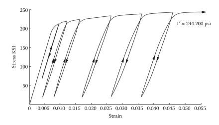
Figure 7.12 Stress-strain curve for steel wire under repeated tensile loading. (Adapted from Sinha, B.P., Gerstle, K.H. and Tulin, L.C. 1964. Journal of the American Concrete Institute, Proceedings, 61(8), 1021-1038; Park, R. 1973. Theorization of structural behaviour with a view to defining resistance and ultimate deformability. Symposium on Resistance and Ultimate Deformability of Structures Acted on by Well-Defined Repeated Loads. IABSE, Lisboa, 1973. With permission of IABSE.)
