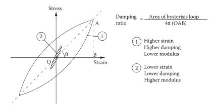
Figure 10.2 The effect of shear strain on damping and shear modulus of soils. (Adapted from Dowrick, D. 2005. Earthquake Risk Reduction, John Wiley and Sons, Ltd, Chichester, West Sussex. England.)
