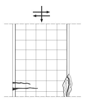
Figure 11.17 Shear wall damage due to flexure and compression.
