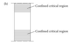
Figure 15.11 Confinement of an orthogonal R/C column by applying CFPR sheets: (a) wrapping with FRP sheets for axial strength enhancement; (b) wrapping with FRP sheets at the plastic joints for increasing ductility capacity of the plastic joints.
