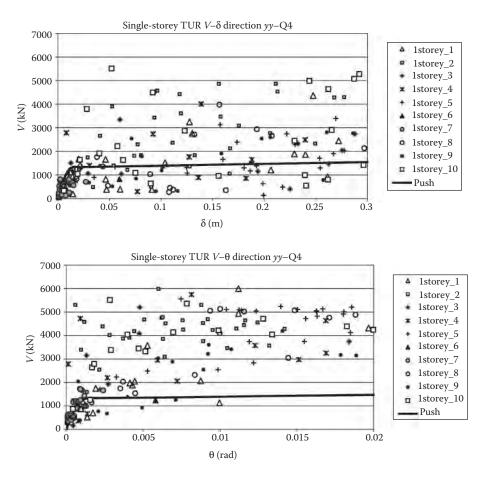
Figure 5.33 Torsionally unrestrained single-storey building  $V-\delta$  and  $V-\theta$ .
