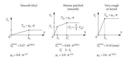
Figure 15.13 Formalistic models for concrete-to-concrete friction as a function of normal compressive stress σ.
