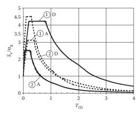
Figure 3.19 Soft soils (D) amplify the maxima of spectral diagrams more strongly than firm ones (A).
