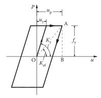
Figure 2.20 Relation between hysteretic damping  $\zeta_{\text{hyst}}$  and ductility  $\mu.$
