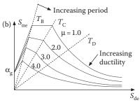
Figure 14.3 Demand spectra for various ductility μ values: (a) traditional acceleration response spectrum in relation to period T; (b) acceleration-displacement response spectra (ADRS) for various ductility  $\mu$  values.
