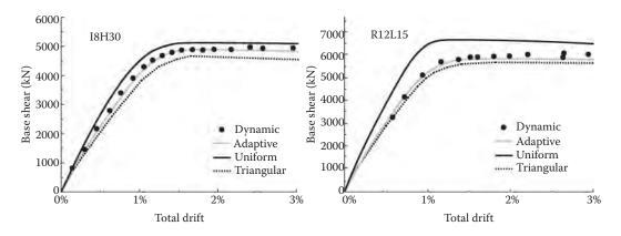
Figure 5.28 Adaptive pushover, pushover and nonlinear T-h: (a) asymmetric system of high ductility; (b) symmetric system of low ductility.
