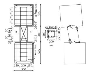
Figure 8.60 Bidiagonal reinforcement and ties of short columns against shear.
