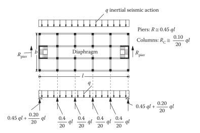
Figure 9.50 The structural behaviour of a long diaphragm with two cores at its ends.
