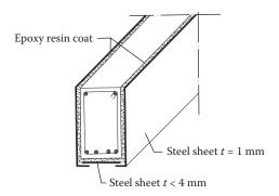
Figure 15.6 Strengthening of a beam with resin bonded metal sheets.
