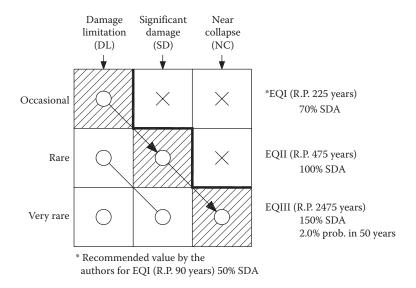
Figure 14.10 Relationship between performance level and earthquake design level (according to EC8-3/2005).
