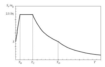
Figure 3.16 Generic shape of the elastic response spectrum. (From E.C.8-1/EN1998-1. 2004. Design of Structures for Earthquake Resistance: General Rules, Seismic Actions and Rules for Buildings. CEN, Brussels, Belgium. With permission of the British Standards Institution (BSI, CEN).)
