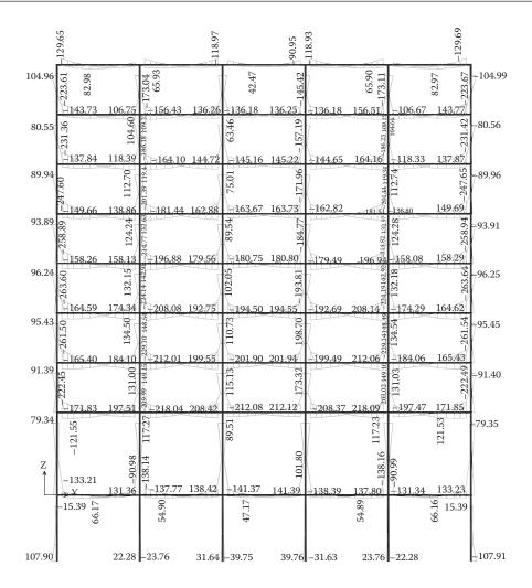
Figure 5.53 Envelope of bending moments - Grid axis B.
