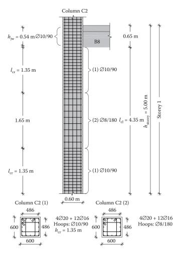
Figure 8.100 Flexural and shear reinforcement of column C2.
