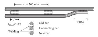
Figure 15.7 Welding of a new reinforcement bar.
