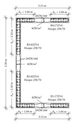
Figure 9.54 Flexural and shear reinforcement of wall W2.
