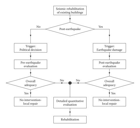
Figure 13.1 Flow chart for pre- and post-earthquake evaluation and rehabilitation.
