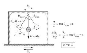
Figure 2.1 Seismic loads of old seismic codes.
