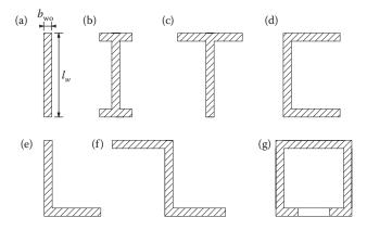
Figure 9.3 Various cross-sections of ductile slender walls: (a) orthogonal; (b) barbell; (c) T-shaped; (d) C-shaped; (e) L-shaped; (f) Z-shaped; (g) tubular.
