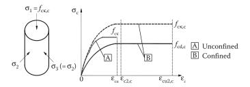
Figure 7.20 Stress-strain diagrams of confined concrete. (Adapted from EC2-1-I/EN1992-1-1. 2004. Design of Concrete Structures—Part 1-1: General Rules and Rules for Buildings. BSI, CEN, Brussels, Belgium.)
