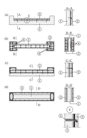
Figure 15.34 Strengthening of a wall with a jacket: (a) one sided jacket; (b) thickenings at the ends of the existing wall; (c) one sided jacket with end-thickenings; (d) jackets, on both sides of the existing wall. I = existing wall; 2 = added wall; 3 = added columns; 4 = welding; 5 = epoxied bar.
