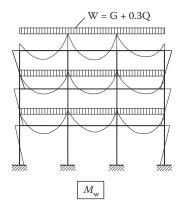
Figure 8.1 Bending moment diagram for gravity loads.
