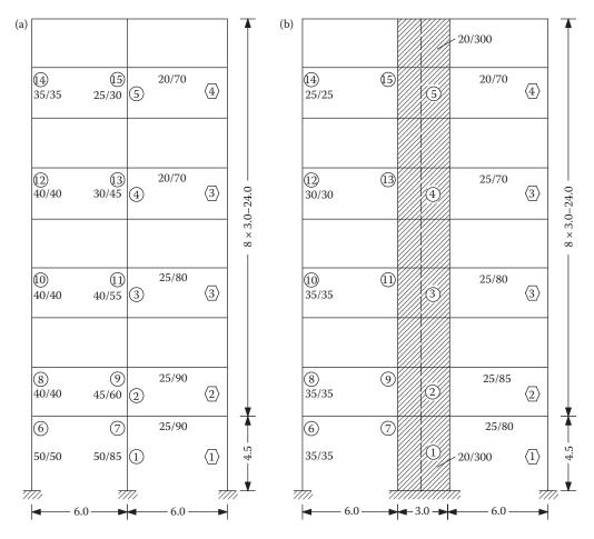
Figure 2.50 Geometric characteristics of two systems for which inelastic analysis was performed: (a) GRFR8 and (b) GRFW8. (Adapted from Kappos, A.J. 1991. Earthquake Engineering and Structural Dynamics, 20(2), 167–176.)
