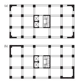
Figure 4.6 Layout of shear walls at the perimeter (a) acceptable arrangement, (b) improved arrangement.
