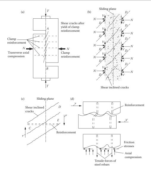
Figure 9.25 Shear transfer model at a sliding joint: (a) experimental set-up; (b) transfer model along an uncracked joint; (c) detail of (b); (d) shear sliding. Friction stresses along a pre-cracked sliding plane.
