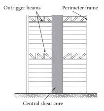
Figure 4.37 Outriggers in a shear core combined with perimeter frame (tube). (Adapted from Booth, E. and Key, D. 2006. Earthquake Design Practice for Buildings, Thomas Telford Ltd.)
