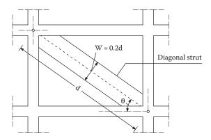
Figure 8.95 Compression diagonal model for the estimation of infill stiffness.
