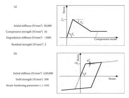
Figure 5.59 Material models (concrete, steel) used for fibre analysis: (a) concrete; (b) steel reinforcement.
