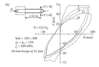
Figure 8.46 Hysteresis loops of elements under flexure and axial loading at various levels: (a) axial load N = 0; (b) axial load N = 0.5 N<sub>b</sub>. (Adapted from Jirsa, J.O. 1974. Factors influencing behaviour of reinforced concrete members under cyclic overloads. Proceed of 5th World Conf. on Earthq. Eng. June 1973, Rome, Italy, 2 pp. 1198–1204.)
