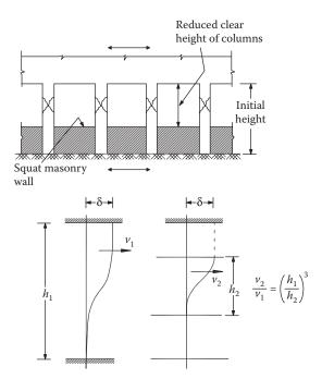
Figure 4.8 Concentration of large shear forces on short columns at the perimeter of the building.
