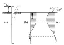
Figure 10.14 Long pile response to  $V_{\rm Ed}$  loading in cohesive soil (a) load pattern—deflections; (b) soil reactions; (c) pile bending moments.
