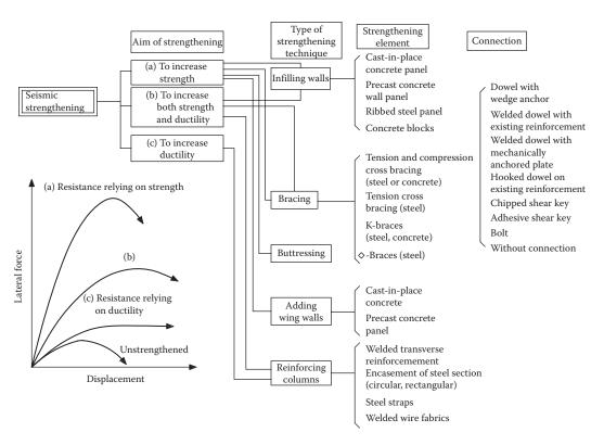
Figure 14.20 Typical strengthening methods used in Japan.
