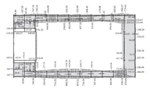
Figure 4.15 Palace—Aliki theaters, Athens, Greece. Axial forces of beams at the level of balconies due to seismic combination in the y-y direction.
