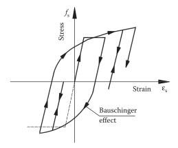
Figure 7.13 Stress-strain diagram for steel under reversed loading (Bauschinger effect). (Park, R. 1973. Theorization of structural behaviour with a view to defining resistance and ultimate deformability. Symposium on Resistance and Ultimate Deformability of Structures Acted on by Well-Defined Repeated Loads. IABSE, Lisboa, 1973. With permission of IABSE.)
