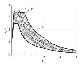
Figure 3.17 Recommended Type I elastic response spectra for ground types A–E (5% damping). (From E.C.8-I/EN1998-1. 2004. Design of Structures for Earthquake Resistance: General Rules, Seismic Actions and Rules for Buildings. CEN, Brussels, Belgium. With permission of the British Standards Institution (BSI, CEN).)
