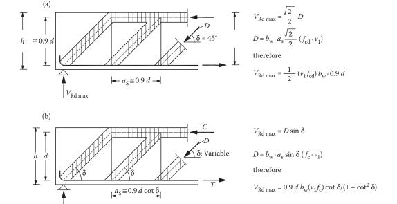
Figure 8.28 Determination of the shear resistance  $V_{\text{Rd max}}$ : (a) diagonal compression failure at  $\delta = 45^{\circ}$ ; (b) variable diagonal compression failure at 21.8°  $\leq \delta \leq 45^{\circ}$ . (Adapted from Penelis et al. 1995; Walraven, J.C. 2002. Delft, University of Technology, Background document for EN1992-1-1. Eurocode 2: Design of Concrete Structures-Chapter 6.2: Shear, Delft.)
