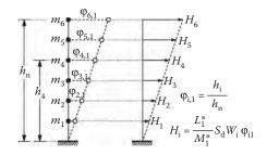
Figure 5.19 The fundamental mode of a multi-storey system and the corresponding inertial forces.
