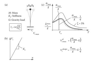
Figure 3.5 Force-based design based on 'model response spectrum analysis' or on 'lateral force method of analysis': (a) structural system under seismic action; (b)  $V_i - U_i$  diagram; (c) relation between elastic and design acceleration response spectrum.
