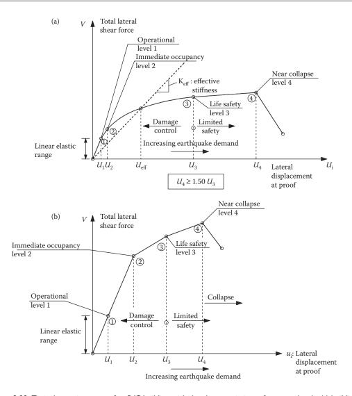
Figure 3.22 Typical capacity curve of an R/C building with the characteristic performance levels: (a) building with a ductile behaviour; (b) building with a brittle behaviour. (Adapted from FEMA 273, 274. 1997. NEHPR Guidelines for the Seismic Rehabilitation of Buildings, FEMA, Washington, DC.)
