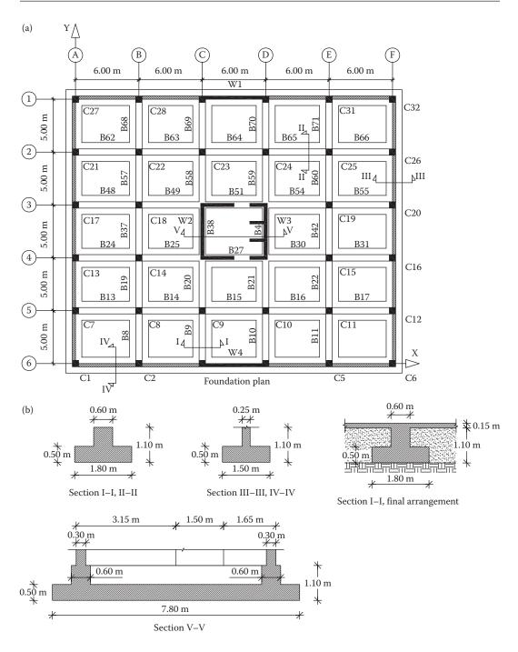
Figure 10.19 (a) Plan view of the foundation system; (b) characteristic cross-sections of the foundation beams.
