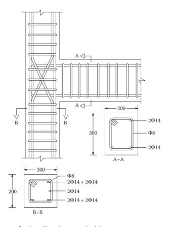
Figure 8.81 Arrangement of x-shaped bars in an exterior joint core.
