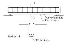
Figure 15.9 Strengthening of a T beam against bending by applying CFRP laminates.
