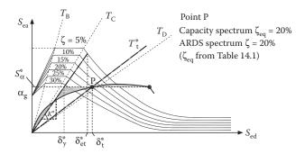
Figure 14.8 Determination of the target displacement implementing iterative procedure.
