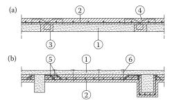
Figure 15.37 Increase of the thickness of the slab and addition of new reinforcement: (a) increase of the thickness on the upper face; (b) increase of the thickness on the lower face with the addition of new reinforcement; I = existing slab; 2 = added reinforcement; 3 = dowel; 4 = anchoring bent bars; 5 = welded connecting bars; 6 = hanging ties.
