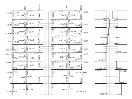
Figure 5.55 Envelope of shear forces – Grid axis C.
