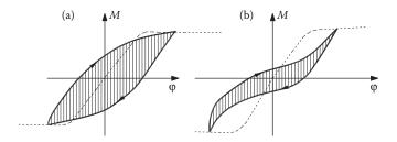
Figure 8.20 M-φ diagrams: (a) spindle-shaped loops when flexure prevails; (b) pinched loops when shear prevails.
