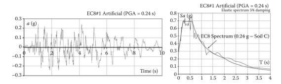
Figure 5.69 EC8 artificial strong motion records (0.24 g and soil C; left) and respective elastic spectra (right).
