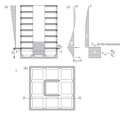
Figure 10.4 Box-type basement and its structural behaviour in relation to the superstructure (dual-system): (a) elevation; rastered area is considered to be the critical region for ductile behaviour; (b) plan view at basement; (c)  $M_{\rm Ed}$ ,  $V_{\rm Ed}$  diagrams of the structural wall core.
