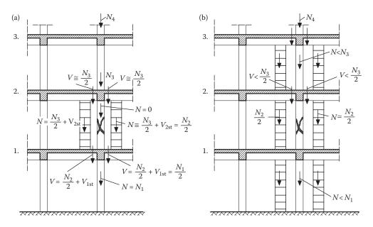
Figure 12.5 Shoring (temporary supporting) of a multi-storey building with a damaged column: (a) shoring of only one floor; (b) shoring of more floors.
