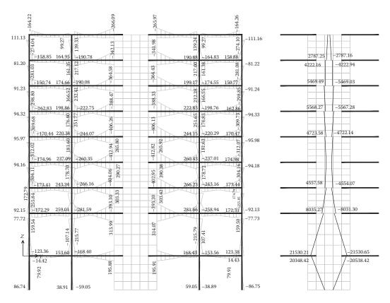
Figure 5.56 Envelope of bending moments - Grid axis C.
