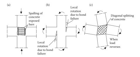
Figure 8.73 Types of failures at beam-column joints: (a) spalling of joint core; (b) anchorage failure of beam bars; (c) shear failure of the joint core.
