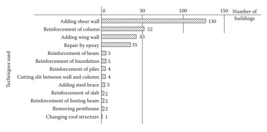
Figure 14.21 Repair and strengthening techniques used for 157 buildings in Japan.
