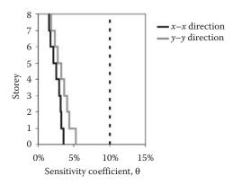
Figure 5.50 Comparison of the calculated inter-storey drift sensitivity coefficients  $\theta_i$  with the Code upper limit ( $\theta_i \le 0.10$ ).
