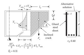
Figure 15.29 Shear force transfer through epoxy resin glued steel sheet.
