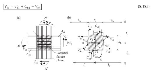
Figure 8.74 (a) Seismic actions in the joint core; (b) internal forces in the joint core (T results from tensile forces and C results from compressive forces at each face of the joint).
