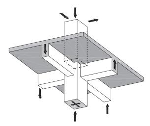
Figure 8.72 Alternative detailing of interior joints. (Adapted from Paulay, T. and Priestley, M.J.N. 1992. Seismic Design of Reinforced Concrete and Masonry Buildings. J. Wiley & Sons, New York.)
