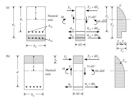
Figure 15.27 Shear stress between old and new concrete: (a) intervention in the tension zone; (b) intervention in the compression zone.
