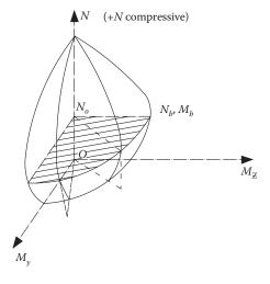
Figure 8.55 Interaction diagram of biaxial bending with axial compressive force.
