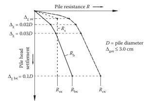
Figure 10.11  $R_c - \Delta z$  curve according to DIN 4014/1990.
