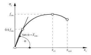
Figure 7.7 Schematic representation of the stress-strain relation of concrete for structural analysis. (Adapted from EC2-1-I/EN1992-1-1. 2004. Design of Concrete Structures—Part 1-1: General Rules and Rules for Buildings. BSI, CEN, Brussels, Belgium.)
