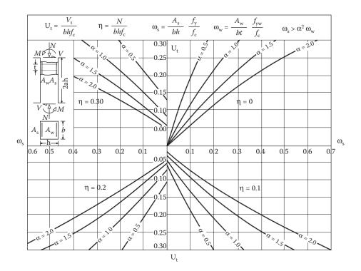
Figure 8.68 Design diagram for the calculation of shear strength in the case that  $\alpha = (M/V \cdot h) \leq 2.0$  and  $\omega_s > \alpha^2 \omega_w$ . (Adapted from Tegos, I. 1984. Contribution to the study and improvement of earth-quake-resistant mechanical properties of low slenderness structural elements. PhD thesis, Aristotle University of Thessaloniki (in Greek).)
