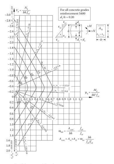
Figure 8.41 Interaction M-N diagrams and the relevant strain patterns at characteristic points. (Adapted from Zararis, P. 2002. Design Methods of Reinforced Concrete (in Greek). Kyriakides Bros. Ltd, Thessaloniki.)
