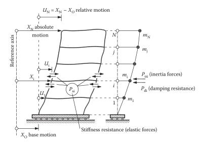
Figure 2.33 Dynamic equilibrium of elastic, damping, and inertial forces at the level of a storey (d'Alembert equation).
