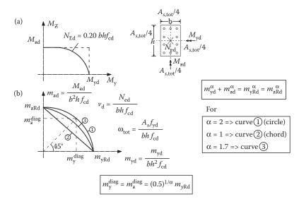
Figure 8.56  $M_y - M_z$  interaction diagrams for a given axial force N (a)  $M_y - M_z - N$ ; (b) normalised diagram of  $M_y - M_z - N$ .
