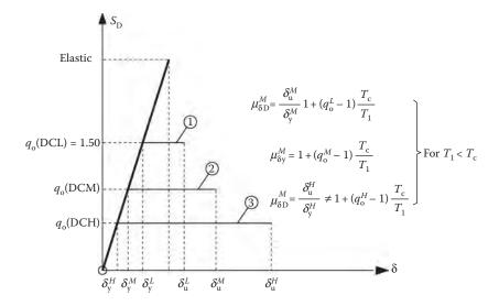
Figure 5.4 Relation between design force and ductility demand at the plateau of the design spectrum (see Chapter 3.2) for fundamental period  $T_1 < T_c$  (Equation 5.17).
