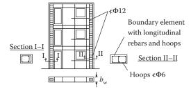
Figure 9.35 Reinforcement of a large, lightly reinforced wall.
