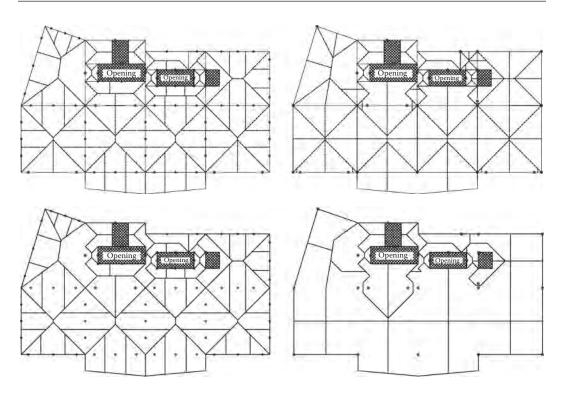
Figure 5.21 Gravity load distribution (left) and mass distribution (right).
