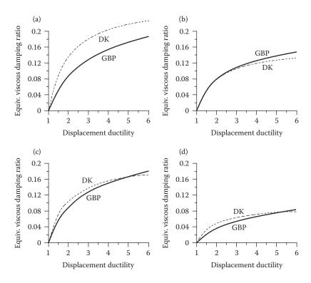
Figure 2.22 Hysteretic component of equivalent viscous damping from two independent studies. (DK indicates Dwairi and Kowalsko, 2007, GBP indicates Grant, D.N. et al. 2005.) (a) Elastoplastic; (b) thin takeda; (c) flat takeda; (d) flag,  $\beta = 0.35$ .
