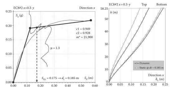
Figure 5.73 Derivation of target displacement and displacement profiles for the EC8#2 x+0.3 y excitation.
