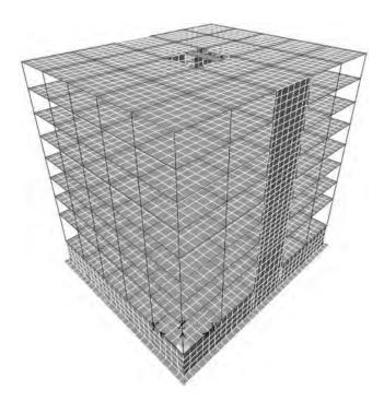
Figure 5.47 Structural model of the eight-storey building.
