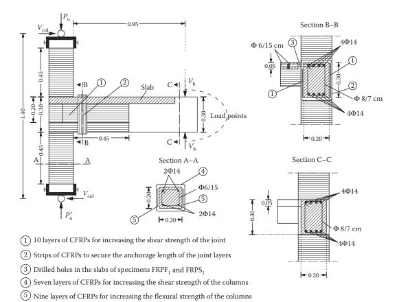
Figure 15.55 Jacketing of column and beam-column connection of subassemblages FRPFI and FRPSI (dimensions in m). (From Tsonos, A. 2008. Effectiveness of CFRP-jackets in post-earthquake and pre-earthquake retrofitting of beam-column subassemblages. Engineering Structures, 30, 777-793. Copyright 2008, with permission from Elsevier.)
