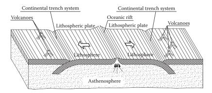
Figure 3.10 Motion system of lithospheric plates.
