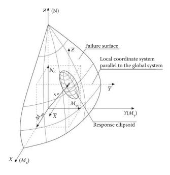
Figure 5.38 Response ellipsoid and failure envelope.
