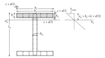
Figure 9.20 Determination of the confined region of a composite cross-section.
