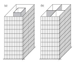
Figure 4.31 Dual system (a) Tube-in-tube system; (b) external tube combined with shear walls. (From König, G. and Liphardt, S. 1990. Hochhäuser aus Stahlbeton, Beton Kalender, Teil II, 457–539. Copyright Wiley-VCH Verlag GmbH & Co. KGaA. Reproduced with permission.)
