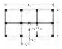
Figure 5.20 Evaluation of the torsional effects on a symmetric system with the aid of an amplification factor.
