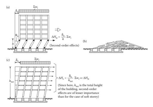
Figure 6.1 Plastic mechanism of a frame system with strong beams – weak columns. (a) Generation of a soft storey. The second order effects lead to an overturning of the formed inverted pendulum; (b) pancake collapse pattern; (c) a frame system with strong columns – weak beams. This ensures the existence of a strong vertical spine preventing collapse.
