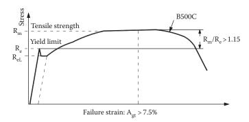
Figure 7.15 Stress-strain diagram of steel B500C (EN 10080).
