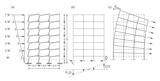
Figure 4.20 Frame system under lateral loading. (a) Moment diagram; (b) axial forces at the columns (opposite sign); (c) displacements due to axial strain of columns.
