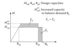
Figure 14.22 Strength of a member increased to balance the deformation  $\theta_{ud}$  inefficiency to cover the deformation demand  $\theta_{E}$ .
