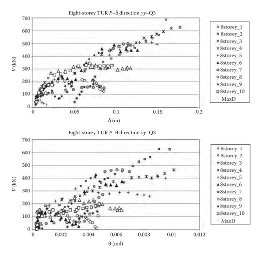
Figure 5.35 IDA of an eight-storey torsionally unrestrained MRF (V- $\delta$  and V- $\theta$  charts).
