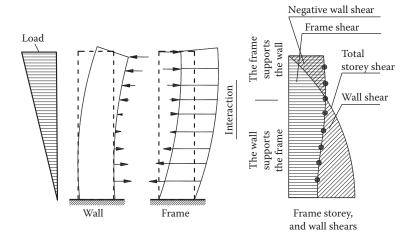
Figure 4.23 Interaction between frame and shear wall in a dual system under lateral loading.
