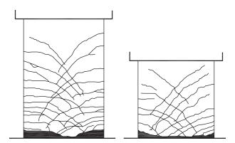
Figure 9.30 Crack patterns for Specimens MSWI and LSW3 at the end of the experiment. (From Salonikios, T. 2007. Analytical prediction of the inelastic response of R/C walls with low aspect ratio. ASCE Journal of Structural Engineering, 133(6), 844–854. With permission of ASCE.)
