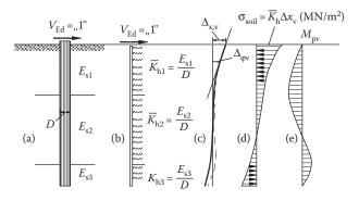
Figure 10.15 Response of a long pile to  $V_{\text{Ed}} = \text{-l}^{\text{I}}$  using the Winkler model: (a) soil layers and pile position; (b) 'Winkler' model; (c) soil stiffness  $\overline{K}_{vv} = (\text{-l}^{\text{I}}/\Delta x_v), K_{\phi v} = (\text{-l}^{\text{I}}/\Delta \phi_v)$ ; (d) soil reactions  $\sigma_{\text{soil}} = \overline{K}_h \Delta x_v (\text{MN/m}^2)$ ; (e) pile bending moments.
