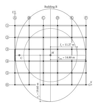
Figure 2.58 Definition of torsional rigidity in Building B.
