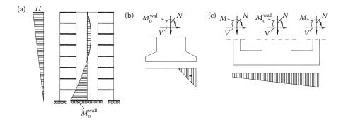
Figure 4.16 Foundation issues of shear (ductile) walls (a) wall response in a dual system under lateral loading; its behaviour maybe simulated to a one end fixed cantilever supported by a spring at the other end (b) wall foundation on a pad; overturning risk; (c) connections of the wall with the external columns with a foundation beam: diminishing of the risk of overturning due to enhancement of the total axial force and broadening of the foundation basis.
