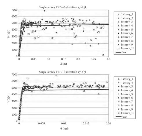
Figure 5.32 Torsionally restrained single-storey building  $V-\delta$  and  $V-\theta$ .
