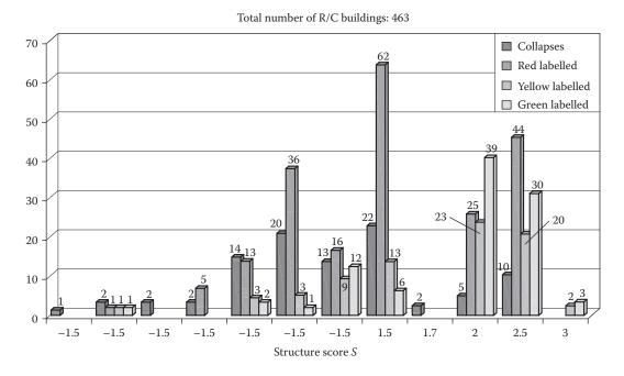
Figure 13.7 Distribution of the structural score to the R/C buildings of the most affected area of Athens due to the earthquake of 1999. (From Karabinis, A. 2002. Validation of the pre-earthquake assessment procedure of R/C buildings in Greece, Technical Report (OASP) Athens, Greece.)
