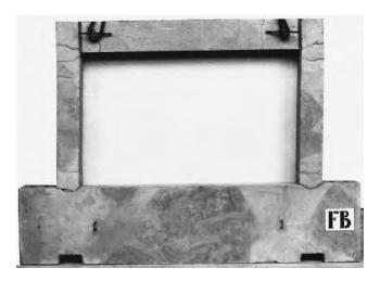
Figure 8.85 Failure mode of bare frame FB. (Adapted from Stylianidis, K. 2012. Journal of O.C.B.T., 6, 194-212.)
