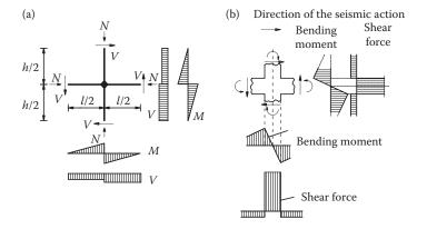
Figure 8.7 (a) M-V diagrams of a frame sub-assemblage due to seismic action (sway); (b) magnification of  $\dot{M}$ -V diagrams in the region of the joint.
