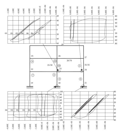
Figure 2.53  $M-\theta$  diagrams at critical sections of the 3-storey frame of Figure 2.52 designed according to the Greek Code of 1959.
