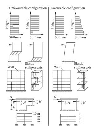
Figure 4.5 Distribution of mass and stiffness in elevation.
