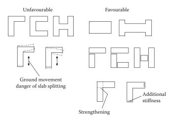
Figure 4.2 Unfavourable and favourable geometric configuration in plan.
