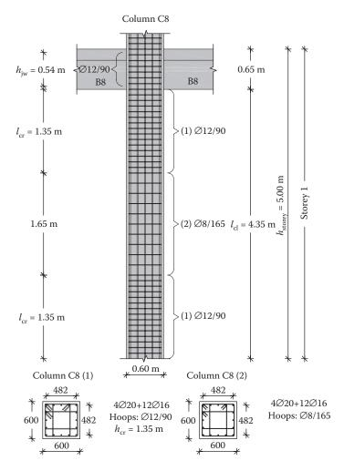
Figure 8.102 Flexural and shear reinforcement of column C8.
