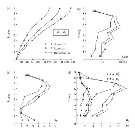
Figure 2.54 Maximum response parameters of a frame system (GRFR8) subjected to a seismic excitation with  $SI = 1.0 SI_0$  for the El Centro x 1.0, Pacoima x 0.4, and Thessaloniki x 2.6 earthquakes: (a) floor displacements; (b) inter-storey drifts  $\Delta x/h$ ; (c) required column ductilities; (d) required beam ductilities.
