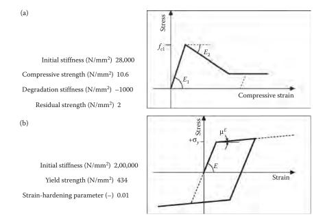
Figure 5.63 Material models (concrete - steel) for fibre analysis: (a) concrete; (b) steel reinforcement.
