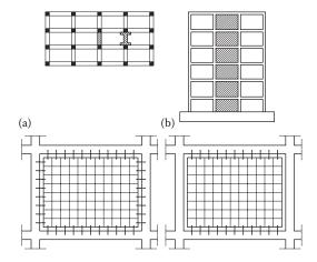
Figure 15.59 Addition of new R/C walls inside a frame: (a) connection along the four sides; (b) connection only with the beams.
