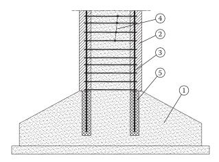
Figure 15.40 Anchorage of the column jacket reinforcement in the footing: I = old concrete; 2 = jacket; 3 = long reinforcement; 4 = new ties; 5 = epoxied connections.
