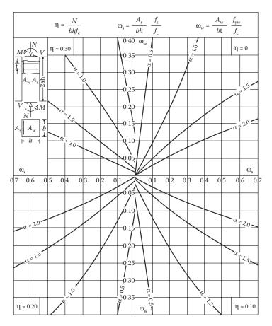
Figure 8.69 Design diagram for the calculation of shear reinforcement (hoops) in the case of  $\alpha = (M/V \cdot h) \leq 2.0$ . (Adapted from Tegos, I. 1984. Contribution to the study and improvement of earthquake-resistant mechanical properties of low slenderness structural elements. PhD thesis, Aristotle University of Thessaloniki (in Greek).)
