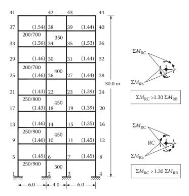
Figure 6.5 Values of the magnification factors  $\alpha_{\text{CD}}$  for a 10-storey, 4-column R/C frame.
