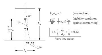
Figure 6.11 Stability condition against overturning.
