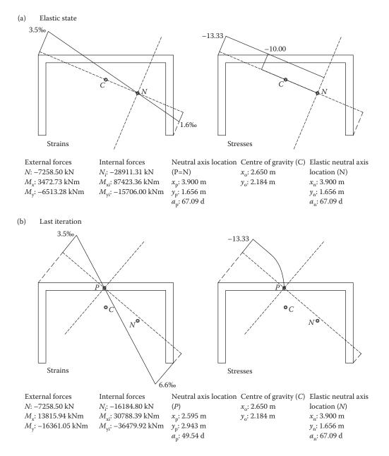
Figure 9.52 W2 cross-section equilibrium: (a) at the elastic state, and (b) at the final iteration step.
