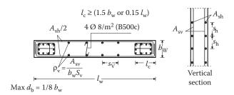
Figure 9.15 Arrangement of horizontal and vertical reinforcement in walls with a rectangular cross-section.
