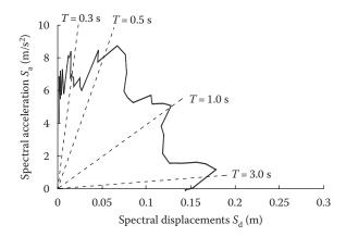
Figure 2.15 Capacity displacement spectrum (ADRS).
