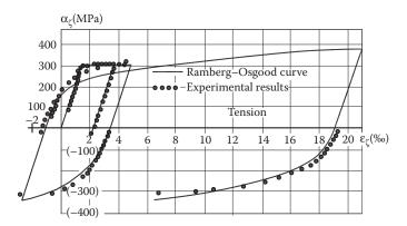
Figure 7.14 Modeling of the cyclic loading of steel bars and comparisons with relevant test data. (From Park, R. and Paulay, T. 1975. Reinforced Concrete Structures. Copyright Wiley-VCH Verlag GmbH & Co. KGaA. Reproduced with permission.)
