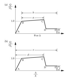
Figure 5.25 Point hinge constitutive law suggested by U.S. guidelines. (a) Deformation; (b) deformation ratio.
