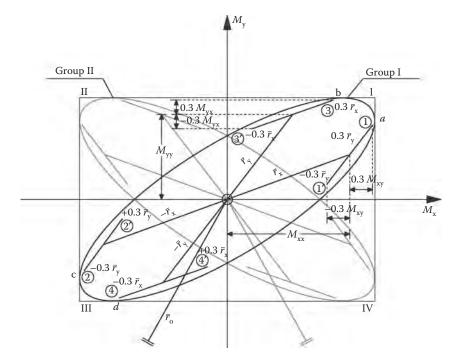
Figure 5.40 The Rosenblueth and Contreras procedure (alternative Code procedure).
