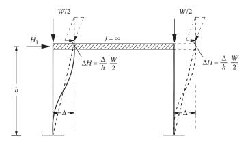
Figure 6.12 Second-order effect on a one-storey, two-column frame.
