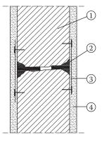
Figure 15.43 Repair of a through-thickness crack in an infill wall: I = existing masonry walls; 2 = sealing of the crack with cement mortar; 3 = wire mesh; 4 = plaster.
