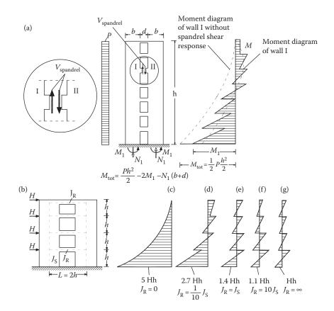
Figure 4.22 (a) Response of coupled shear walls under lateral loading; (b) to (g) the influence of the spandrel stiffness on the moment diagrams of the walls.
