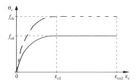
Figure 7.8 Parabola-rectangle diagram for concrete under compression for design. (Adapted from EC2-I-I/EN1992-I-I. 2004. Design of Concrete Structures—Part I-I: General Rules and Rules for Buildings. BSI, CEN, Brussels, Belgium.)
