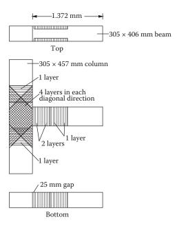
Figure 15.54 CFRP-strengthened specimen tested by Clyde and Pantelides. (Adapted from Clyde, C. and Pantelides, C.P. 2002. Seismic evaluation and rehabilitation of R/C exterior building joints. Proceedings of the Seventh U.S. National Conference on Earthquake Engineering, Georgia Institute of Technology, Boston, USA.)
