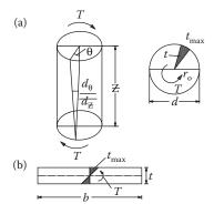
Figure 9.39 Torsion according to Saint-Venant theory (Zero axial strain of the cross-sections): (a) notation for uniform torsion, and
