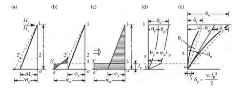
Figure 5.9 Moment—curvature displacement diagrams of an R/C cantilever beam: (a) loading pattern at yield and failure; (b) curvature diagram at yield and failure; (c) definition of the plastic rotation at the fixed end; (d) rotation of the plastic rotation at the fixed end; (d) rotation diagram at yield and failure; (e) displacement diagram at yield and failure.
