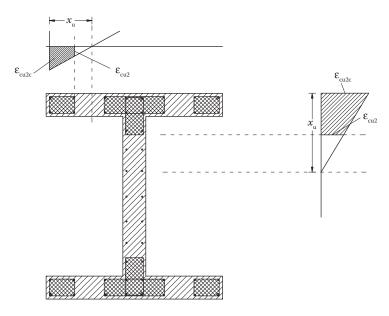
Figure 9.21 Determination of the confined regions of a composite cross-section based on the assumption of sacrificed flanges.
