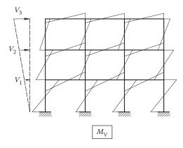
Figure 8.2 Bending moment diagram for horizontal seismic actions.
