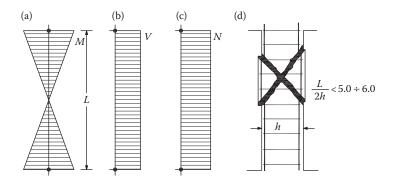
Figure 11.4 Column damage due to strong axial compression and shear (a) bending diagram; (b) shear force diagram; (c) axial force diagram; (d) sketch damage.
