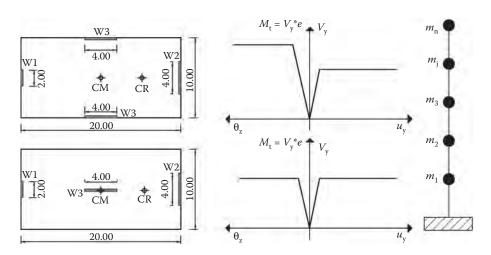
Figure 5.30 Torsionally restrained (TR-top) and torsionally unrestrained (TUR-bottom) multi-storey buildings.
