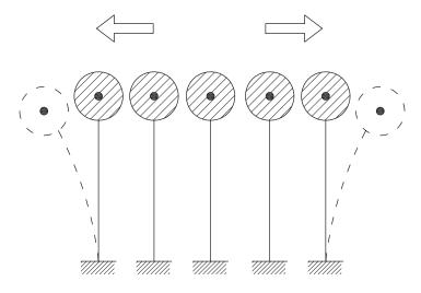
Figure 11.50 Transfer of energy at the end of SDOF oscillators in a series of adjacent systems.
