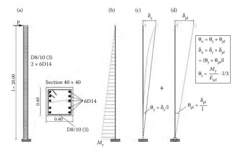
Figure 5.57 Cantilever with lateral loading: (a) geometry; (b) moment diagram at yield; (c) deflexion at yield; (d) post-yield plastic deflexions.
