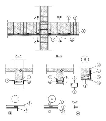
Figure 15.24 Strengthening of a beam on the lower face: I = existing reinforcement; 2 = existing stirrups; 3 = added longitudinal reinforcement; 4 = added stirrups; 5 = welded connecting bar; 6 = welding; 7 = collar of angle profiles.
