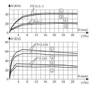
Figure 8.91 Program #2. Lateral load-displacement envelopes of bare frames  $F_{1,1,8}$ , and  $FN_{1,1,6}$  infilled frames  $F_{1,1,6}$  and  $FN_{1,1,6}$ . (Adapted from Stylianidis, K. 2012. *Journal of O.C.B.T.*, 6, 194–212.)
