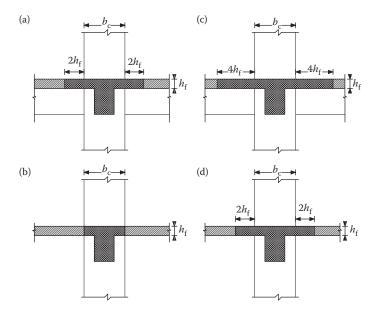
Figure 8.32 Effective flange width b<sub>eff</sub> for beams framing into columns: (a) exterior column with transverse beam; (b) exterior column without transverse beam; (c) interior column with transverse beam; (d) interior column without transverse beam. (Adapted from E.C.8-I/EN1998-I. 2004. Design of Structures for Earthquake Resistance: General Rules, Seismic Actions and Rules for Buildings. CEN, Brussels, Belgium.)
