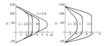
Figure 8.63 Application for dimensional M-N and V-N of 200 mm square column with four 16 mm bars (CEB, 1996a; Adapted from Fardis, M.N. 2009. Seismic Design, Assessment and Retrofitting of Concrete Buildings. Springer, Heidelberg.)
