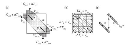
Figure 8.75 Shear transfer mechanism in a joint core: (a) diagonal concrete strut; (b) truss mechanism; (c) typical components of the truss.
