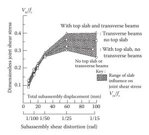
Figure 8.77 Effect of top slab and/or transverse beam on both sides on the ultimate shear strength of interior joints. (Adapted from Kitayama, K., Otani, S. and Aoyama, H. 1991. Development of design criteria for R/C interior beam-column joints, ACI Special Publication SPI23, American Concrete Institute, Detroit, Michigan, 97–124.)
