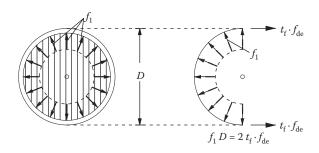
Figure 15.53 Confinement of a circular cross-section by wrapping with FRP sheets.
