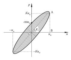
Figure 2.18 Diagram of the restoring force P versus relative displacement u for an excitation  $u = u_0 \sin \omega t$  of an SDOF with damping c.
