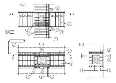
Figure 15.31 Strengthening of a joint with a jacket: I = column reinforcement; 2 = beam top reinforcement; 3 = beam bottom reinforcement; 4 = joint vertical stirrups; 5 = beam stirrups; 6 = column ties; 7 = column ties in joint.
