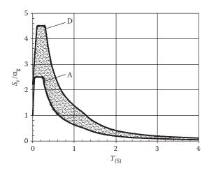
Figure 3.18 Recommended Type 2 elastic response spectra for ground A–E (5% damping). (From E.C.8-1/EN1998-1. 2004. Design of Structures for Earthquake Resistance: General Rules, Seismic Actions and Rules for Buildings. CEN, Brussels, Belgium. With permission of the British Standards Institution (BSI, CEN).)
