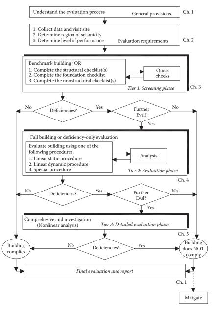
Figure 13.8 Evaluation process according to ASCE 31-02/FEMA 310/1998. (From FEMA-310/1998/ASCE 31-02. Handbook for the Seismic Evaluation of Buildings—A standard prepared by the ASCE for the Federal Emergency Management Agency, Washington, DC. With permission.)
