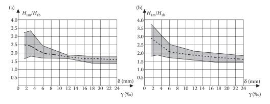
Figure 8.90 Program #1. Ratio of infilled frames to bare frames strength. (a) Models without axial force (b), models with axial force. First cycles only. (Adapted from Stylianidis, K. 2012. *Journal of O.C.B.T.*, 6, 194–212.)
