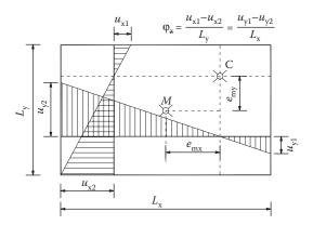
Figure 2.42 Determination of the centre of stiffness and the torsional rigidity with respect to the centre of stiffness, using a computer-aided procedure.
