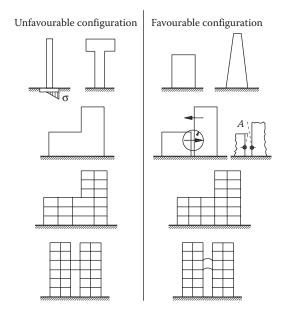
Figure 4.4 Unfavourable and favourable configuration in elevation.
