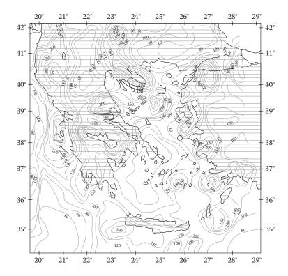
Figure 3.14 Maximum accelerations in gal (1000 gal = g) with a 90% probability to not be exceeded in 25 years reference period (Greece).
