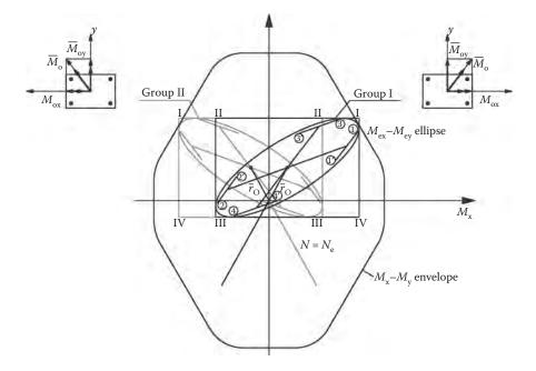
Figure 5.42 Choice of the proper ellipse (group I or group II) in regard to the position of the gravity load effects vector  $\overline{r}_0$  in the quarters of the capacity envelope of a symmetric cross-section.
