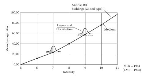
Figure 16.5 Mean damage ratio at different intensity levels of midrise R/C buildings after CAR and BU. (Adapted from Erdik, M. and Aydinoğlu, N. 2000. Earthquake vulnerability of buildings in Turkey. Internal report, Boğaziçi University, Istanbul.)
