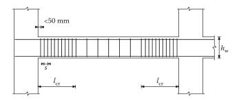
Figure 8.35 Transverse reinforcement in critical regions of beams. (Adapted from E.C.8-I/EN1998-1. 2004. DesignofStructuresforEarthquakeResistance:GeneralRules,SeismicActions and Rules for Buildings. CEN, Brussels, Belgium.)
