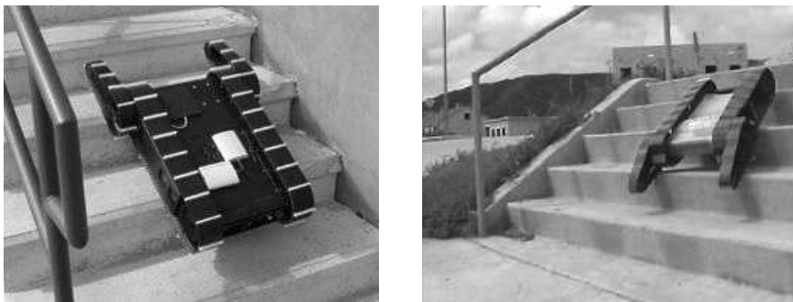
EXHIBIT 14-7 Alpha (left) and beta (right) prototypes of the PackBot.
