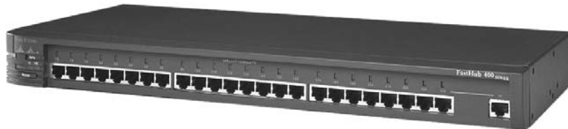
Figure 2-23 Hubs Have Several Ports
