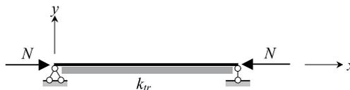
FIGURE 8.2. Beam on an elastic foundation.
