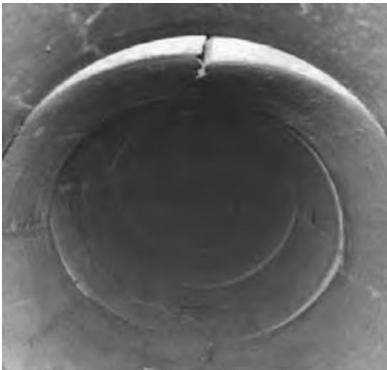
Figure 8.6 The inside of the broken rigid pipe test section after loading to a vertical soil pressure of 5040 \text{ lb/ft}^2 (equivalent burial depth of 42 ft).
