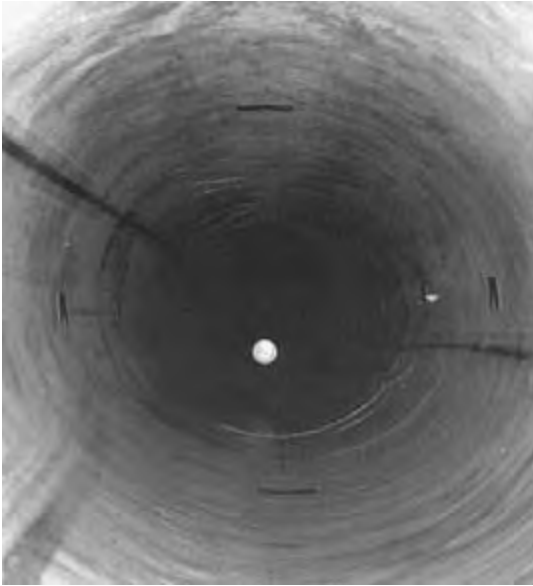
Figure 8.7 The inside of the lined broken rigid pipe test section. The vertical soil pressure is 5040 \text{ lb/ft}^2 (equivalent burial depth of 42 ft).
