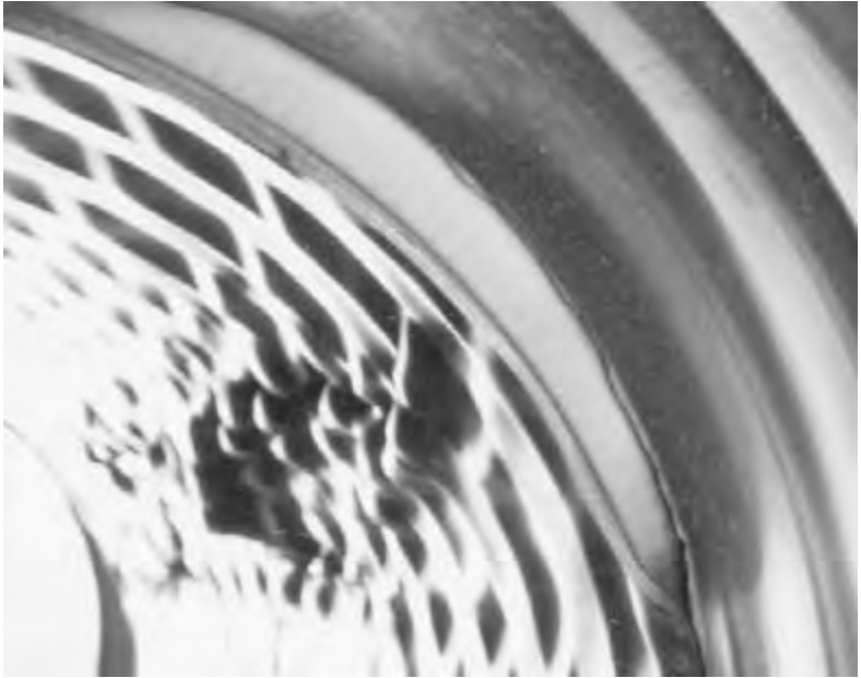
Figure 7.49 Test X-5, waffling pattern and local buckling (25 m of cover).
