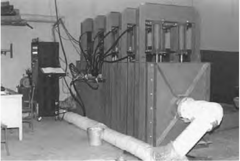
Figure 6.57 Soil load cell showing the insulation used on return piping.
