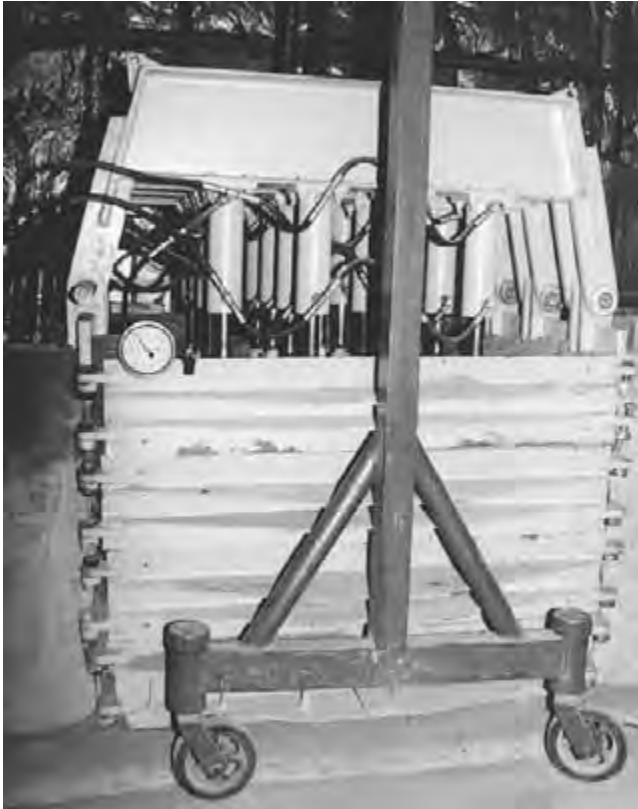
Figure 6.10 Test cell in operation—pistons of cylinders extended.
