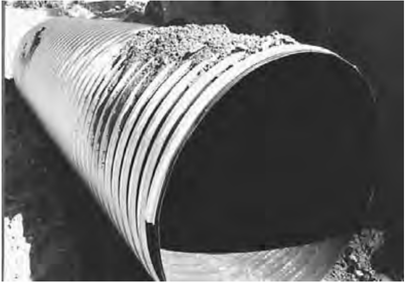
Figure 7.45 Test pipe being placed in test cell.
