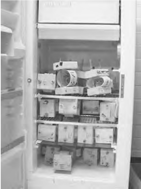
Figure 7.5 Stress relaxation specimens in the refrigerator at 40°F.
