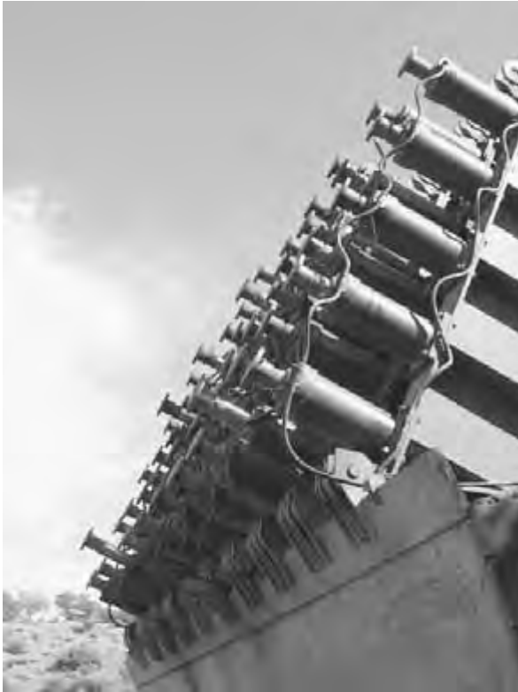
Figure 7.56 Photograph showing the 50 hydraulic cylinders used for loading.
