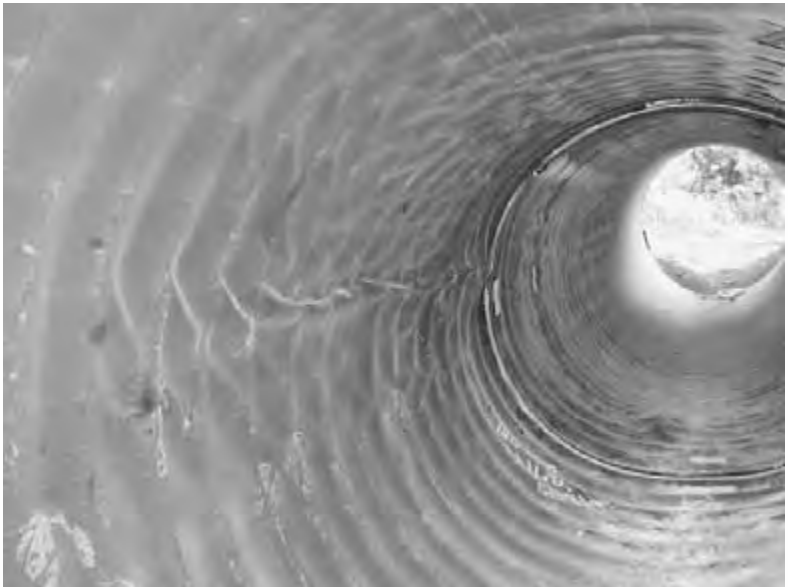
Figure 7.74 Wall crushing and dimpling pattern on left side. Density = 95 percent, and load is 152 ft of cover.
