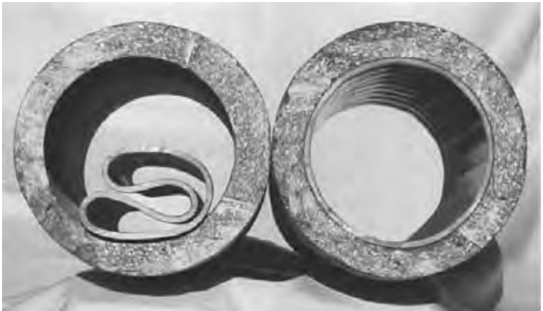
Figure 8.13 Portrayal of the folded pipe as inserted and how it appears after expansion. (Courtesy of Ultraliner.)
