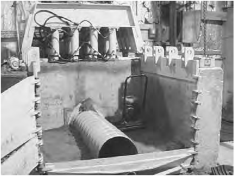
Figure 6.21 An 18-in ribbed pipe is being installed in small soil load cell at Utah State University.
