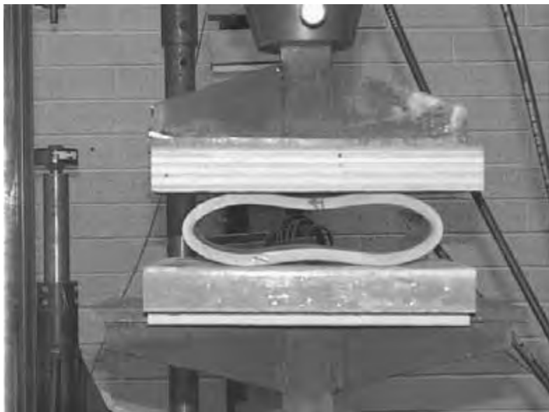
Figure 4.11 Prequalification flattening test (after flattening).
