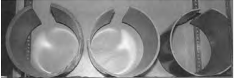
Figure 7.18 Control of frozen-in stresses in PVC pipe samples.
