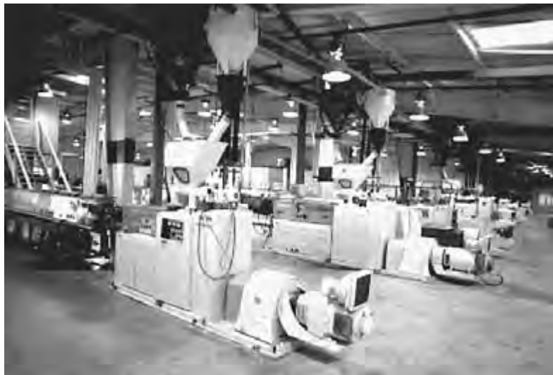
Figure 7.2 PVC pipe extrusion plant. (Reprinted by courtesy of Uni-Bell PVC Pipe Association.)
