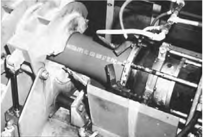
Figure 7.3 PVC pipe belling operation. (Reprinted by courtesy of Uni-Bell PVC Pipe Association.)
