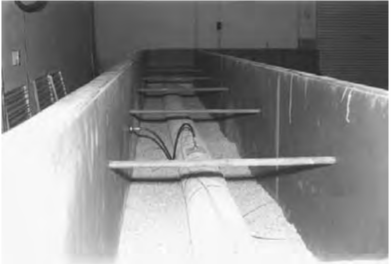
Figure 6.60 High-temperature pipe installed in the test cell. Note the following: (1) joints misaligned by 1.5^\circ , (2) thermocouple wire running along pipe, (3) fitting and hose for water damage test.
