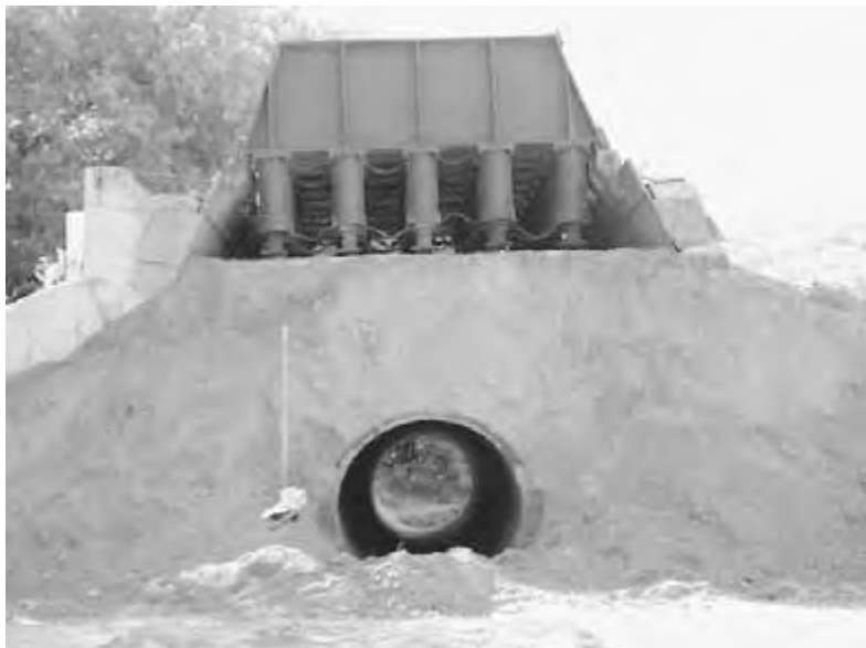
Figure 7.60 Soil cell full, loading beams down, and load being applied to soil surface.
