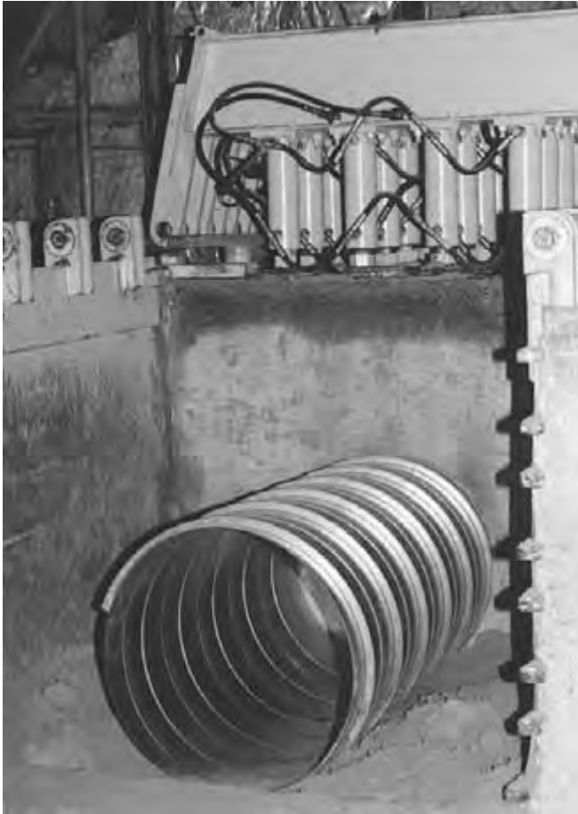
Figure 6.9 Placement of ribbed steel pipe in test cell.
