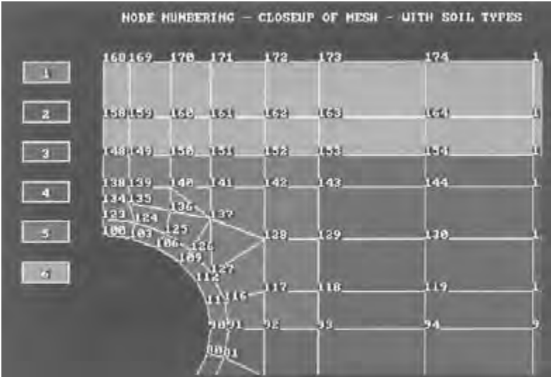
Figure 3.45 Printed output showing node numbering scheme of upper part of mesh in an FEA model.
