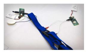
Figure 2: The AutoSense wearable sensor system includes six sensing modalities including ECG, respiratory inductive plethysmograph (RIP), and three-axis accelerometer.
