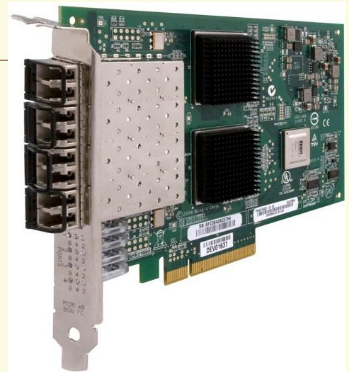
Qlogic 8Gb Quad Port FC HBA, x8 PCIe, LC multi-mode optic
