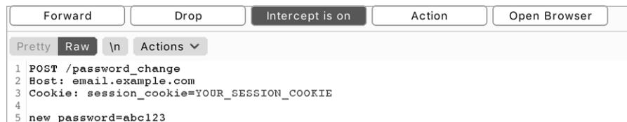
Figure 9-3: Set to **Intercept is on** to capture your browser's traffic. Click the **Forward** button to forward the current request to the server.
