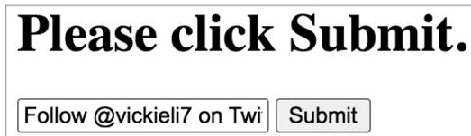
Figure 9-2: An example HTML form that an attacker uses to exploit a CSRF vulnerability
