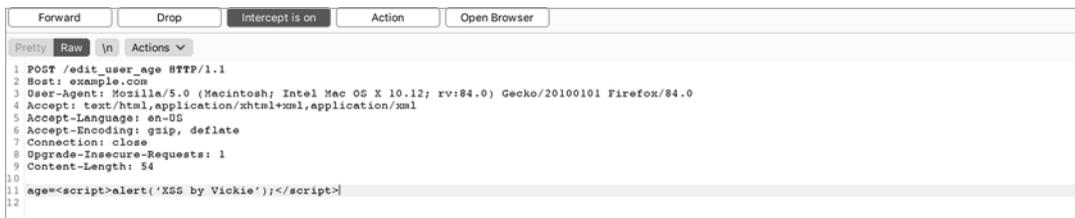
Figure 6-7: Change the URL post request parameter to your XSS payload.
