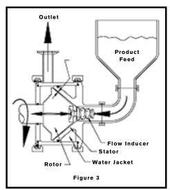
By decreasing the distance between the rotor and stator, shear on the product is increased; however, there are limitations in this procedure. Decreasing the gap will also substantially decrease the flow rate and increase the temperature rise in the product. Figure 3 shows a new design for a patented APV colloid mill (US Patent 6,305,626).
