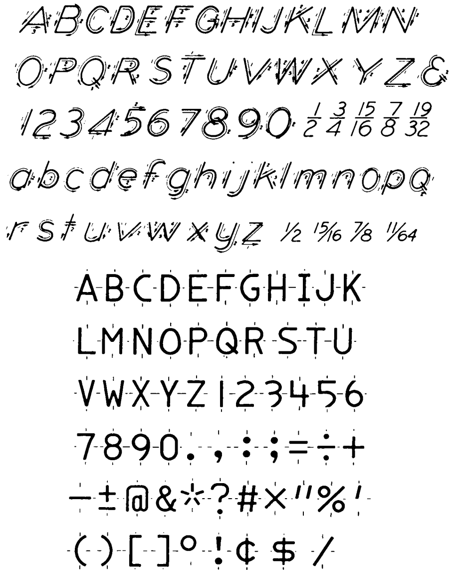
Fig. 3.2. Lettering and symbols and lettering styles (adapted from AISC practice)
