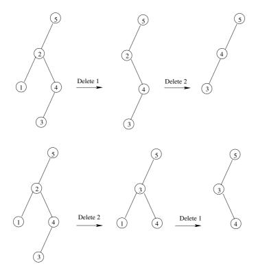
Figure 1: Two deletions where the order of the operations matter.
