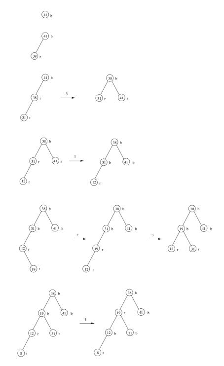
Figure 2: Inserting 41, 38, 31, 12, 19, 8 into a red-black tree. The arrows indicate transformations. Notice that the root is always coloured black
