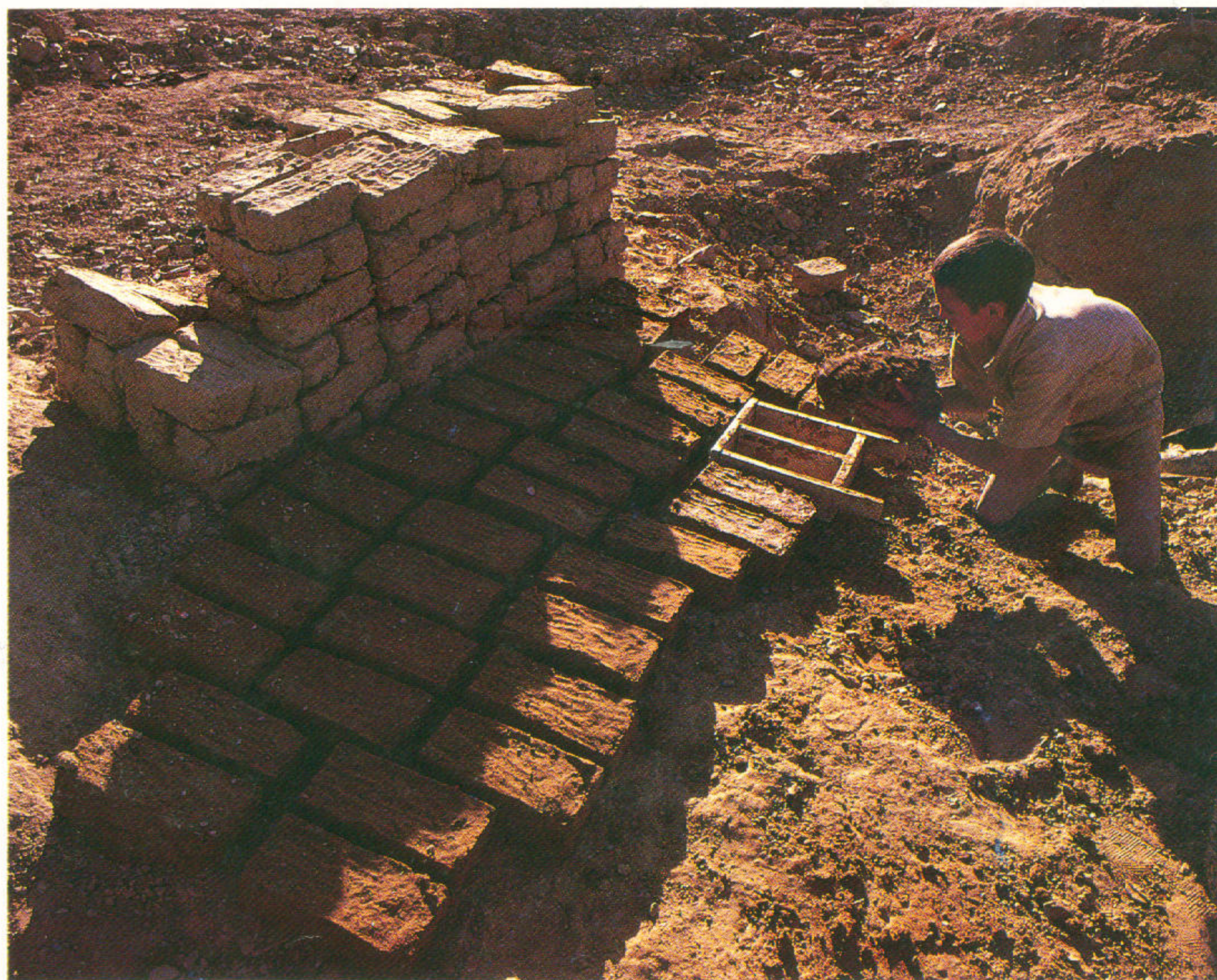
Pl. 5. Making mud bricks with a double mold.
