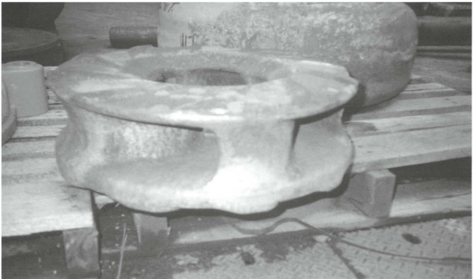
Figure 2.2 Impeller of ash slurry pump, showing general erosion
