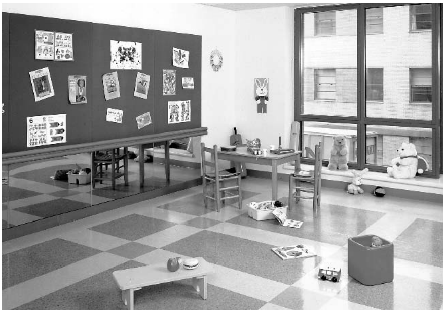
◀ The typical classroom at the Coleman School in the New York Foundling Hospital, New York City, is designed to let severely disabled students sit on the floor. It includes a mirror at eye level, low windowsills, radiant heating, and a flexible layout. Perkins Eastman Architects.
