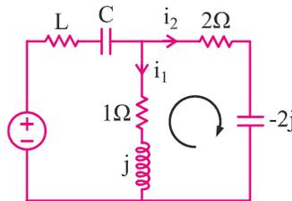
$$\text{KVL: } -(1+j)i_1 + (2-2j)i_2 = 0 \rightarrow (1+j)i_1 = (2+2j)i_2 \rightarrow i_1 = 2i_2$$
