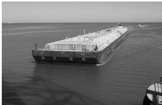
FIGURE 4.6 Tanker barge approaching a bridge. Note the bow depth of at least 1.8 m and the four push knees.
