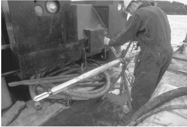
FIGURE 7.7 In situ vane shear device.
