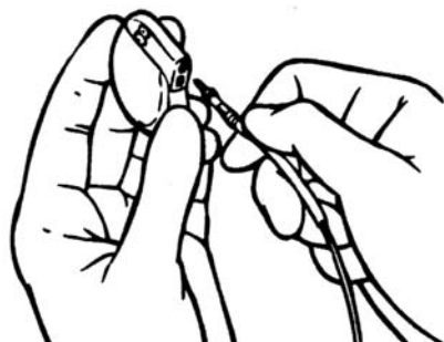
Figure 24-21. Insertion of lead to connector block. Source: From Thera DR: Product Information Manual. Minneapolis, MN: Medtronic; 1995:UC9403918EN.
