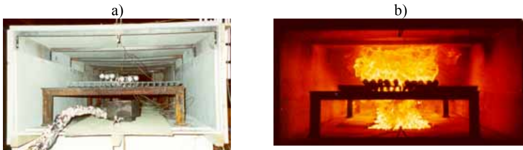
Figure 31. a) Positioning of the burner under the cables. b) View of the burning at ca. 8 minutes after burner ignition (the 10 cable experiment).
