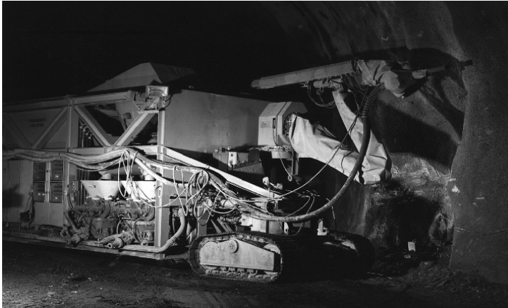
Figure 2-64 Tunnel concrete spraying machinery on electro-hydraulically driven tracks; Mobil-Crete-Spritzbeton GmbH
