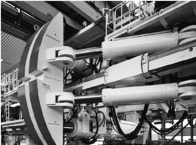
Figure 6-45 Grippers with thrust cylinders, Gripper TBM S-167 (Herrenknecht AG) Lötschberg Base Tunnel, Steg section [242]
