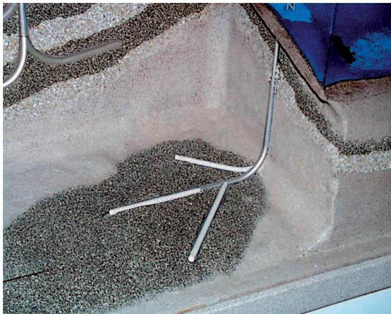
Figure 4.20 Model of multilateral well to increase reservoir contact.
