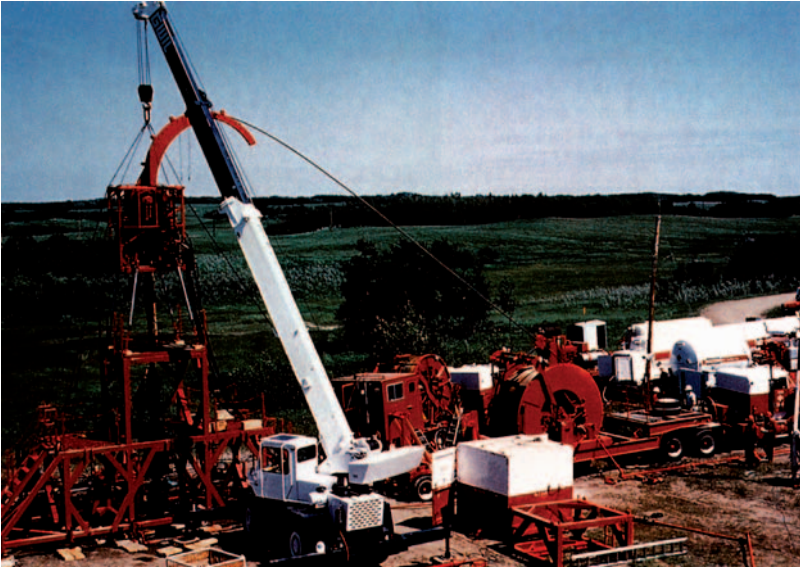
Figure 4.23 Coiled tubing drilling unit.
