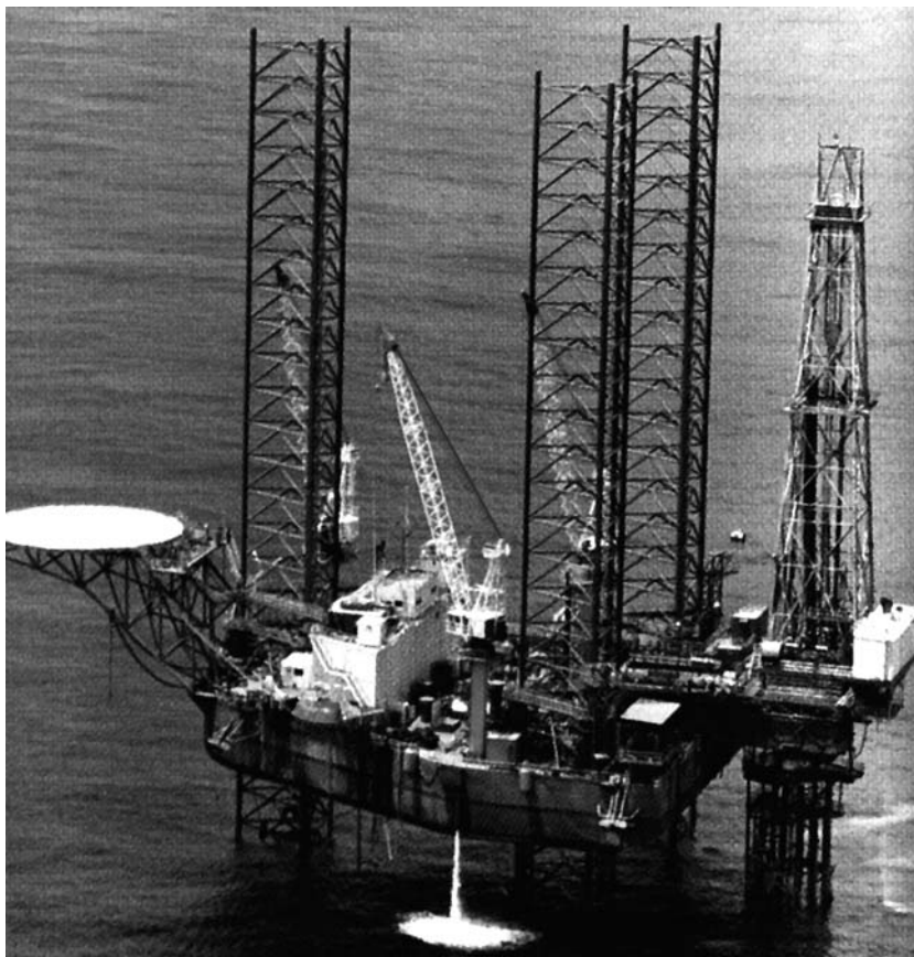
Figure 4.2 Jack-up rig (courtesy of Reading & Bates, UK).
