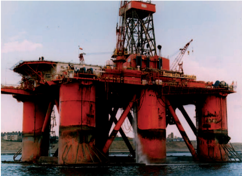
Figure 4.3 Semi-submersible rig (courtesy of Stena Drilling).
