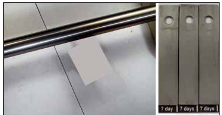
Figure 12 - Engineering Film Technology focused on chemistries that can enrich the metal oxide interface and build the capping layer without the use of metals under low hardness conditions. EXP2 was successful at passivating under low hardness conditions and was transferred over to synthetic cycled cooling water. Below are photos of the low carbon steel heat transfer tube and coupons after seven days with residual chlorine levels of 0.3 ppm.
