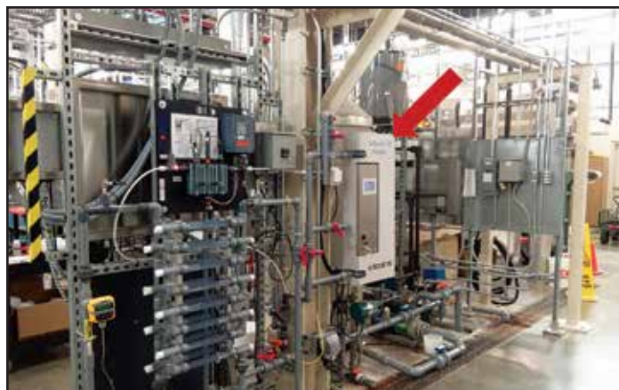
Figure 2. Overview of pilot scale testing apparatus. Biofilm monitoring and control device (indicated by arrow) is located on the center-right and biofilm sampling rack is on the left side of the image.
