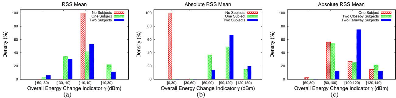
**Figure 1: In terms of overall energy change indicator  $\gamma$ , (a) “RSS Mean”, for zero, one, and two subjects. (b) “Absolute RSS Mean” for the same measurement shows better discrimination between zero and more than zero subjects. (c) Two subjects separated by more than 4 meters are clearly distinguishable from one subject.**
