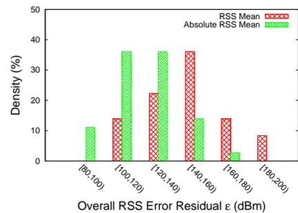
**Figure 2: The RSS residual error forms a double-sided distribution when using RSS mean, while it is approximately single-sided distributed using absolute RSS mean.**
