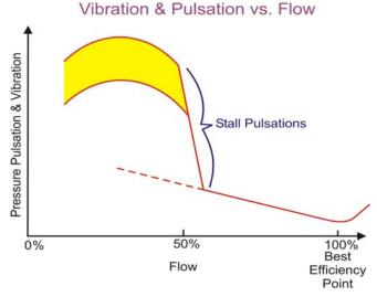
Figure 11. Effect on Vibration on Off-BEP Operation
