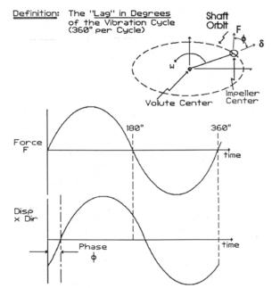
Figure 2. Definition of Phase Angle
