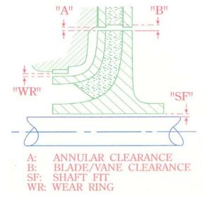
Figure 13. Various Impeller Gaps of Importance
