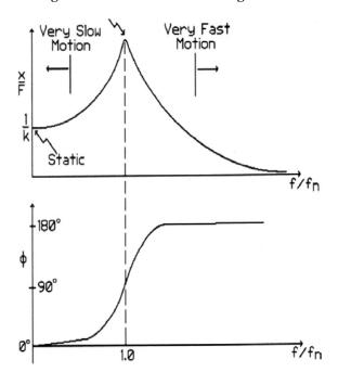
Figure 3. Relationship of Phase Angle to Frequency
