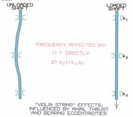
Figure 16. Vertical Pump Lineshaft Rotor Behavior
