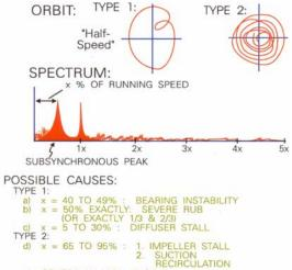
Figure 9. Subsynchronous Vibration
