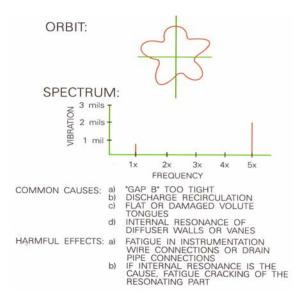
Figure 12. Vane Pass Vibration
