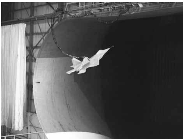
Free-flight evaluation of the dynamic stability and control of a powered model of the YF-22 fighter prototype at high angles of attack in the Langley Full-Scale Tunnel. The model was powered with compressed air ejectors and included thrust-vectoring engine nozzles and a nose boom equipped with angle-of-attack and sideslip vanes and sensors for implementation of critical flight control system elements of the full-scale aircraft. The outstanding behavior of the model at high angles of attack was subsequently verified by the airplane.
