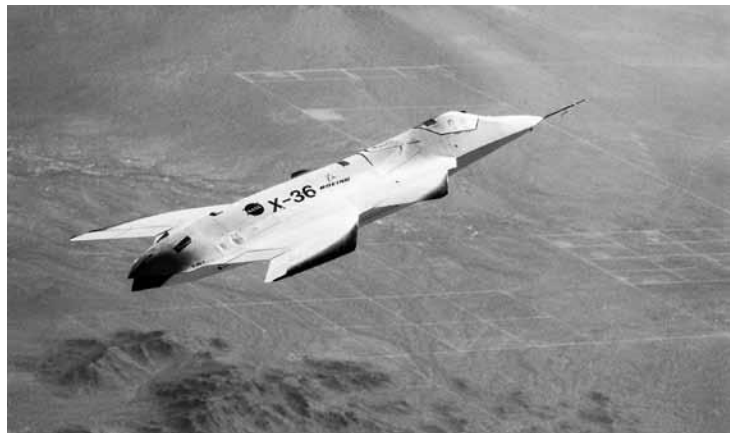
The X-36 Tailless Fighter Agility Research Aircraft in flight. The sophisticated model demonstrated that a tailless, low-signature configuration could achieve high levels of maneuverability through the use of advanced technology.
