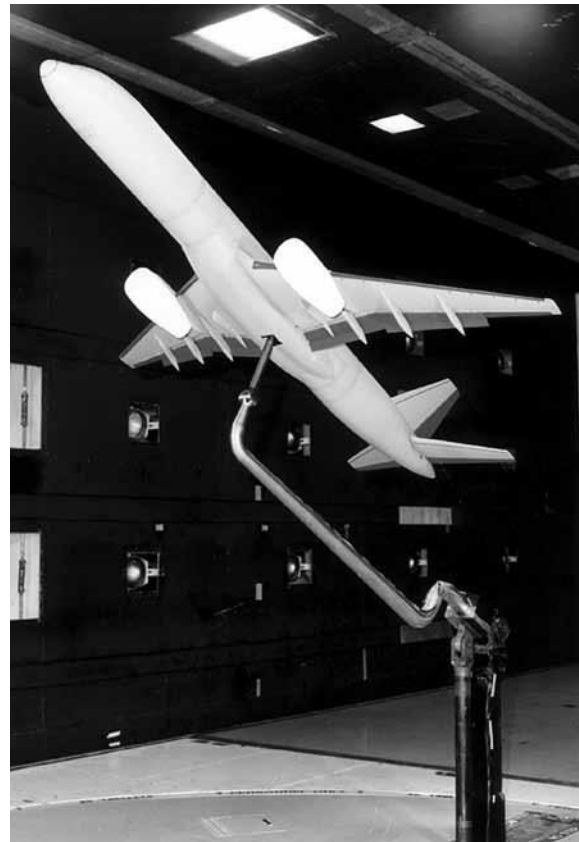
In preparation for model flight tests in the AirSTAR project, Langley has conducted conventional and dynamic force tests in the 14- by 22-Foot Tunnel to measure the aerodynamic characteristics of the configuration.
