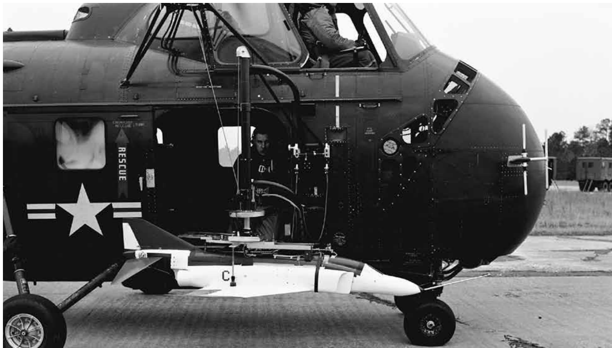
Drop model of the F-4 fighter mounted on launch helicopter during an evaluation of spin resistance in 1960 at the West Point, VA, airport. After the altitude and speed for launch conditions were satisfied, the model was lowered on a vertical shaft and released.
