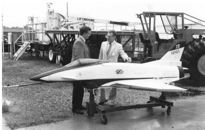
The X-31 drop model is inspected in 1991. The drop program ran simultaneously with the full-scale flight program being conducted at Dryden, providing real-time support for problems that occurred in flight.
