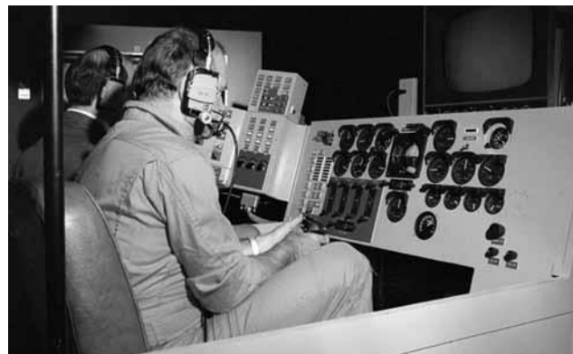
NASA research pilot Bill Dana flies the HiMAT vehicle from a fixed-base ground cockpit.
