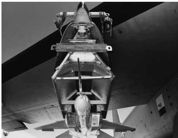
F-15 spin research vehicle mounted to a pylon on its B-52 launch aircraft. The unpowered drop model was the first in a long line of remotely piloted subscale models and was used in conjunction with a piloted simulator at Dryden and a smaller F-15 drop model at Langley to define spin entry maneuvers for the F-15 aircraft.
