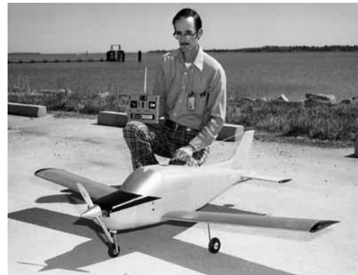
NASA conducted research on the spinning characteristics of general aviation designs in the mid-1970s with powered radio-controlled dynamically scaled models using modified hobbyist-type gear. These dynamically scaled models were significantly heavier than conventional hobbyist radio-controlled models.
