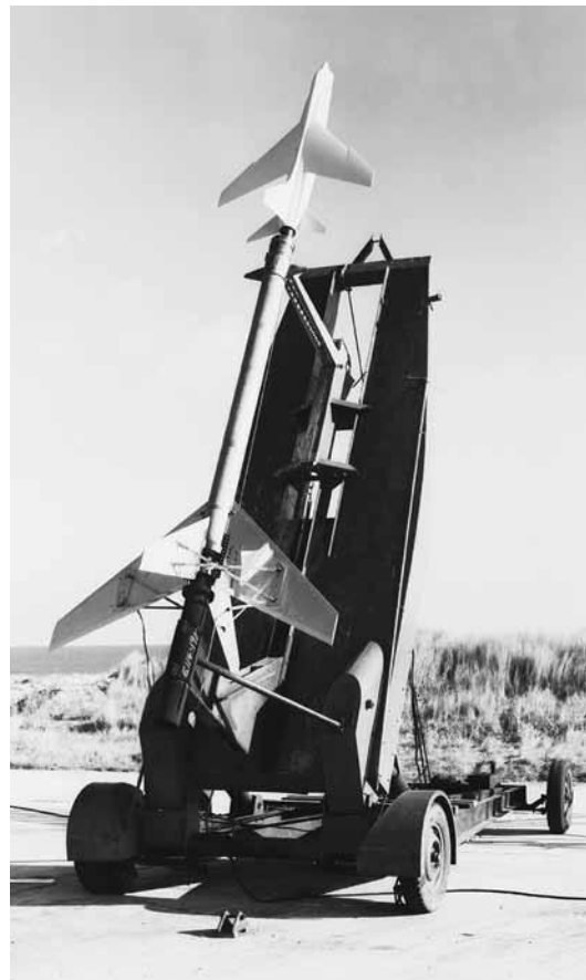
Model of the Chance Vought F8U used by the Langley Pilotless Aircraft Research Division at its Wallops flight station in rocket-launched model tests to determine supersonic dynamic stability.
