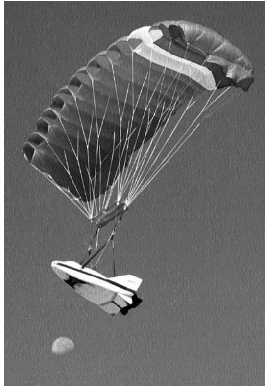
A 0.80-scale model of the X-38 Crew Return Vehicle in controlled glide using a parafoil for landing.
