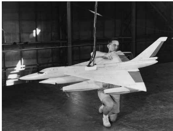
Free-flight model of the Convair XB-58 bomber is prepared for dynamic stability and control evaluations in the Full-Scale Tunnel.
