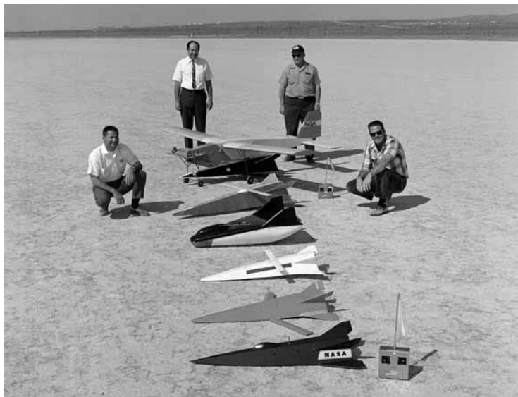
Photograph of Dryden free-flight research models of reentry lifting bodies. Dale Reed, second from left, and his test team pose with the mother ship and models of the M2-F2 and the Hyper III configurations.
