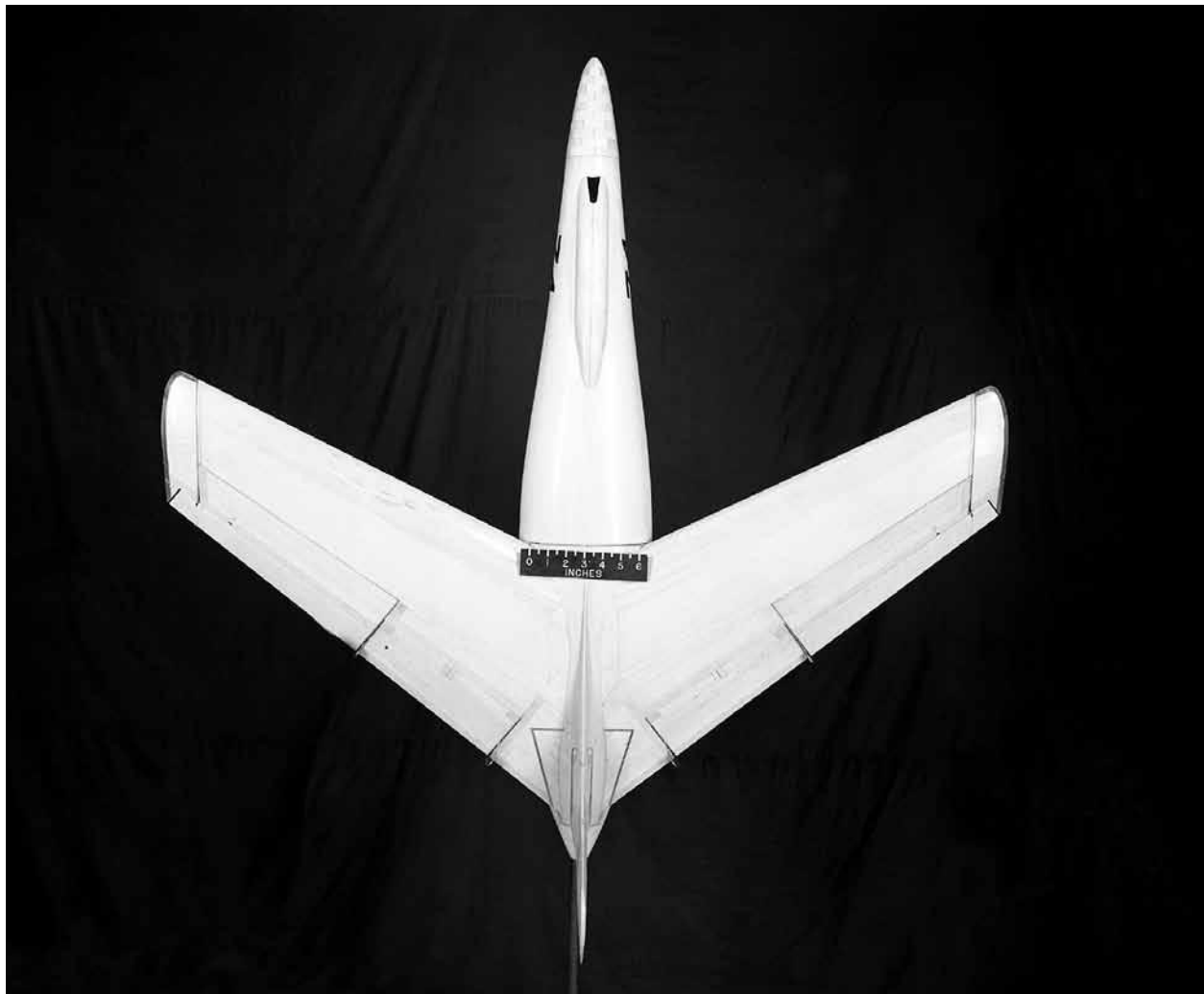
Top view of the model of the Convair XB-53 forward-swept wing bomber tested in the Free-Flight Tunnel. The aircraft incorporated a 30-degree swept-forward wing and was tested in several facilities at Langley but did not enter production.
