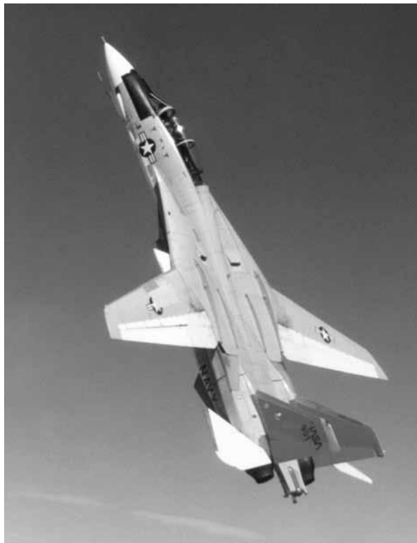
The F-14 aircraft was used for the joint NASA–Grumman–Navy assessment of automatic control concepts for enhanced high-angle-of-attack behavior. NASA's use of free-flight models in the Full-Scale Tunnel, the Spin Tunnel, and the drop-model operation provided substantive data for the planning of the program.
