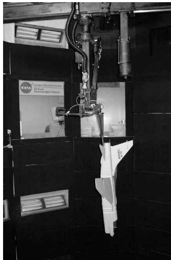
The latest rotary-balance test apparatus in the Langley Spin Tunnel permits roll oscillations to be superimposed on the steady spinning motion.
