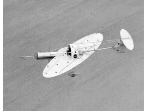
Oblique wing research vehicle flown in cooperative study between Ames and Dryden researchers during the 1970s to explore the aerodynamics and flying characteristics of the configuration. The vehicle was designed to permit its left wing panel to be swept forward 45 degrees. Three research flights in 1976 provided data for the design of the piloted AD-1 research aircraft.
