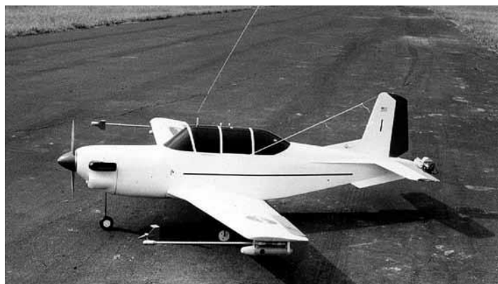
The Beech Aircraft Corporation conducted spin tests with this radio-controlled model of the YT-34 military trainer in 1976. Note the wingtip booms with flow vanes, the tail-mounted spin recovery parachute, and the wingtip rocket pods used for pro-spin inputs.
