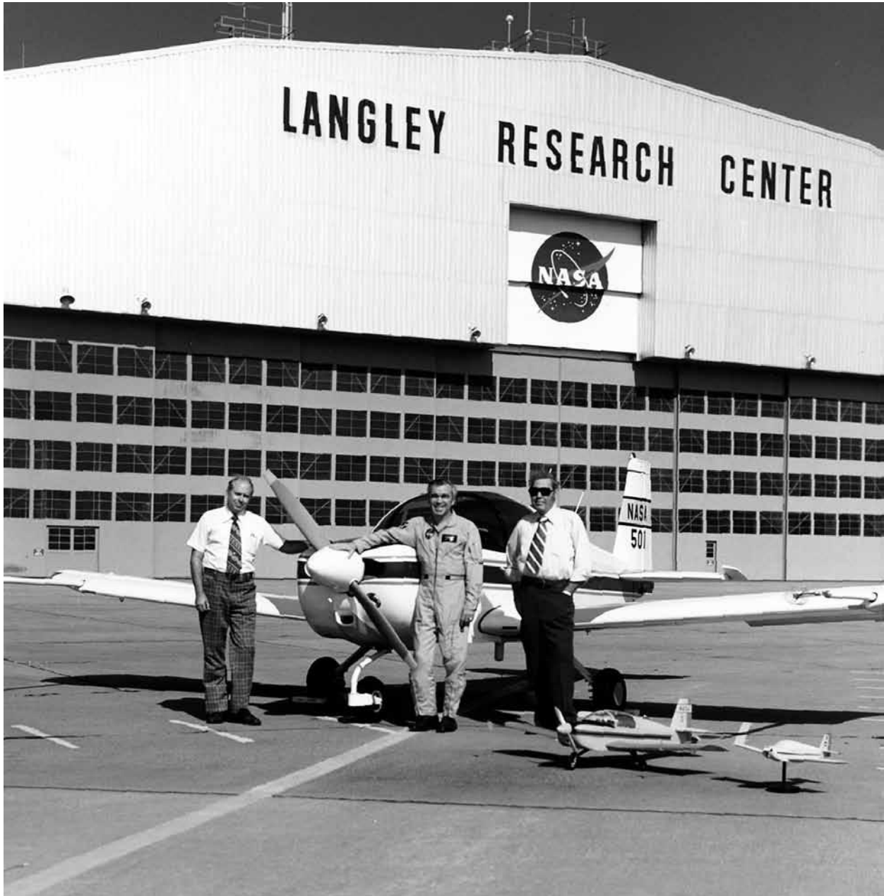
Predictions obtained from dynamic model tests are routinely correlated with results from aircraft flight-testing. In a classic NASA study of spinning characteristics of general-aviation configurations, tests were conducted with, right to left: a spin tunnel model, a radio-controlled model, and the full-scale aircraft. Langley test pilot Jim Patton, center, and researchers Jim Bowman, left, and Todd Burk pose with the test articles.
