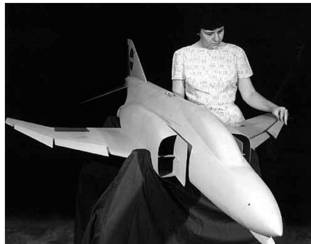
Free-flight tests of this model of the F-4 Phantom II in 1970 provided data for analysis of the wing rock and directional divergence exhibited by the configuration at high angles of attack. The test program also included demonstrations of the benefits of two-position fixed leading-edge slats, which were incorporated in later versions of the airplane.
