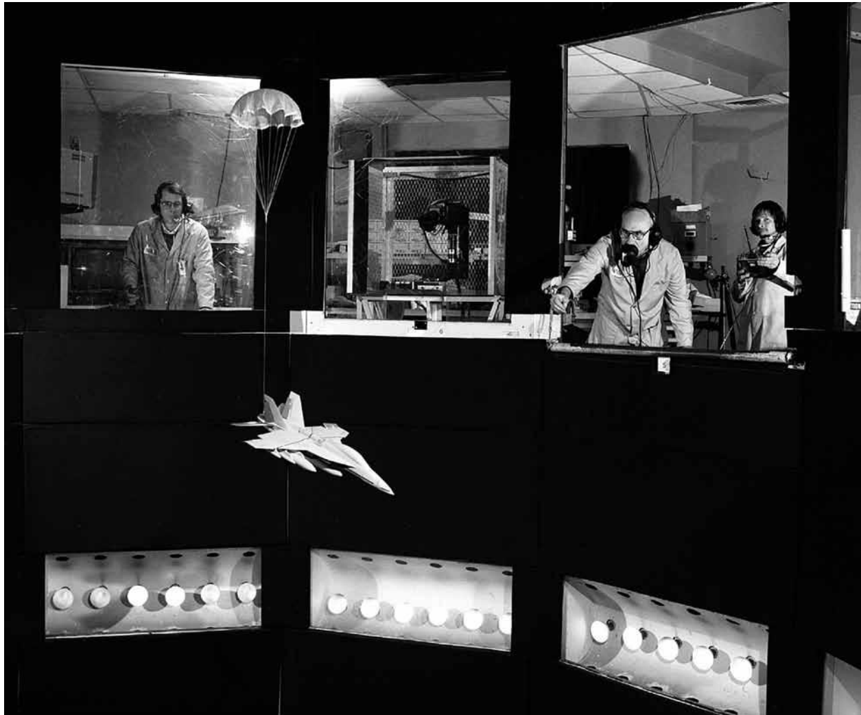
Free-spinning tests are used to determine the effects of external stores on the spin and recovery characteristics of military aircraft. The photograph shows a model of the F/A-18F during store effects testing after the deployment of the emergency spin recovery parachute.
