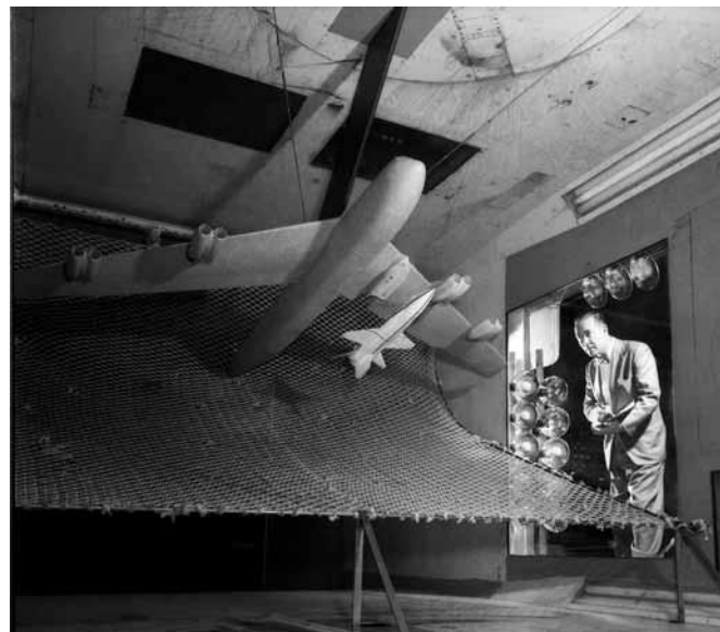
Free-flight drop model of the X-15 research aircraft undergoes separation testing beneath a B-52 model in the Langley 300 mph Low-Speed 7- by 10-Foot Tunnel. The model was mounted under the left wing of the bomber for these tests for visibility.
