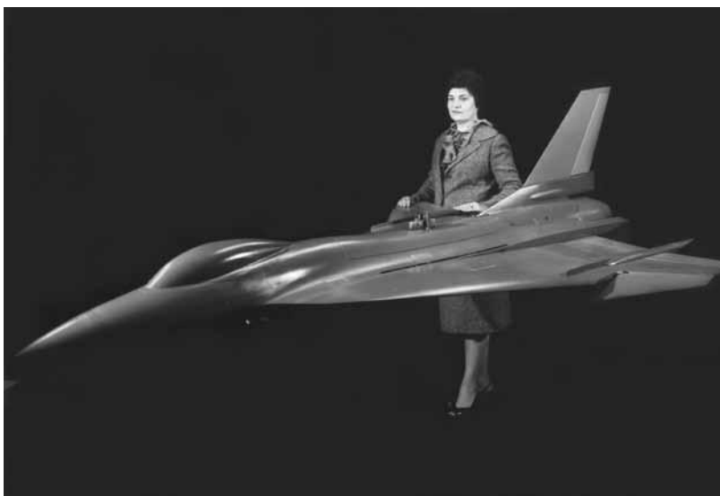
Configuration modifications to the General Dynamics F-16XL aircraft included geometric shaping of the wing apex area and wing fences. These modifications were derived from highly successful free-flight and force tests conducted in the Full-Scale Tunnel in 1981.
