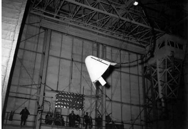
Photograph of the Ames M1 reentry concept in free-flight during evaluations in 1959. The model was powered by compressed air through a nozzle at the rear of the model and used two pairs of control surfaces.
