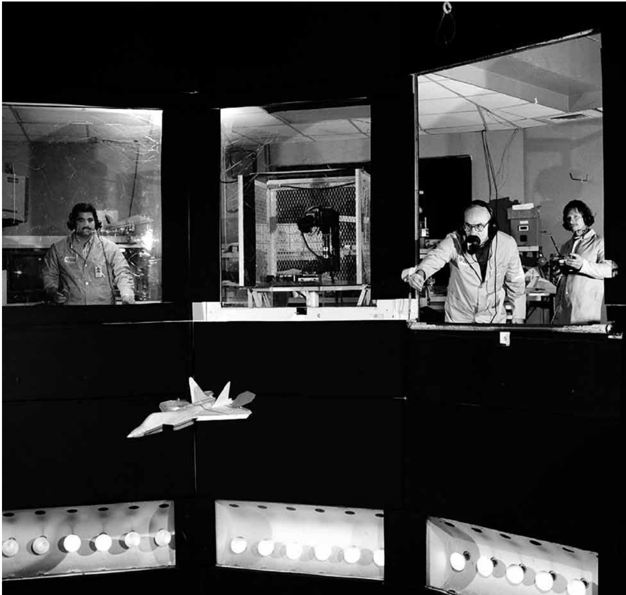
Spin tunnel test of a dynamically scaled model of the F-22 fighter. The model has been hand-launched with a spinning motion into a vertical airstream controlled by the tunnel operator on the left. The spin recovery controls will be applied using the hobbyist-type, radio-controlled transmitter held by the technician on the right.
