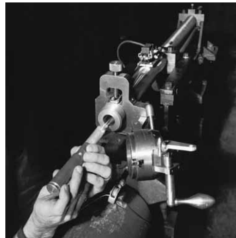
Model, sabot, and cartridge assembly prepared for firing in the Ames Supersonic Free-Flight Tunnel.
