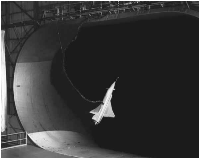
NASA activities in support of the international X-31 research aircraft program included free-flight model testing in the Full-Scale Tunnel.
