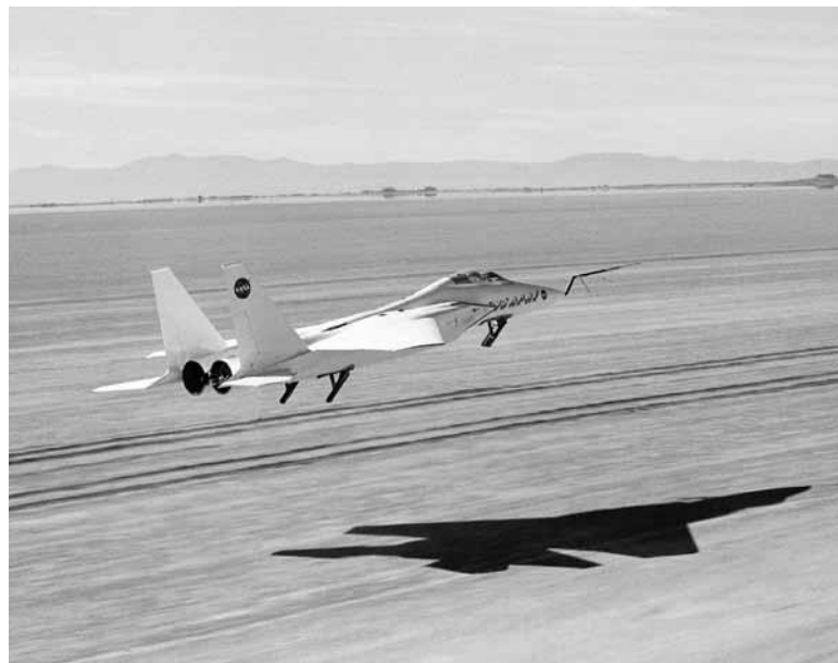
The 0.38-scale F-15 RPRV lands on the lakebed at NASA Dryden after a successful flight.
