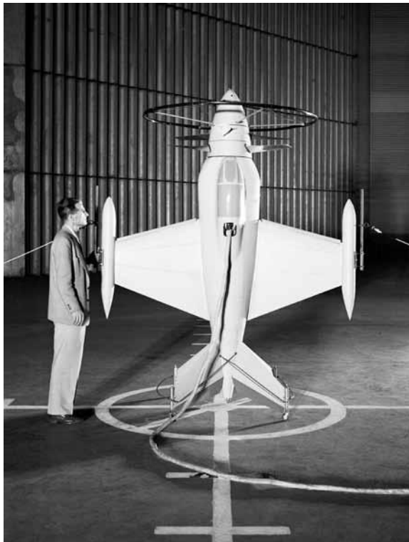
A one-quarter-scale free-flight model of the Lockheed XFV-1 VTOL tail sitter airplane being prepared for hovering tests in the return passage of the Ames 40- by 80-Foot Tunnel. The test of the 250-pound model was the only subscale free-flight test conducted in the facility. Note the propeller-guard assembly for the counter-rotating propellers, the flight cable providing power and control inputs, and the wingtip-mounted stabilization lines.
