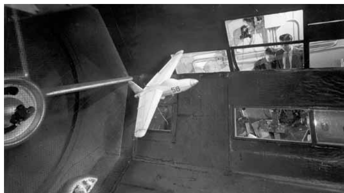
Free-flight test of a swept-forward wing, tailless fighter design known as the Air Material Command MCD-387-A in the Langley 12-Foot Free-Flight Tunnel. The evaluation pilot is visible in the enclosure at the lower left, while the two tunnel operators controlling airspeed and tunnel tilt angle are at the right.
