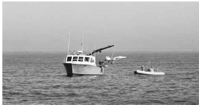
Water retrieval of the F/A-18E drop model from the Atlantic Ocean after a drop test. The descent by parachute into the water posed special problems for model designers, instrumentation specialists, and the operational crew.
