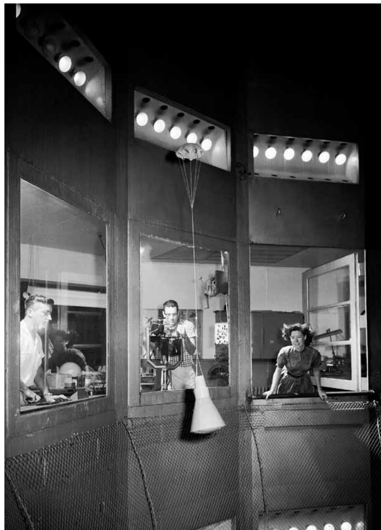
Photograph of the free-flight Mercury capsule in vertical descent in the Spin Tunnel with drogue parachute deployed. Tests to determine the dynamic stability characteristics of capsules have continued to this day.
