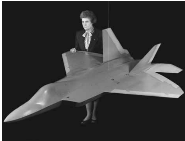
Free-flight model tests of the YF-22 prototype in 1989 had demonstrated outstanding stability and control characteristics at high angles of attack, which were subsequently verified in the competitive evaluation flight tests of the aircraft. The follow-on F-22 program did not request a NASA free-flight study, but a conventional force-test program was conducted in the Full-Scale Tunnel in 1992 with a model similar to those used in free-flight testing.
