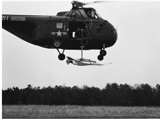
The launch helicopter with the drop model of the F4H-1 in an extended position on its launch rig prepares to climb to altitude at West Point in 1960. The primary objective of the tests was to establish the relative ease with which the model would enter a flat spin.
