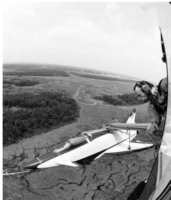
A fish-eye camera lens captures a scene of a drop model of the X-31 research aircraft being prepared for a drop as part of poststall and spin resistance studies.
