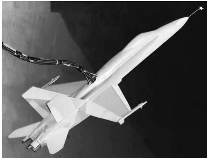
The free-flight model of the F-18 flies at high angles of attack with thrust-vectoring vanes and deflectable nose strakes. Both concepts were subjects of intense flight-test investigations at Dryden.
