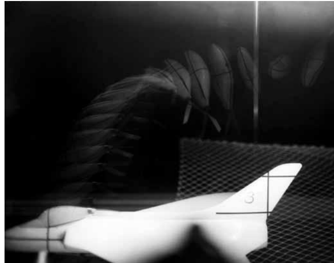
Time sequence of a canopy ejection test in the Langley 300 mph 7- by 10-Foot Wind Tunnel. The staff of the facility conducted extensive separation studies of aircraft stores and components using a net to catch components released from models under test.
