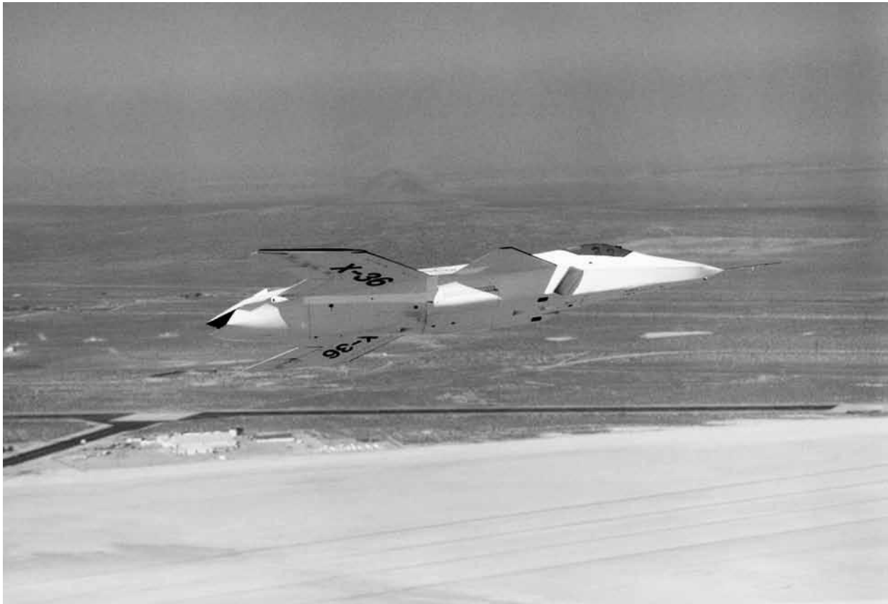
The X-36 tailless advanced fighter flight demonstrator in flight at NASA Dryden. The radical configuration conducted a successful flight investigation in one of the more remarkable remotely piloted vehicle programs at Dryden.
