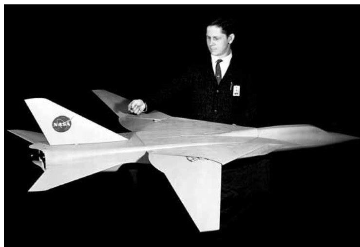
Free-flight model of outboard pivot variable-sweep model used in research studies at Langley. Conceived by researchers at the Langley 7- by 10-Foot High-Speed Tunnel, this configuration was tested across the speed range, including low-speed flight tests in the Full-Scale Tunnel.
