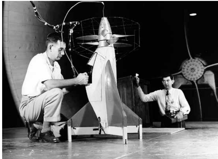
Flight studies of the stability and control characteristics of the Convair XFY-1 were conducted in the Langley Full-Scale Tunnel. Note the flexible flight cable, the one-eighth-inch steel safety cable, and the wire propeller guard.
