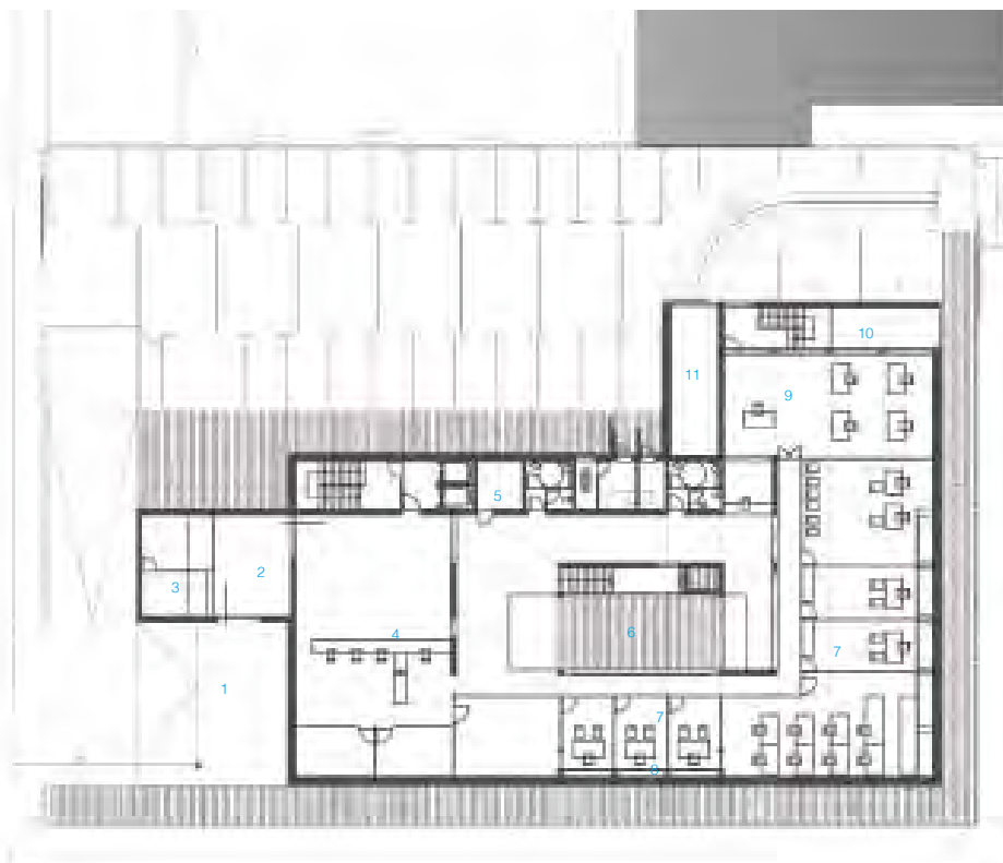
Ground floor plan 1. Entry hall 2. Principal entry 3. Security zone 4. Customer service & reception 5. Service area & installations 6. Central hollow 7. Engineer offices 8. Illumination void 9. Management 10. Emergency exit 11. Garage entry
