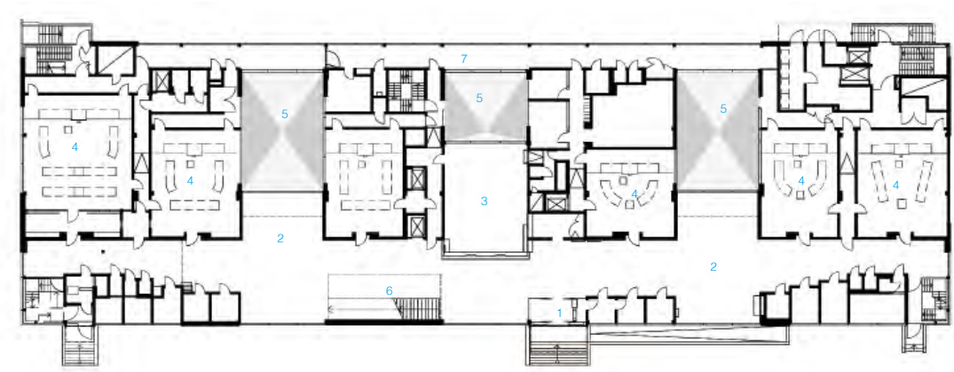
Ground floor plan (Floor plan court rooms) 1. Public entrance 2. Foyer area 3. Reception 4. Court room 5. Atrium 6. Stairway to upper floor 7. Protected area
