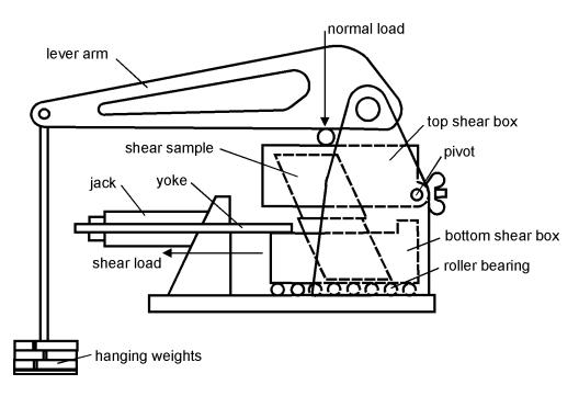
Figure 2: Diagrammatic section through shear machine used by Hencher and Richards (1982).
