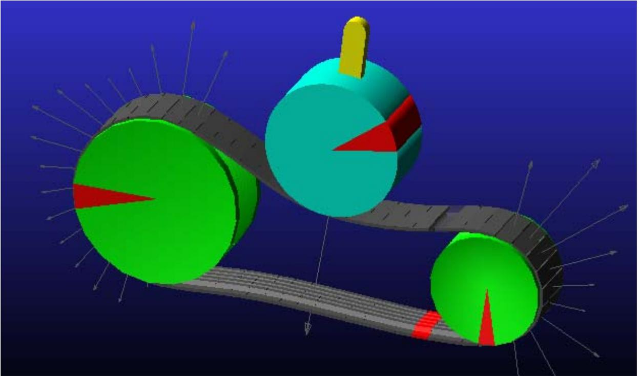
Figure 1 Poly-V Grooved Belt System
