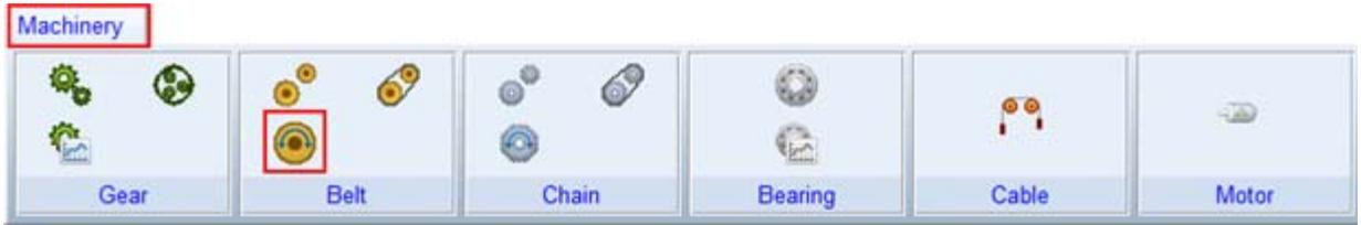
23. The **Actuate Belt** wizard is launched. In the Pulley Set **Name** field enter the name of the pulley set you just created (right-mouse-click in the field and use **Pick** or **Guesses** to quickly select). In the Actuator Pulley field enter the name of the driver pulley (right-mouse-click in the field and use **Pick** or **Guesses** to quickly select). Then click **Next**.
