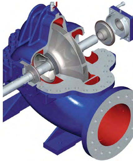
(b) Cut-away diagram of single stage double suction split case centrifugal pump. (Courtesy of Clyde Pumps Ltd. incorporating Weir Pumps, Glasgow)
