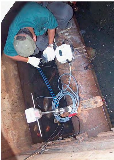
(c) Electromagnetic flowmeter insertion probe with pressure transducer and data logger. (Black & Veatch)
