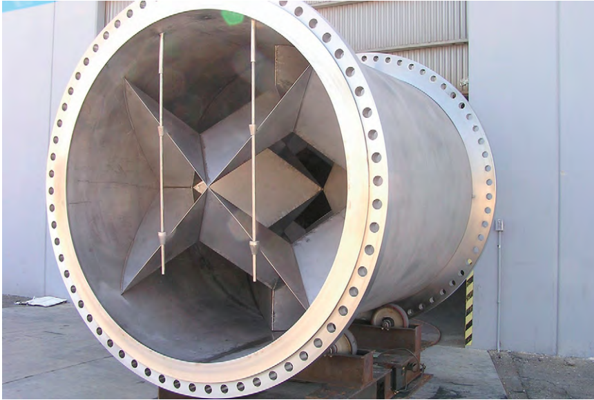
(a) 2.8 m diameter static mixer for pH control using 98% sulphuric acid. (Manufacturer: Statiflo, UK)
