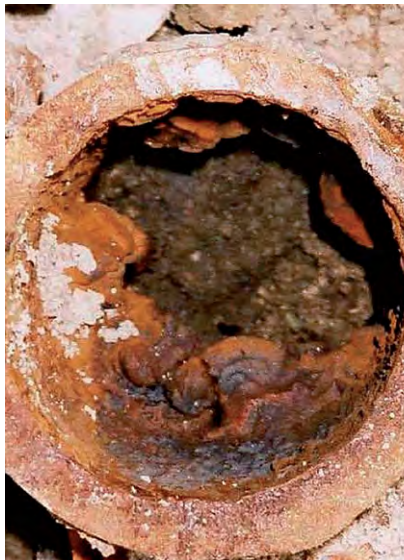
(a) Heavily tuberculated cast iron pipe. What is the value of pipe roughness?
