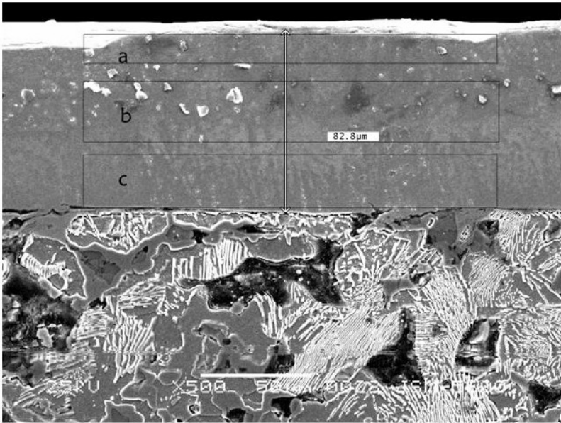
Figure 5: Cross section of the biomimetic gradient n-Al 2 O 3 /Ni-Co nanocomposite coating on the surface of metal metallurgy parts.
