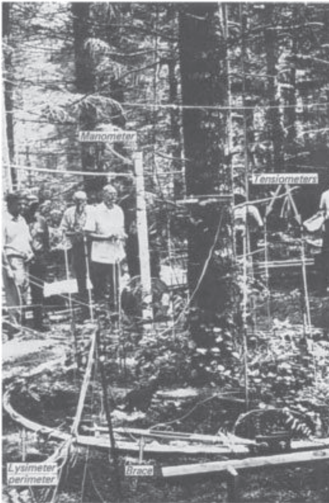
(b) A giant 'floating' lysimeter containing a mature Douglas fir tree at Cedar River, Washington. The observer (centre left) is reading the manometer which monitors mass changes by the soil-tree monolith. Tensiometers are installed both inside and outside the lysimeter to ensure that similarity of moisture content is maintained. The brace in the foreground prevents rotation, and the tree is lightly 'guyed' to surrounding trees to prevent it falling over in high winds.
