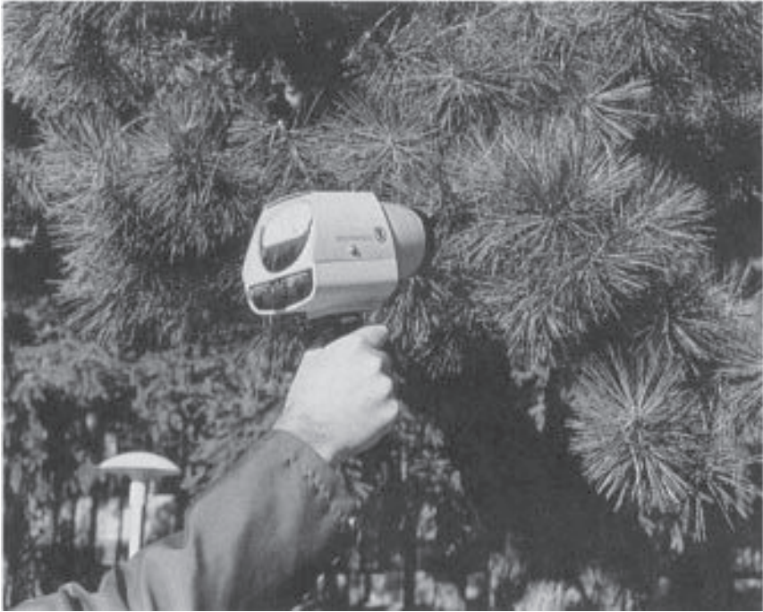
Figure A2.2 Hand-held infra-red radiation thermometer (Barnes PRT-10) for surface radiation temperatures.
