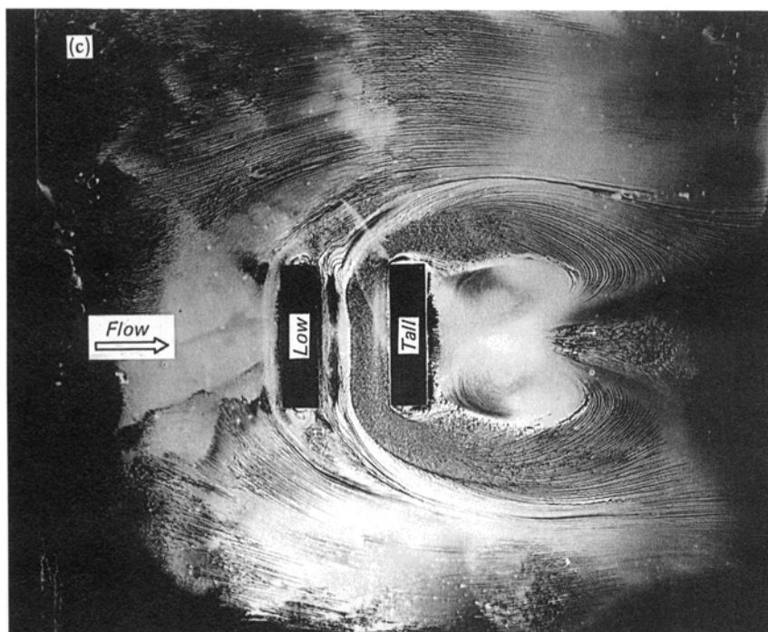
Figure 8.3 Flow around a tall building with lower buildings upwind, (a) Flow over the windward face visualized by the deflection of smoke jets emanating from a wind tunnel model, (b) Illustration of the three main regions of increased wind speed at pedestrian level (stippled), see the text for the meaning of the numbers. (c) Plan view of flow at ground level around a tall building (rectangle on the right) with a low building upwind. Horseshoe pattern is made visible by surface film of pigmented oil around wind tunnel models (photographs after Penwarden and Wise, 1975, Crown copyright by permission of the Director, Building Research Establishment).
