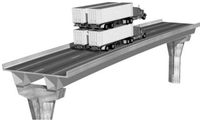
FIGURE 5.18 Loading proposed by NCHRP 406 for evaluation of system redundancy and reserve capacity (multiples of HS-20 pairs).
