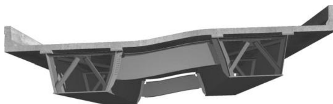
FIGURE 5.19 Deformed shape, showing load paths and components included in redundancy and reserve capacity assessment.
