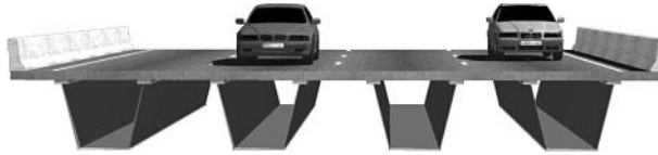
FIGURE 5.4 Typical multi-box girder superstructure (four lane bridge).
