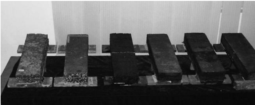
FIGURE 16.42 Six wearing surface fatigue test rectangular specimens. (Courtesy of Charles Seim.)
