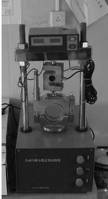
FIGURE 16.43 Marshall testing machine. (Courtesy of Charles Seim.)
