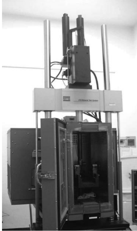
FIGURE 16.41 Wearing surface fatigue testing machine with environmental chamber. (Courtesy of Charles Seim.)
