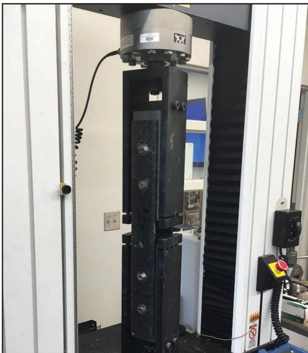
Figure 6: Fixture With Test Specimen Mounted To Tensile Tester
