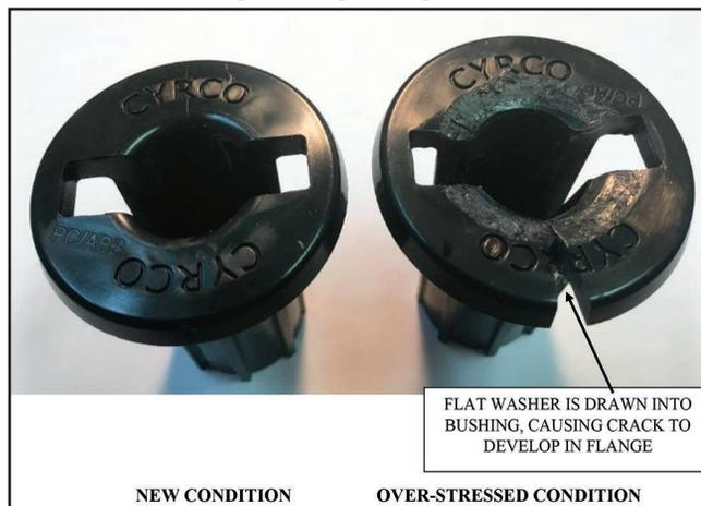
Figure 14a Compression Over-Stress Test 84 N-M (62 Ft-Lbs) Torque
