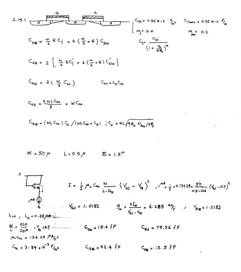
$$f_{T} = \frac{9_{m}}{2\pi (C_{q0} + C_{qs})} = 10.6 \text{ GH}_{3}^{2}$$
