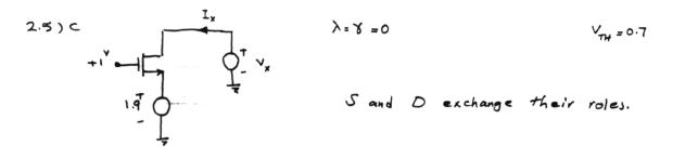
$V_{GS} = 1 - V_{X}$   $V_{DS} = 1 - 9 - V_{X}$   $V_{OD} = V_{GS} - V_{TW} = 0.3 - V_{X}$
