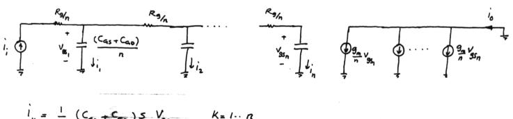
$$(\bigstar) \quad l_{i} = l_{i} + l_{2} + \dots + l_{n} = \frac{l}{n} \left( C_{q_{s}} + C_{q_{0}} \right) S \left( V_{g_{s}} + V_{g_{s_{2}}} + \dots + V_{g_{s_{n}}} \right)$$
