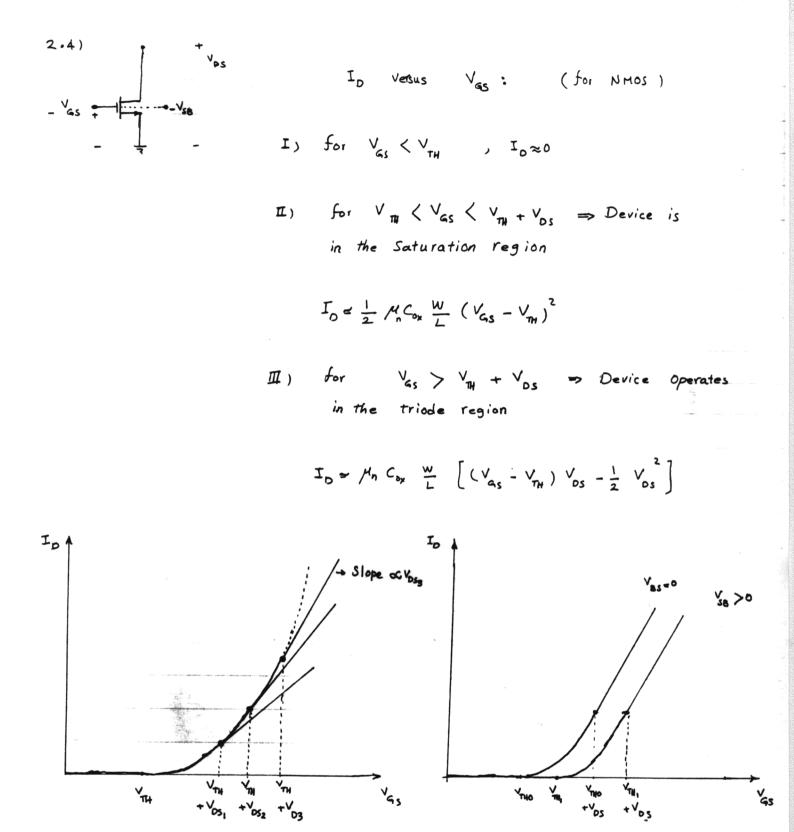
Changing  $V_{so}$  just shifts the curve to the right for  $V_{so} > 0$  or to the left for  $V_{so} < 0$
