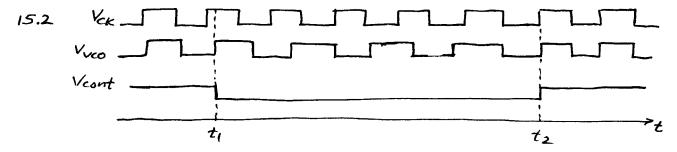
The difference between the two frequencies is integrated between t, and to accumulate a difference of \$:
