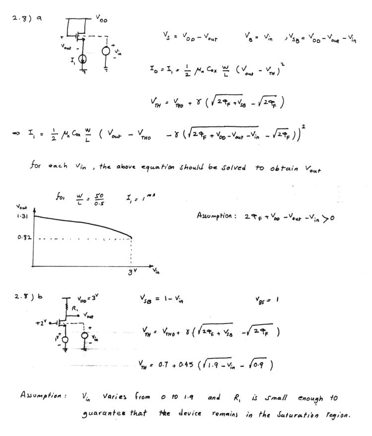
$V_{aut} = 3 - R_1 \cdot \frac{1}{2} \mu_a G_{0x} \frac{W}{L} (0.3 - 0.45 (\sqrt{1.9 - V_{in}} - \sqrt{0.9}))^2$
