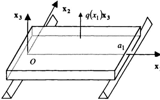
Figure 10.1. Plate under cylindrical flexure
