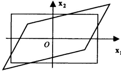
Figure 2.8. Strains when  $S_{16} = S_{26} = S_{36} = 0$
