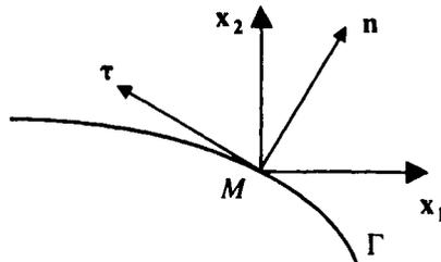
Figure 18.1. Local axes attached to an edge
