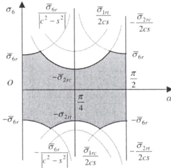
Figure 4.5. Maximum stress criterion for pure shear
