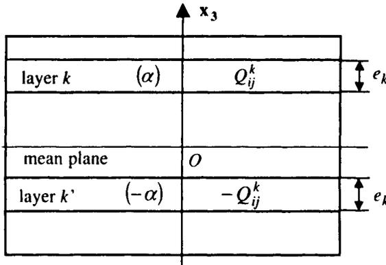
Figure 5.4. Balanced laminate
