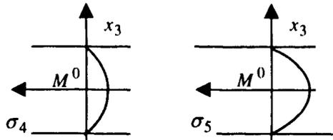
Figure 6.8. Transverse shear stress variations
