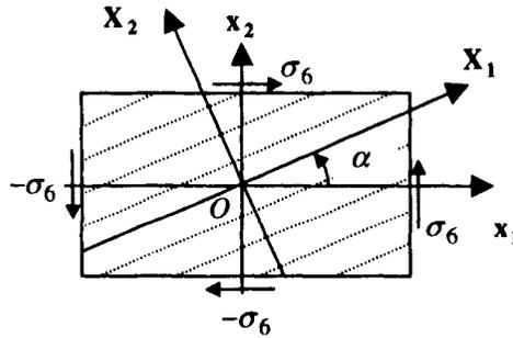
Figure 4.4. Off-axis shear
