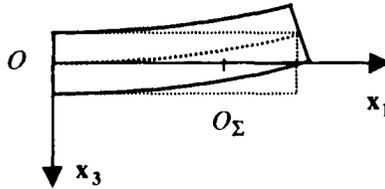
Figure 13.1. Beam element deformed in the plane  $(O|x_1, x_3)$
