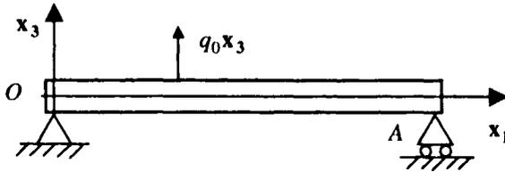
Figure 14.1. Beam subjected to a sinusoidal load
