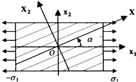
Figure 4.1. Off-axis tension
