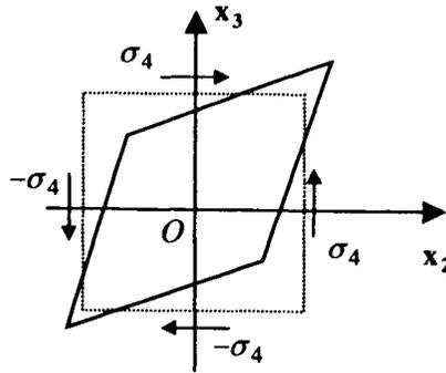
Figure 1.3. Simple shear
