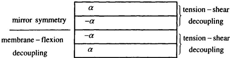
**Figure 5.5. Balanced symmetrical laminate**
