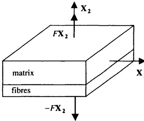
Figure 3.2. *Transverse tension*
