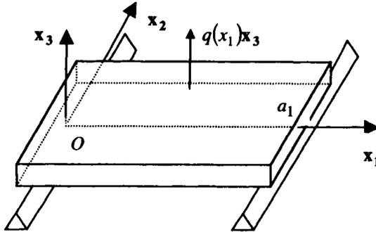
Figure 11.1. Plate in cylindrical flexure
