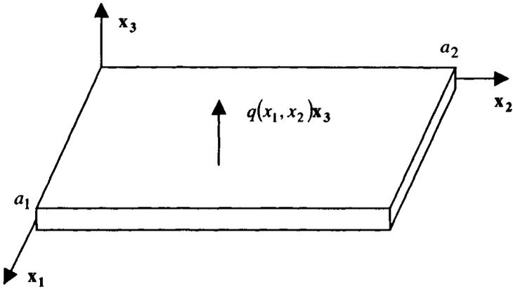
Figure 9.4. Asymmetrically balanced plate in flexure
