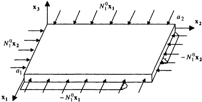
Figure 6.15. Identical compression loads in two directions
