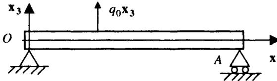
Figure 13.3. Beam subjected to a sinusoidal load
