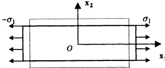
Figure 1.2. Simple tension
