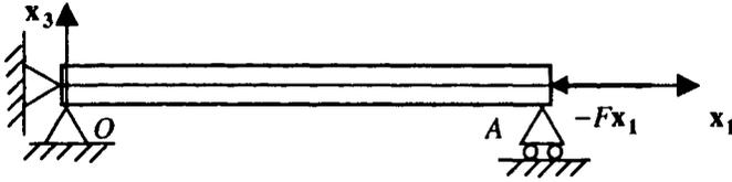
Figure 14.2. Beam buckling
