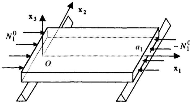
Figure 10.2. Plate subjected to buckling
