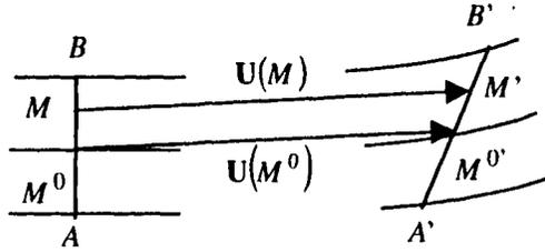
Figure 15.2. Displacement field
