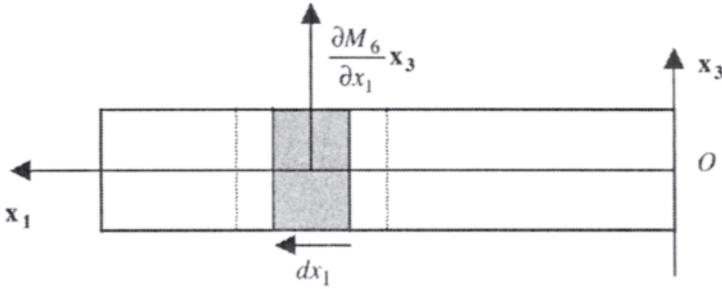
**Figure 5.15.** Equivalent linear force density acting on two contiguous edge half elements  $x_2 = a_2$
