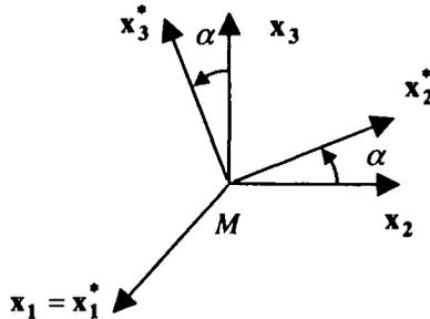
Figure 1.4. Isotropic plane
