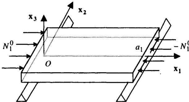
Figure 11.2. Plate in buckling situation
