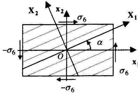
Figure 2.6. Shear in off-axis directions
