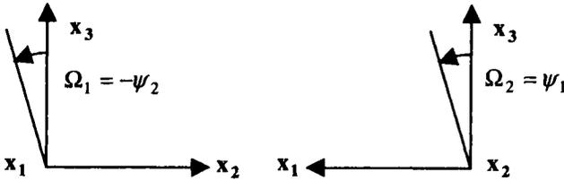
Figure 15.3. Infinitesimal rotations
