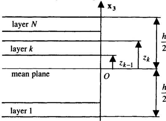
Figure 5.2. Distribution of layers in the composite
