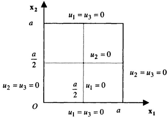
Figure 6.3. Zero displacement
