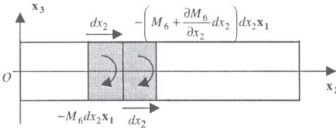
Figure 5.10. Couples acting on two elements next to the edge  $x_1 = a_1$
