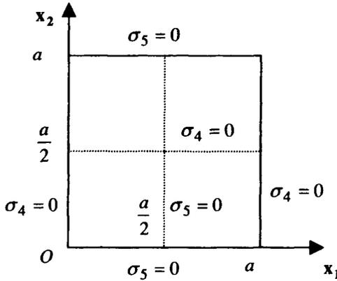
Figure 6.9. Zero transverse shear stresses
