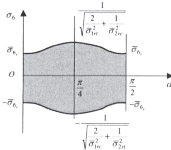
Figure 4.6. Tsai-Hill criterion for pure shear
