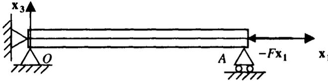
Figure 13.4. Beam buckling
