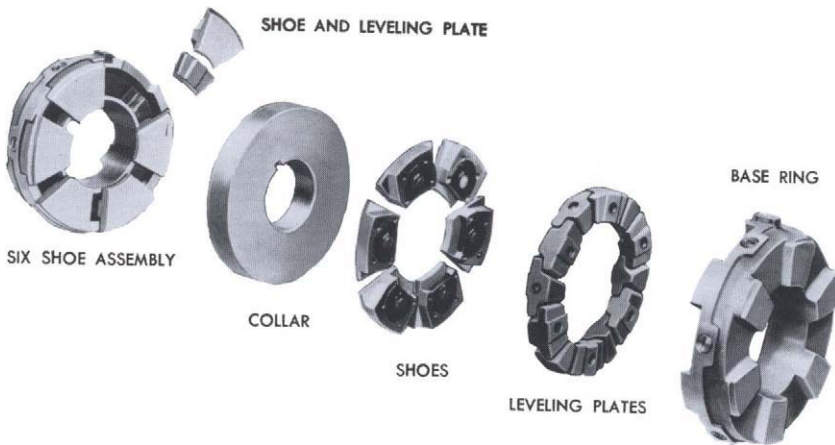
Figure 9.35 Small Kingsbury six-shoe two-direction thrust bearing. Left-hand group assembled, except for one shoe and 'upper' leveling plate. Right-hand group disassembled. (Courtesy of Kingsbury, Inc)
