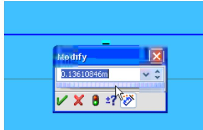
You can change the length of the line by using the slider bar or you can simply enter in 4 m in the box shown. Enter the value 4 then click the green check. Since the box is way too big, press “f” on the keyboard to fit. Then drag down the dimension so that you can see it after hitting escape.
