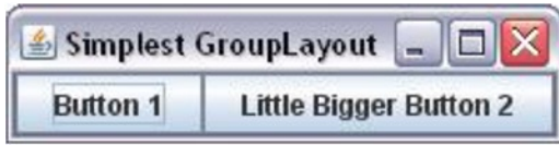
Figure 1-51. The simplest GroupLayout in which two buttons are placed side by side
