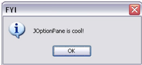
Figure 2-31. An information message dialog using the JOptionPane.showMessageDialog() method
