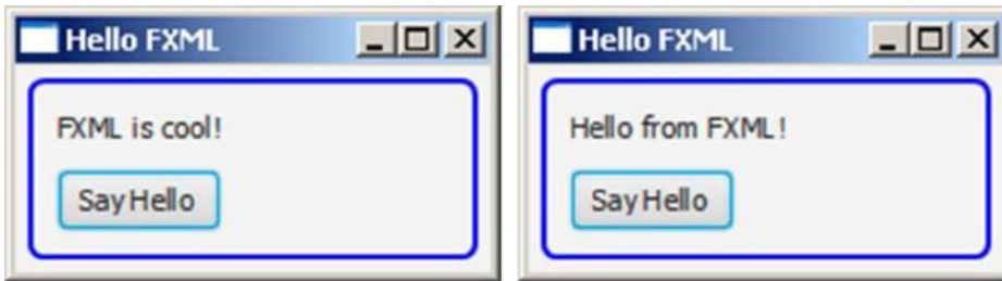
Figure 9-26. Two instances of a window whose scene graph is created using FXML
