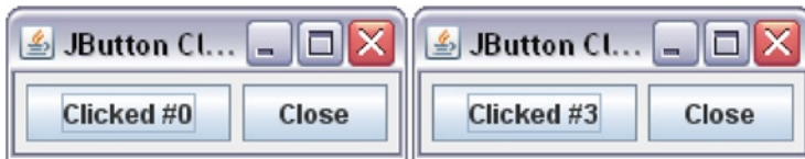
Figure 1-57. A JFrame when it is displayed and after the counter JButton is clicked three times
