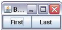
Figure 1-21. A horizontal box with two buttons and a horizontal glue between them
