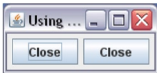
Figure 2-4. Two Close buttons created using the same Action object
