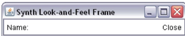
Figure 3-6. A JFrame with a Synth L&F where the Synth XML file does not define any styles
