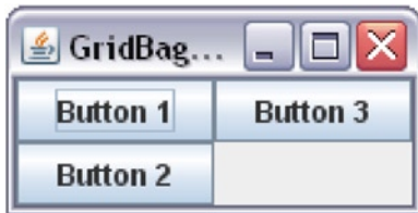
Figure 1-28. Specifying gridx and Setting gridy to RELATIVE
