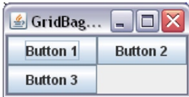
Figure 1-29. Specifying gridy and setting gridx to RELATIVE in a GridBagLayout
