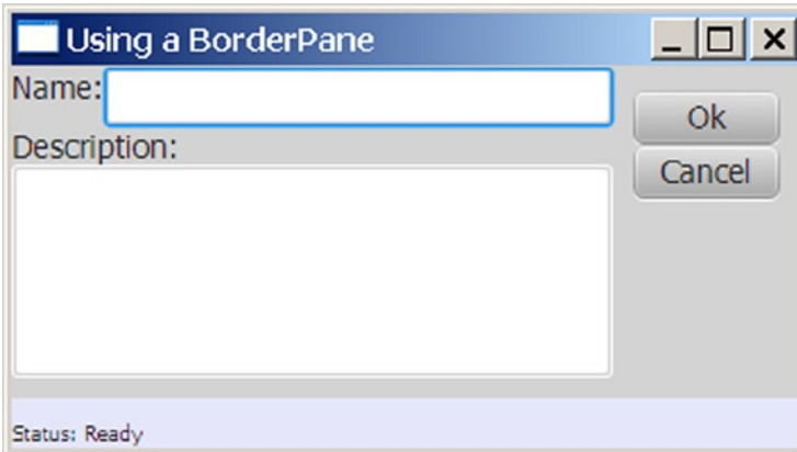
Figure 9-12. A BorderPane using some controls in its top, right, bottom, and center regions
