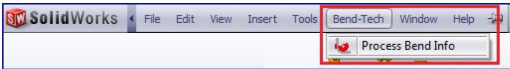
Once Process Bend Info has been clicked, the Send To Bend-Tech panel will be opened on the left side of the window. Depending on what kind of feature you selected (3D Sketch or Sweep), it will be shown in either the Feature Selection or Sketch Selection box. Ensure that the listed feature is correct, click on it to select it, then click the green check button.
