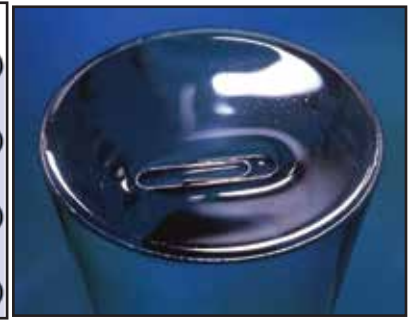
Figure 4 : Visible effect of surface tension
