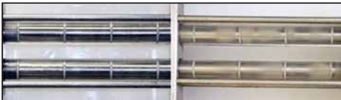
Figure 8: Appearance of test heat exchanger surfaces before and after scale development “crash point”
