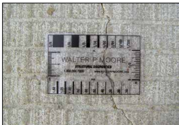
Figure 8: Crack Comparator for Measuring Crack Widths
