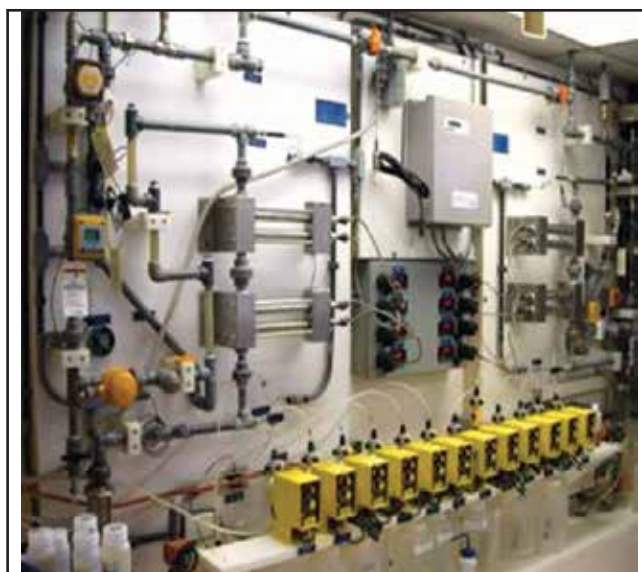
Figure 6: Pilot cooling tower heat exchanger and instrumentation.
