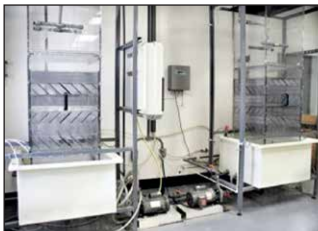
Figure 7: Pilot cooling towers
