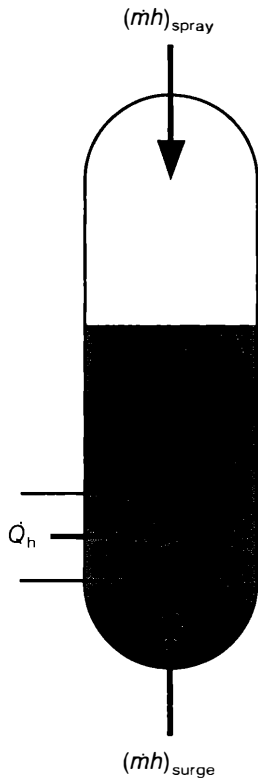
Figure 7-10 Externally supplied mass flow rate, enthalpy, and heat to the one-region pressurizer.
