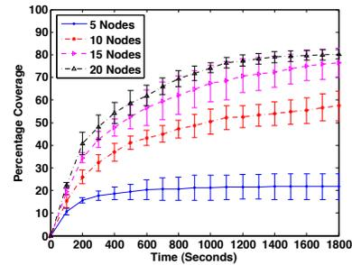
Figure 8: The figure shows the percentage 3-D coverage for SensorFly nodes in the 3 room simulation arena over a duration of 1800 seconds. The error bars show the standard deviation of coverage obtained.
