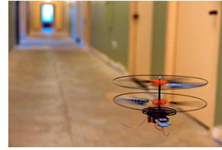
Figure 4: The 29g SensorFly node hovering in a hallway.
