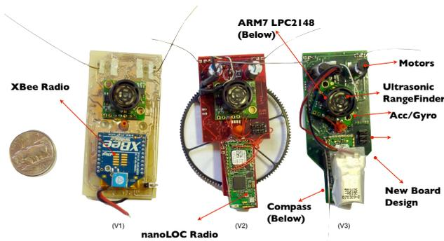
Figure 1: Three generations of SensorFly node design.
