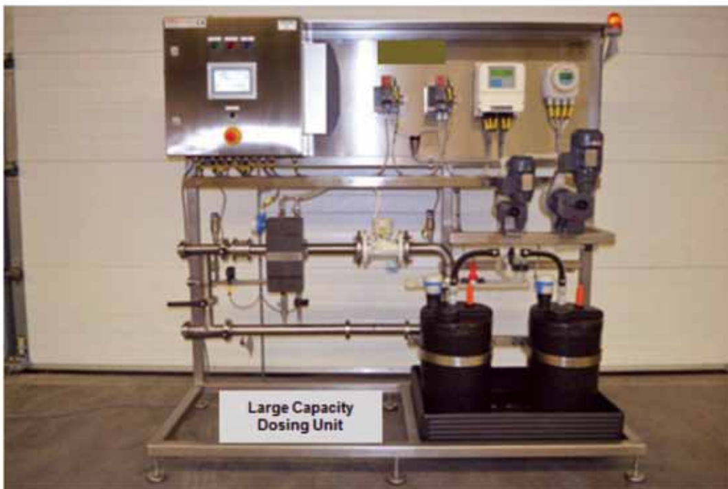
Figure 6. Design and Arrangement of Dosing Equipment for Chlorine Dioxide Prepared From Powdered Precursors for Various capacity Applications.
