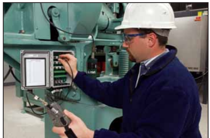
Figure 10: Data collection using a walk around data collector, permanently mounted accelerometers, and a junction box.
