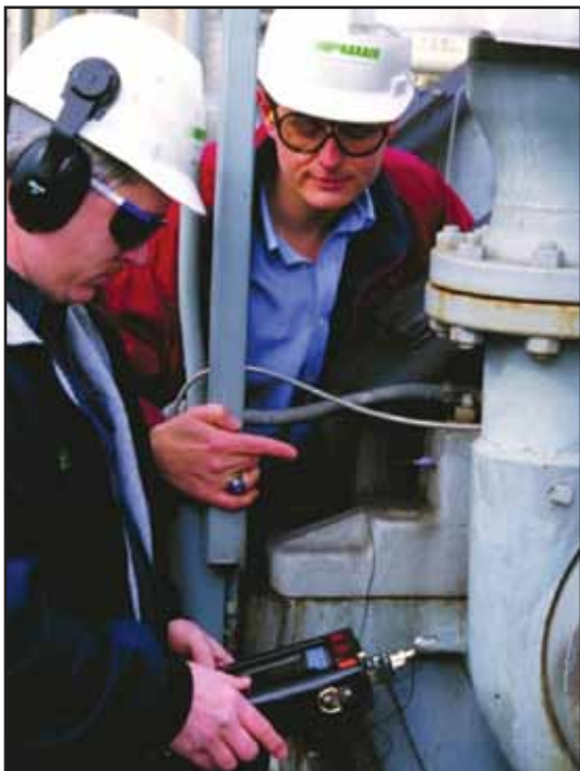
Figure 8: Data collection using a walk around data collector with a magnetically mounted high frequency accelerometer (photo courtesy of Praxair)
