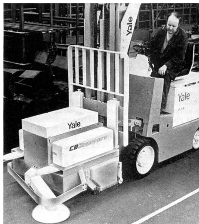
Figure 6.28 Useful sweeper attachment to a forklift truck.
