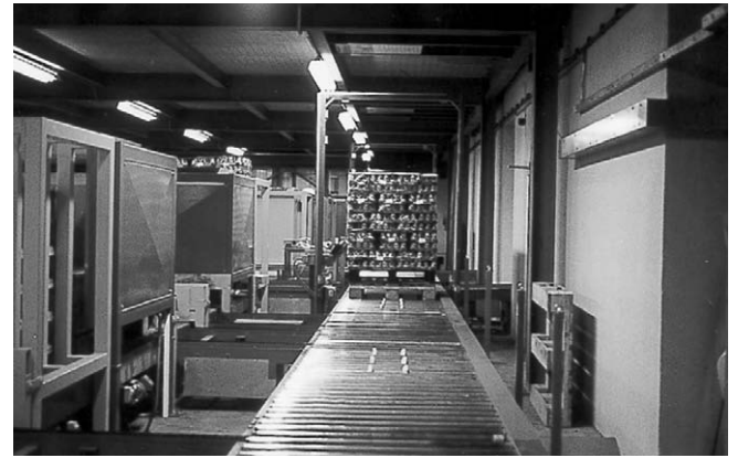
Figure 5.13 Automated pallet in-feed; pallet passing through dimension check gauge.
