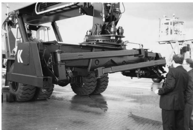
Figure 3.32 Adjustable spreader beam.
