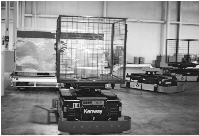
Figure 5.51 Two types of AGV in use in a warehouse. In the foreground AGV with direct load, behind articulated AGV towing a trailer.
