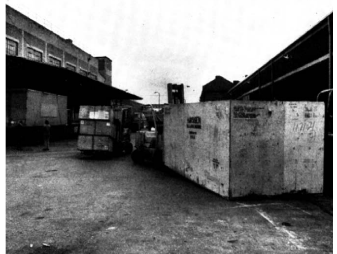
Figure 2.11(b) With two forklifts in operation, the throughway is frequently impassable to heavy vehicles.
