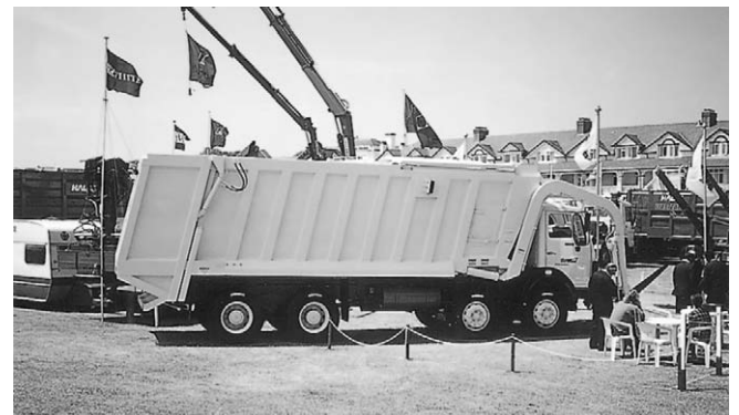
Figure 2.50 Front-loading bin collection vehicle: the front lift-arms empty the bin over the cab.
