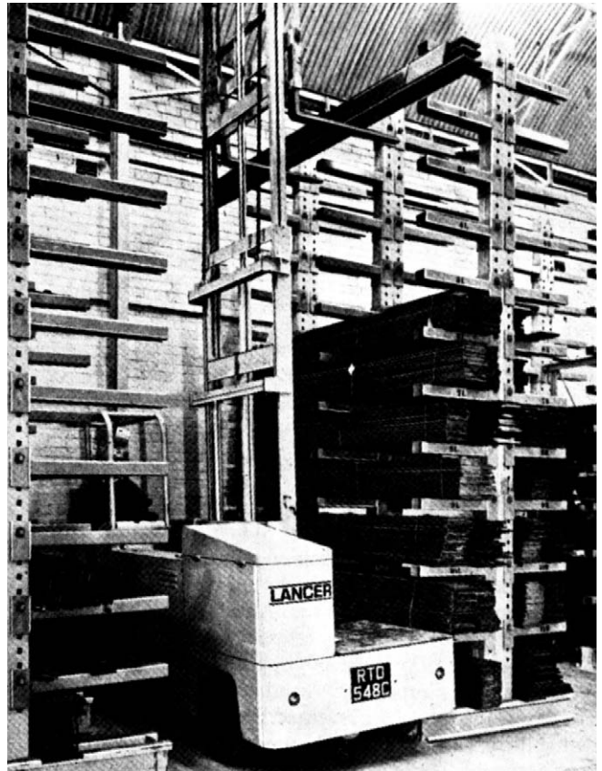
Figure 4.102 Fir tree racking is suitable for long narrow objects.
