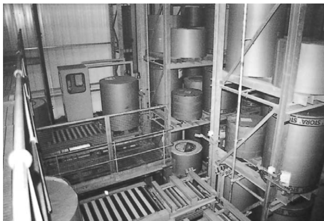
Figure 7.11 Reels of newsprint stored on end rather than edge to avoid flat spots. Apart from handling by heavy-duty forklift trucks with clamps to stack reels up to 9 m high, the automated storage process is similar.
