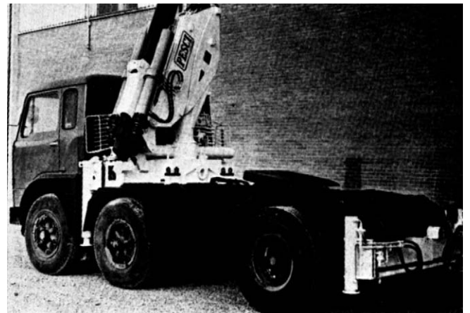
Figure 3.34 Artic tractor with self-loading crane.
