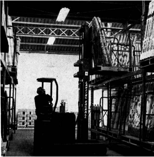
Figure 4.14 Typical reach truck retracting its mast within its wheelbase.
