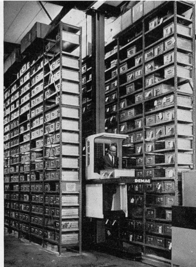
Figure 4.158 Fixed-path order picker in 950 mm wide aisle used here with tote boxes.
