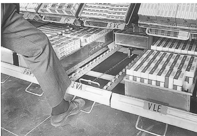
Figure 4.105 Foot-operated brake release on manual carton dispenser.
