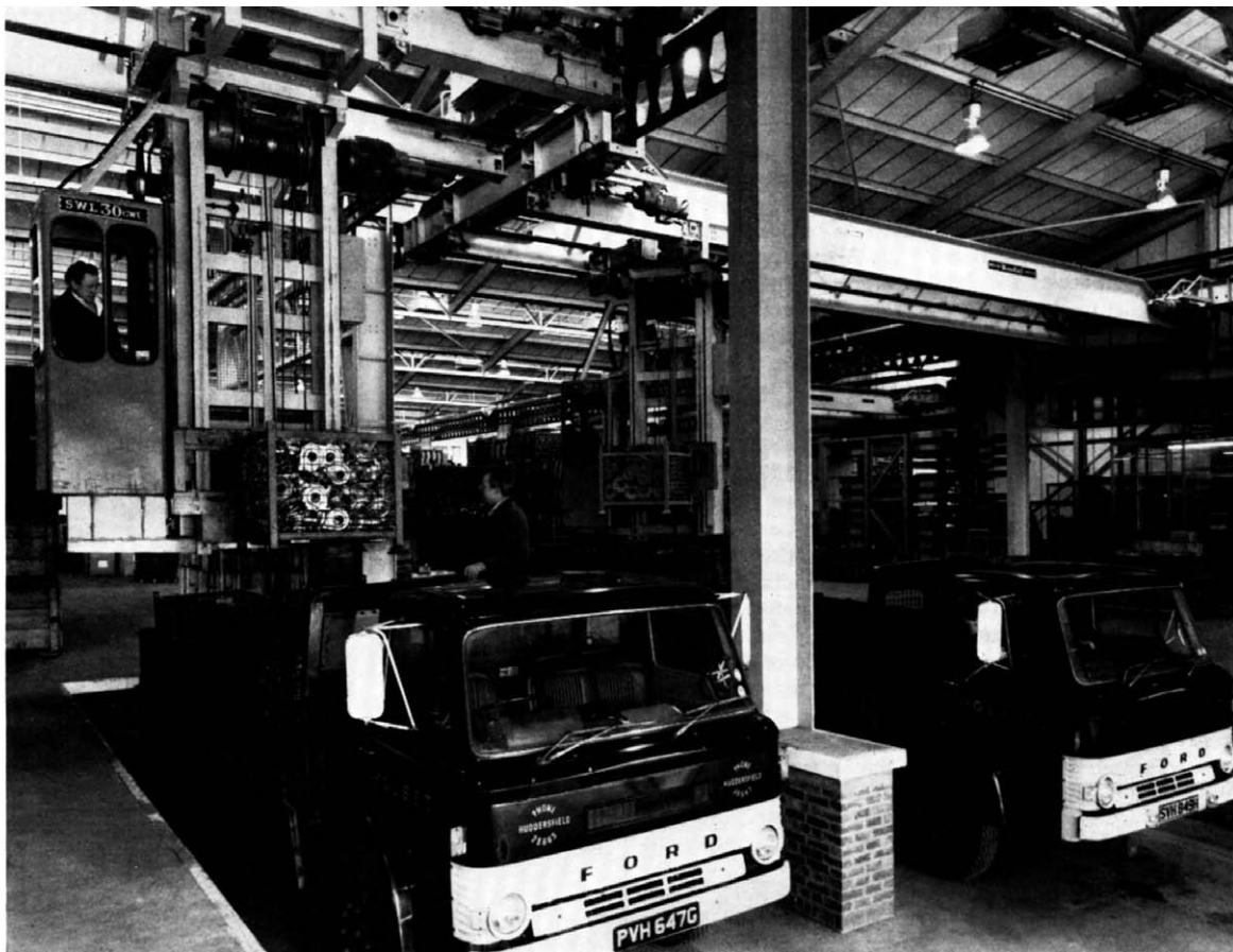
Figure 2.19 Daventry parts store, loading with overhead gantry-slung stacker cranes.
