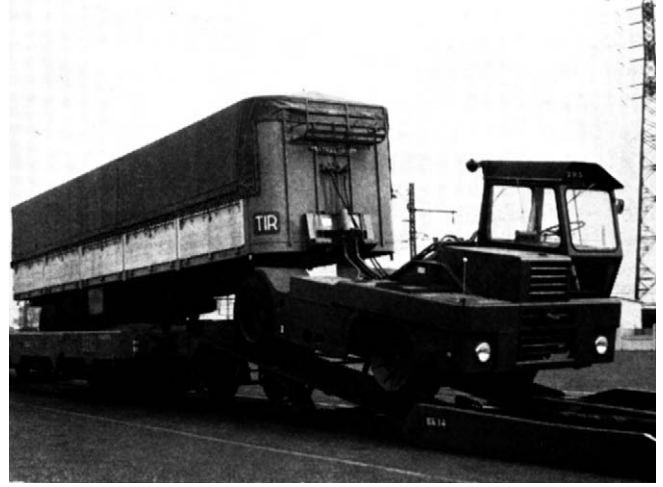
Figure 3.37 Kangaroo tractor loading trailer onto rail wagon.
