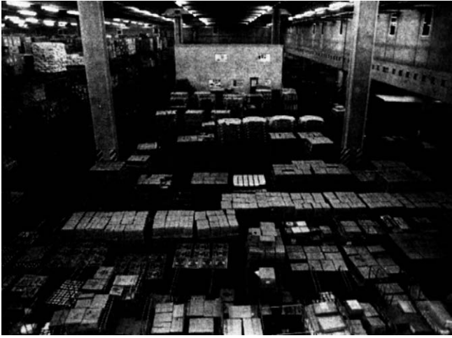
Figure 4.41 Load assembly area of large food distribution warehouse. Congestion occurs when incoming roll pallets meet full units seen here awaiting dispatch.
