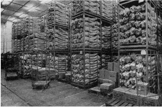
Figure 6.12 Special carcass pallets stacked three high in a cold store. Carcasses can be packed more compactly when flat than when hung.
