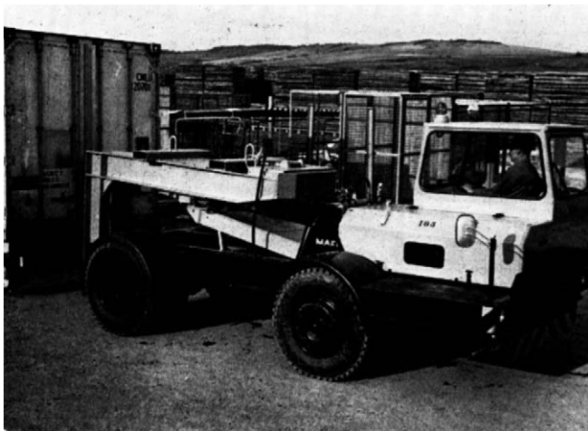
Figure 3.26 Tug towing stillage trailer with ISO container (see Figure 3.22).
