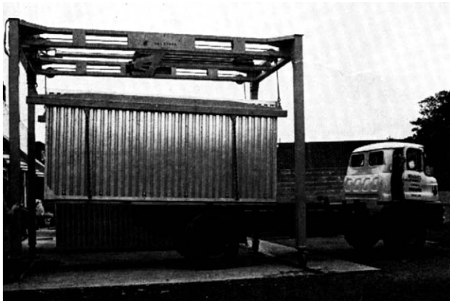
Figure 3.31 'Four-poster' mobile manual gantry.
