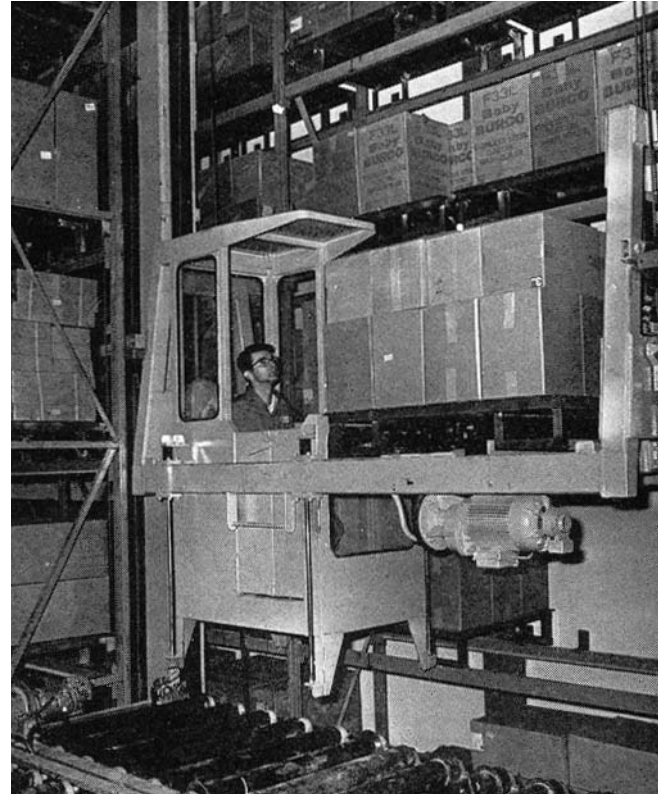
Figure 5.27 Free path machines like this are now being automated by wire guidance or light beams.
