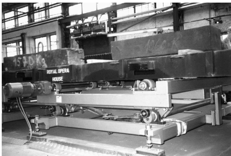
Figure 7.1 Scenery pallet during factory acceptance test. Note heavy duty conveyor system which will become an automated storage and sorting system.
