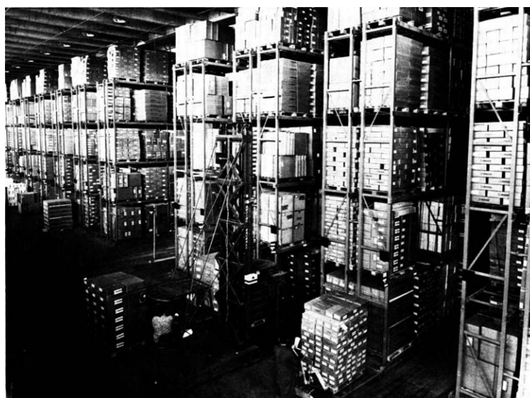
Figure 4.48 A big box structure allows both freedom in positioning racking and full height stacking.
