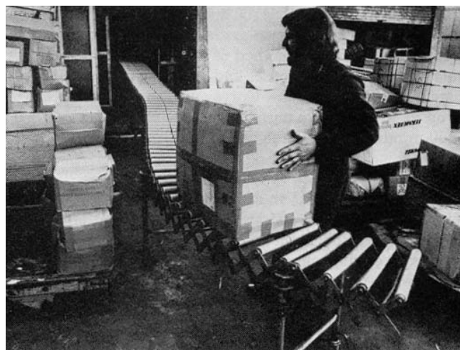
Figure 4.179 Extendible roller conveyor 'stuffing' truck.
