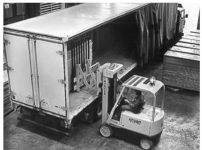
Figure 4.3 Forklift trucks with extending fork carriage discharging pallets from side loading curtain-sided trailer.
