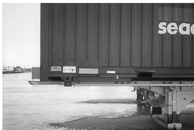
Figure 3.9 Two types of landing legs: the swop body's landing legs are folded up; the trailer's hydraulic legs are extended.
