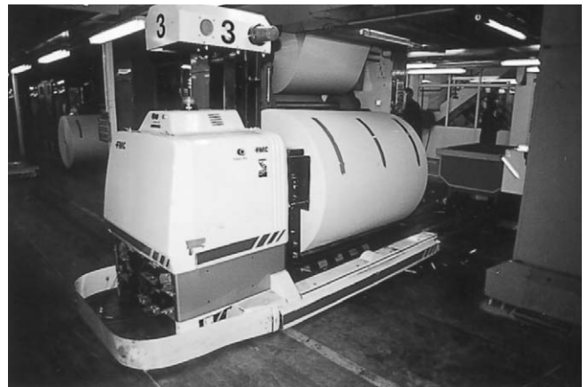
Figure 7.19 Automated guided vehicle handling new print reel stripped of barrier wrap direct to press spider interface. Similar heavier duty machines are now used for metal coils to slitting lines.
