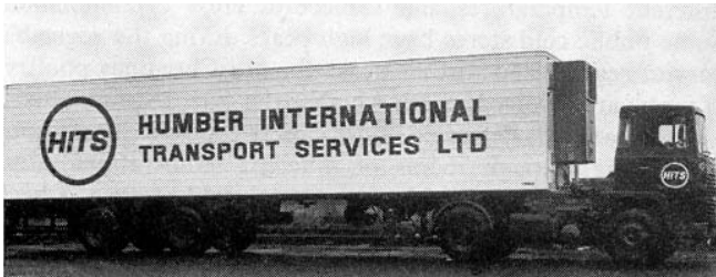
Figure 6.5 Refrigerated trailer with cooler on front.
