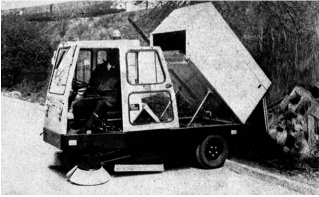
Figure 4.68 Mobile sweeper. Note the hoppers of these sweepers can lift to tip into a compaction skip: just tipping onto the ground is not acceptable!
