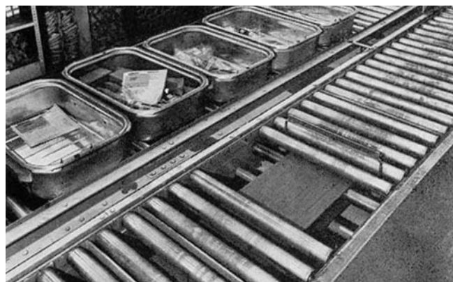
Figure 4.170 Powered roller conveyor.
