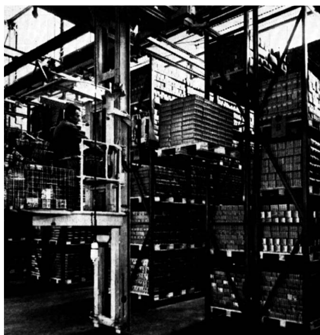
Figure 4.20 Gantry slung stacker/order picker. Allows narrow aisles but only one crane per gantry.
