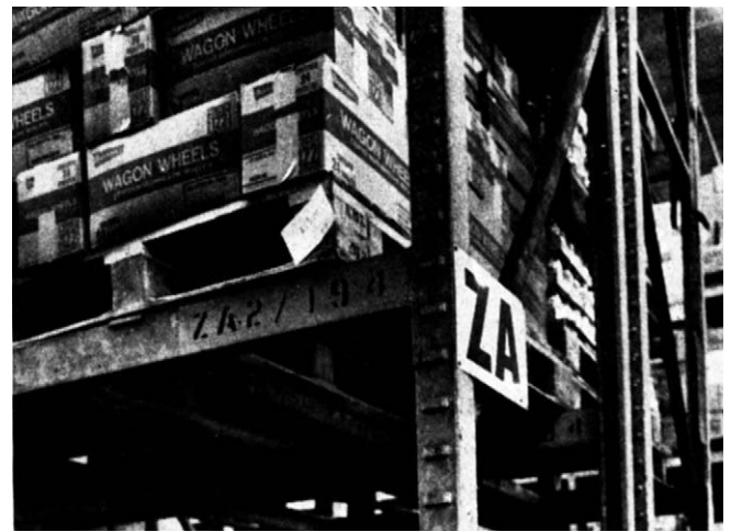
Figure 4.21 This shows the main rack code, ZA, and the pallet position code ZA2/194. The rack behind is numbered ZA1/194; i.e. transverse aisle pallets are numbered .../194 for identification. Also illustrates adjustable pallet racking.
