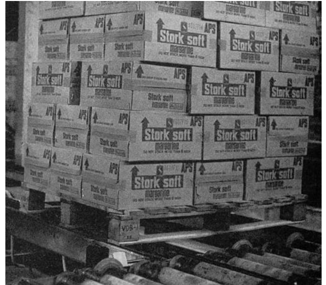
Figure 5.14 This pallet has a broken corner. Timber resin leaves a deposit on the rollers that may drop off and affect the mechanical equipment.
