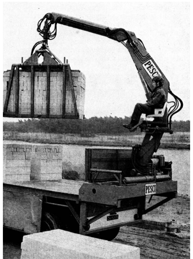
Figure 3.35 Typical sliding trailer loading crane. Useful for many general purpose goods.
