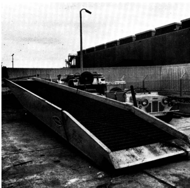
Figure 2.17 Loading ramp for forklift trucks.
