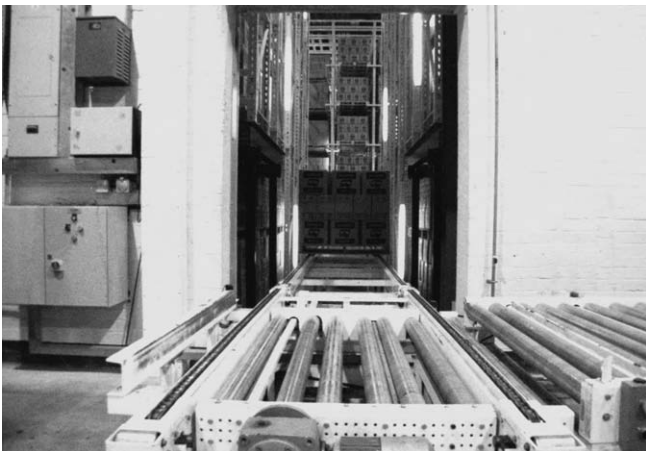
Figure 4.199 A 90° direction change. Note rollers sink to deposit pallet onto chains running in opposite direction.
