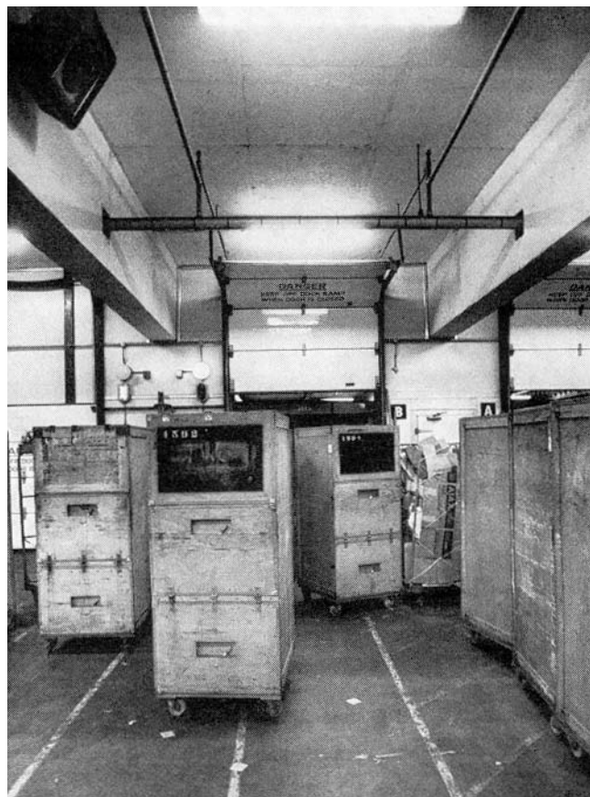
Figure 6.15 Incoming empty insulated roll pallets being pushed out of the vehicle to the left insulated. Full dispatch units waiting for loading on the right. Channels are clearly marked, and loading bay door is insulated. Incoming units may constrict dispatch units in peak conditions in dual-purpose docks.
