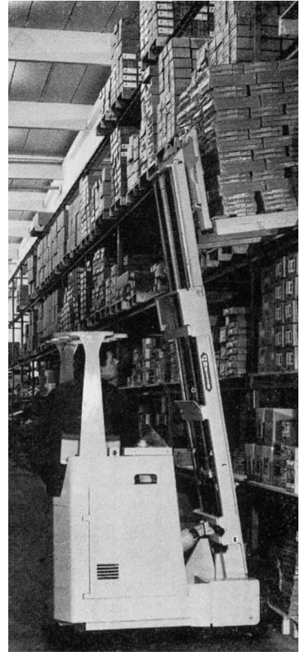
Figure 4.141 Narrow aisle stacker truck: a forklift with no reach action, relying on mast angle and short dimensions to reduce aisle space; often used in smaller stores.
