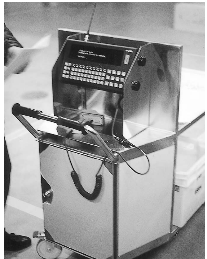
Figure 4.22 Radio data terminal mounted on picking cart: note screen giving location and description and bar code wand for proof of pick.
