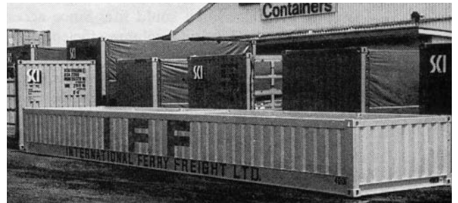
Figure 7.3 Open, half height container used for carrying steel.
