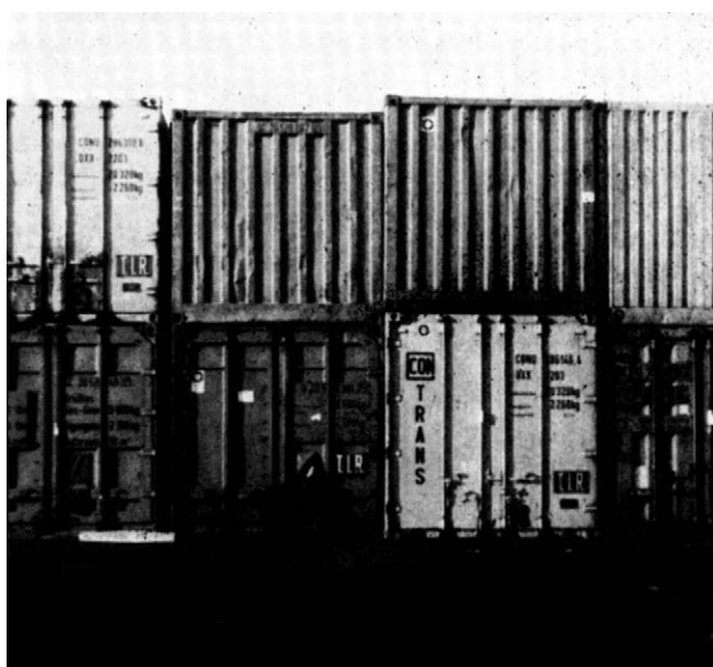
Figure 3.1 Different heights of ISO containers makes stacking difficult.
