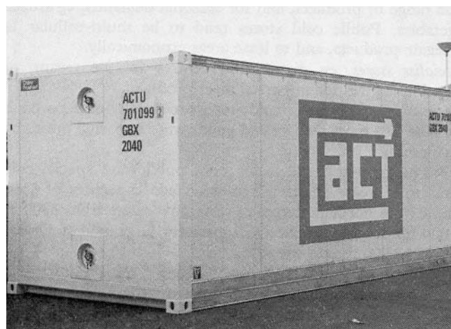
Figure 6.3 Reefer container, which must be connected to cooling source (i.e. non-autonomous).
