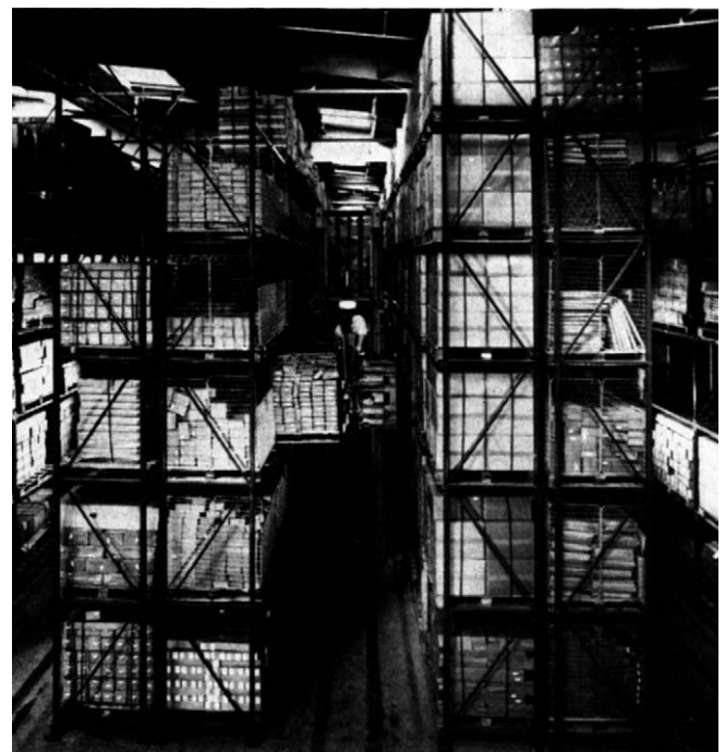
Figure 4.108 In many cases, nearly as much space can be gained by using narrow aisles and high lift machines as by more expensive mobile racking and general purpose reach trucks. Compare with Figure 4.110.
