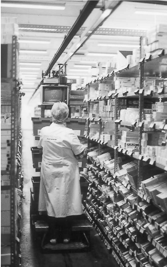
Figure 4.84 'Live' shelving in a pharmaceutical warehouse. Note inclined track with barcode labels and 'pick car'.
