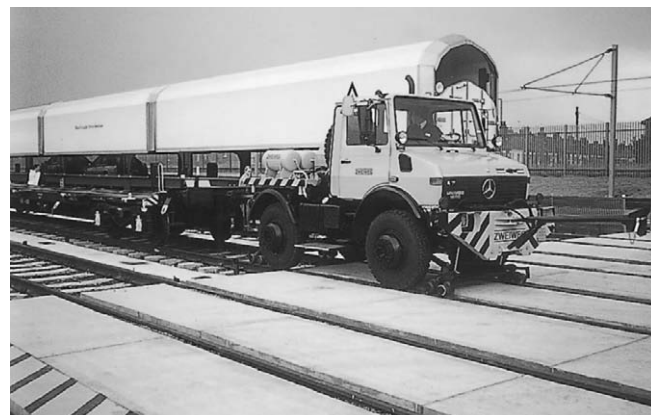
Figure 2.73 A Unimog road/rail tractor used in local depot shunting.
