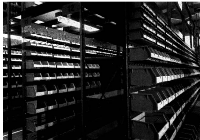
Figure 4.75 Louvre panels used in high-density storage.
