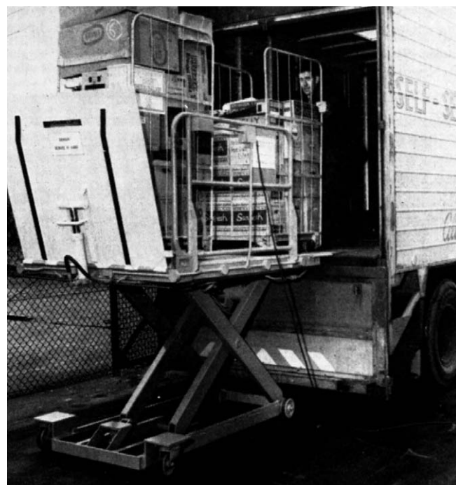
Figure 2.63 Mobile dock leveller loading roll pallets.
