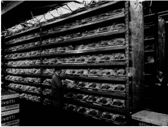
Figure 4.82 Long span adjustable shelving.
