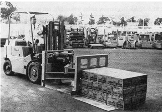
Figure 4.133 Push/pull attachment in extended position with load on slip sheet about to be withdrawn onto platen arms.
