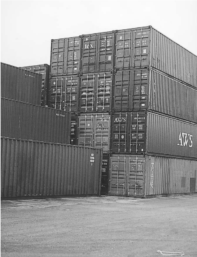
Figure 3.13 Containers can be stacked four high, three deep, by a reach stacker, by loading progressively from the rear.
