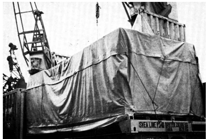
Figure 3.29 Stillage trailer with ISO 'flat' for loads unsuitable for containers for roll-on/roll-off use.
