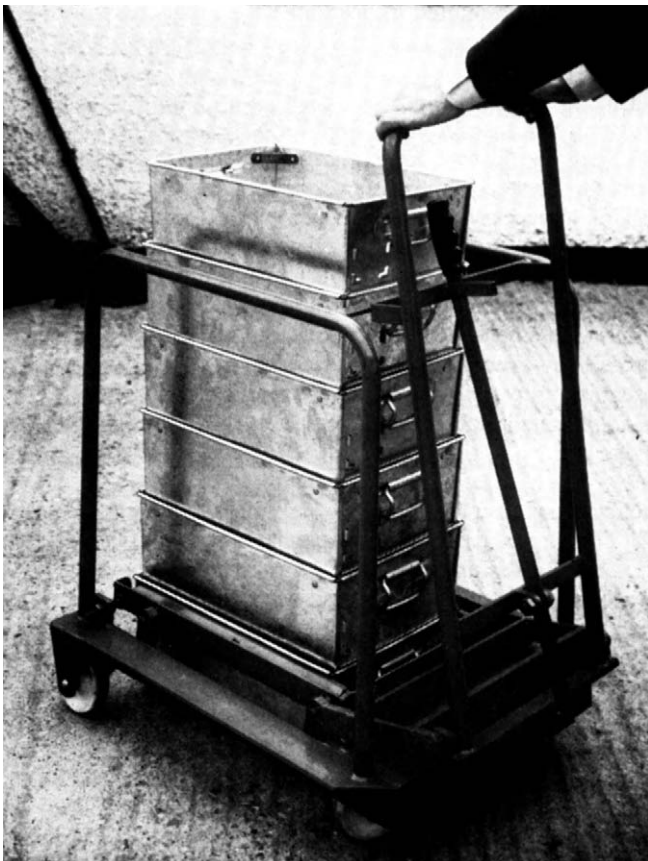
Figure 4.72 Stacked metal tote boxes.
