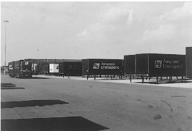
Figure 3.6 Swap body interchange park. Note truck and drawbar trailer for maximum cubic capacity.
