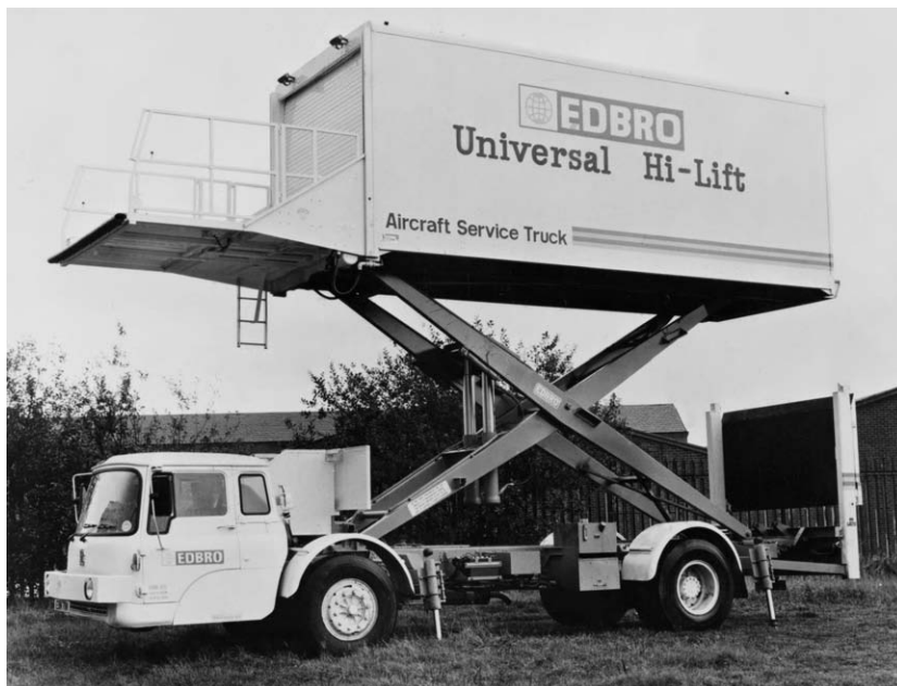
Figure 1.12 Container is lifted to load directly into aircraft deck.
