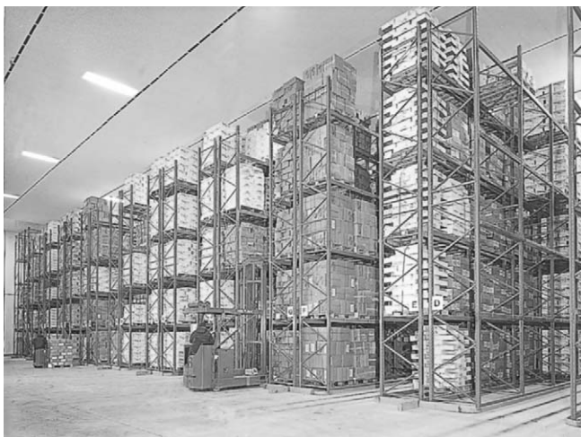
Figure 6.16 Nine metre clear height (manned) cold store with narrow aisles. Fully automated versions are built at three times this height.
