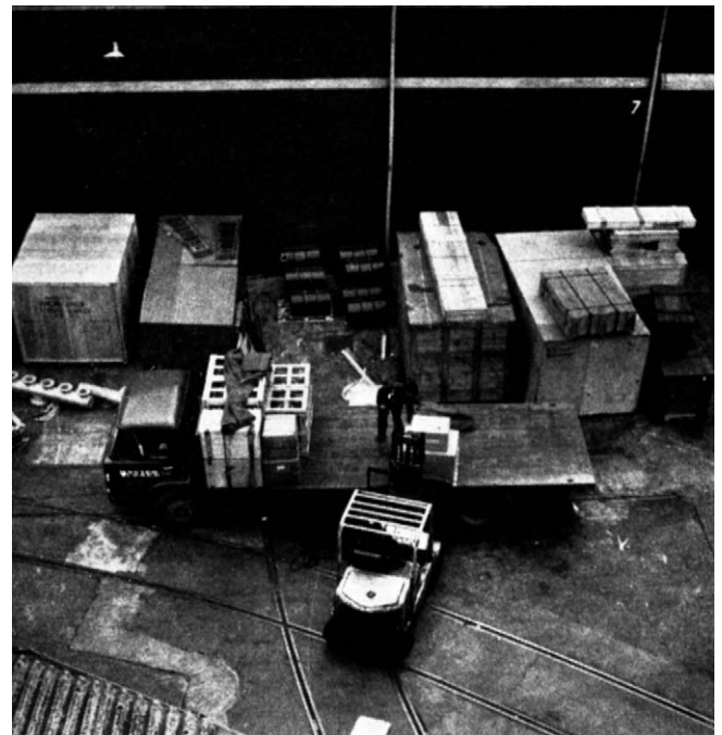
Figure 2.11(a) When a truck stops to load it constricts the road. Manoeuvring forklift trucks then block it completely. Externally stacked goods impede loading on both sides.
