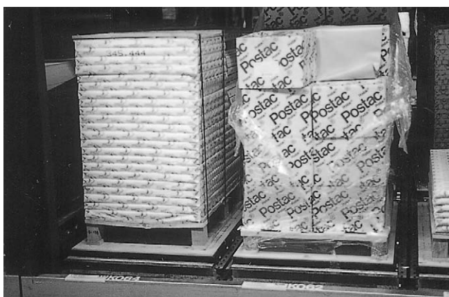
Figure 4.18 'Live racking' at the picking end. Note pallets on 'plattens' for smooth running on the incline.
