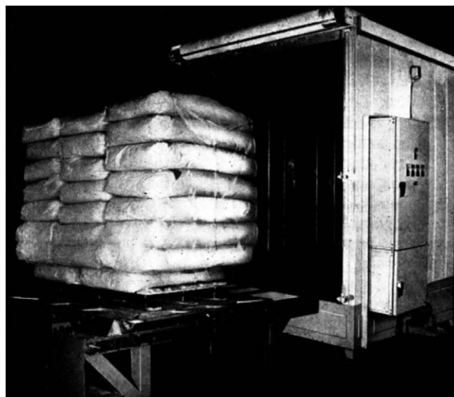
Figure 4.39 Shrink-wrapped palletized load emerging from shrink-wrap tunnel.
