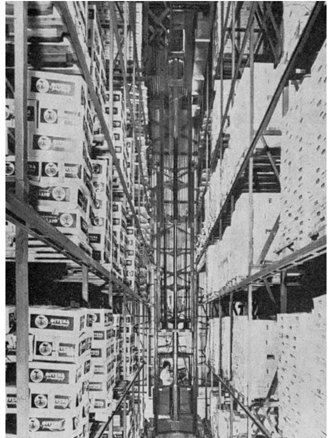
Figure 5.40 Free-path, high-rise machine (here semi-automatic). Floors have to be constructed to very tight tolerances (Class 1).
