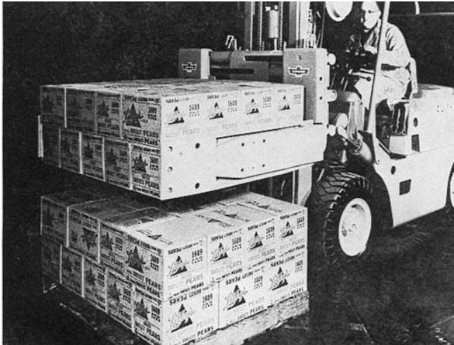
Figure 4.132 Turning fork attachment with arms set in load clamping position.
