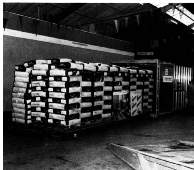
Figure 2.16 Roll-in system allows container to be loaded in one movement.
