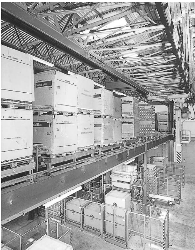
Figure 4.155 Gantry slung stacker crane – effectively an upside-down forklift.
