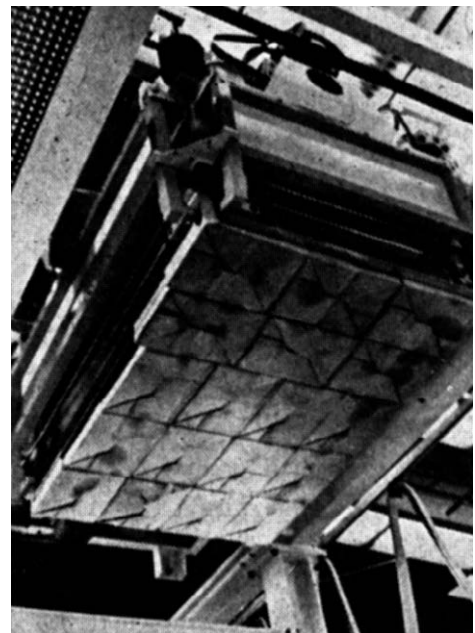
Figure 4.60 Manually operated vacuum palletizer.
