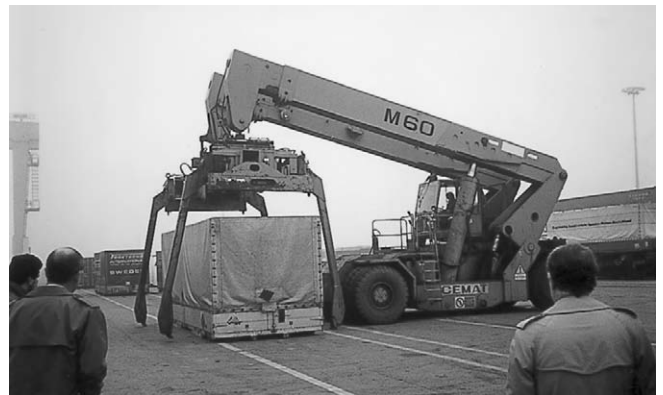
Figure 3.38 Trailer being lifted by reach stacker. Note clearly marked lanes for load transfer.
