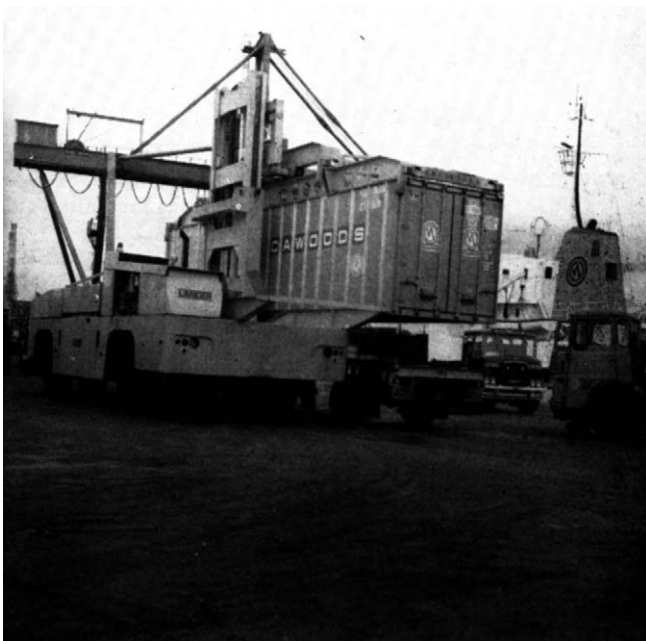
Figure 3.19(a/b) Sideloader placing container onto vehicle trailer.
