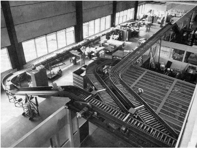
Figure 4.198 A conveyor system serving a three level mezzanine storage system leading to the dispatch sorting area.
