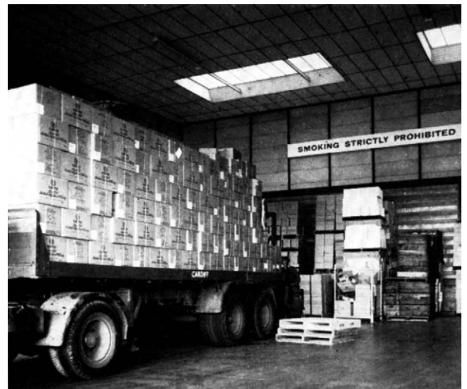
Figure 2.6 Hand-stacked load of bulk cartons, loaded over the side from forklift truck. Still used in developing economies.
