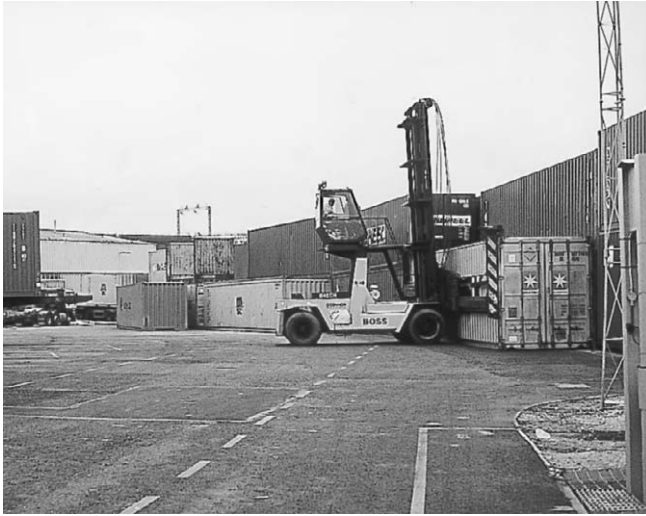
Figure 3.18 Note raised cab for driver vision.
