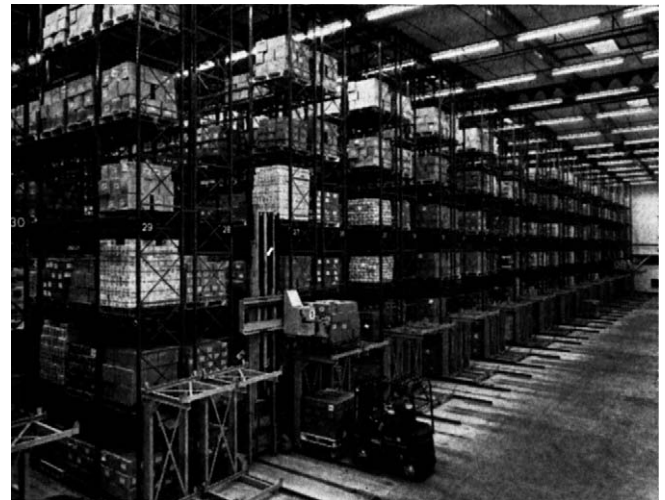
Figure 4.17 Transfer position between turret truck and forklift from loading bay known as a P&D station.
