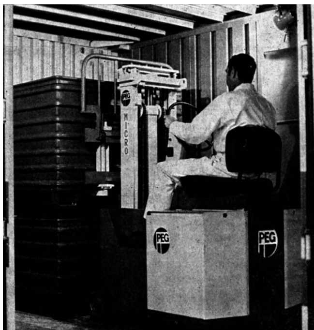
Figure 4.113 Bins to modular pallet dimensions loaded into container by forklift.
