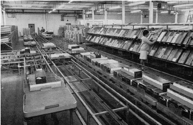
Figure 5.29 Cartrac transporters being used as both transport and as order-picking carousel.
