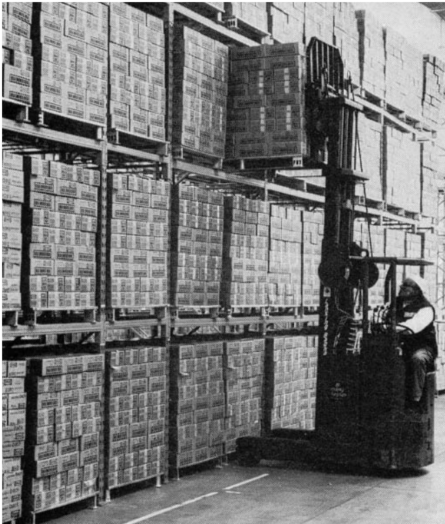
Figure 6.13 Reach truck being used in a cold store for bacon. Standard machines can be used after modifications to the electrical and hydraulic systems.
