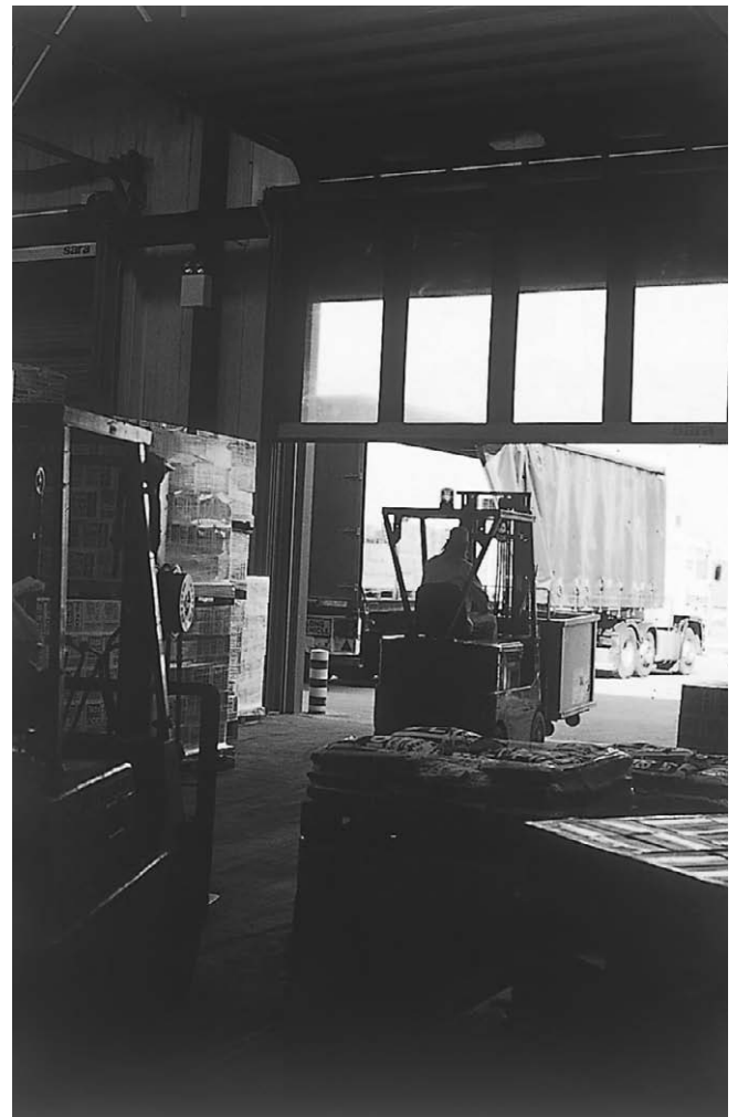
Figure 2.53 Fast door between a load assembly area and external loading bay; here it is rising as the forklift approaches it.
