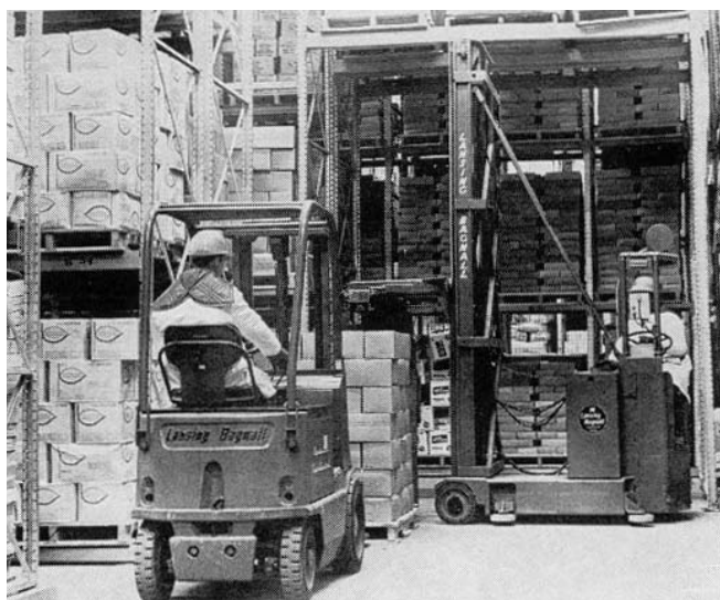
Figure 6.27 Forklift delivering frozen pallet from the truck dock to turret truck operating the narrow aisle warehouse.
