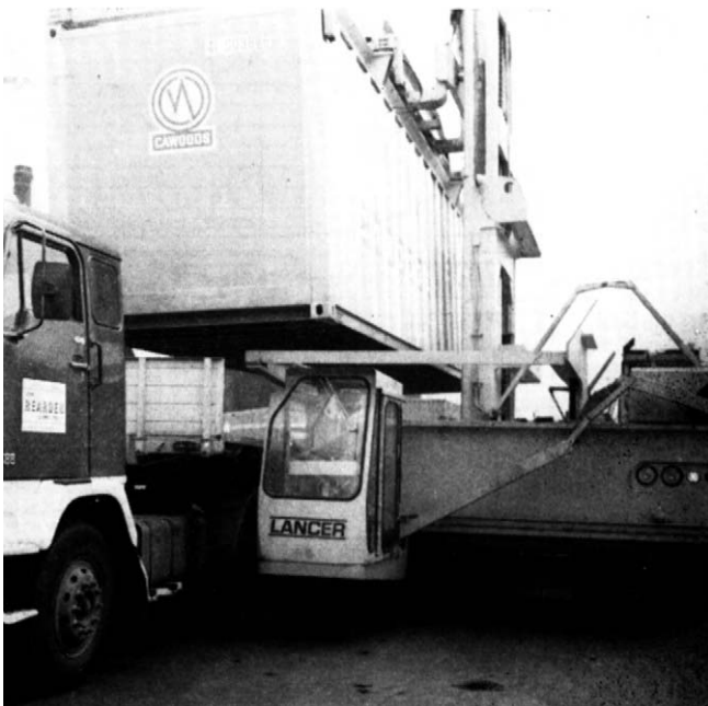
Figure 3.18 Note raised cab for driver vision.
