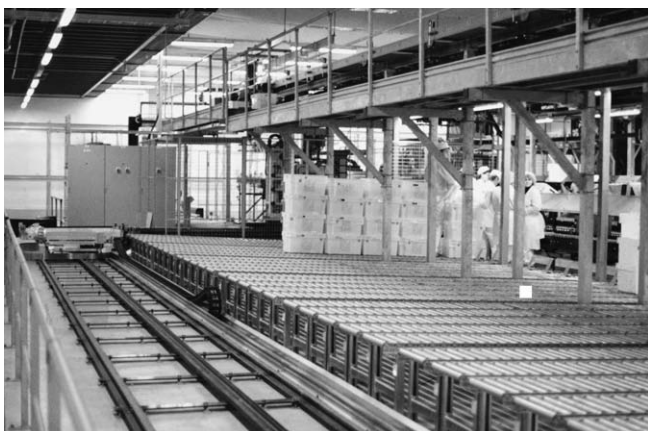
Figure 5.49 Shuttle car with festoon cable in low profile chain.
