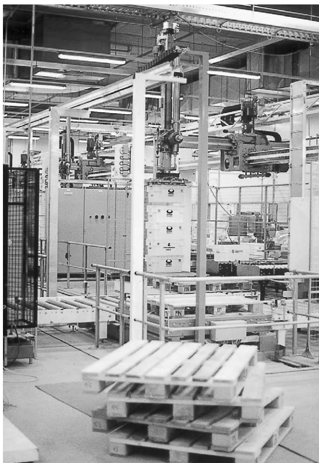
Figure 4.37 Gantry robot for palletizing crates of meat.
