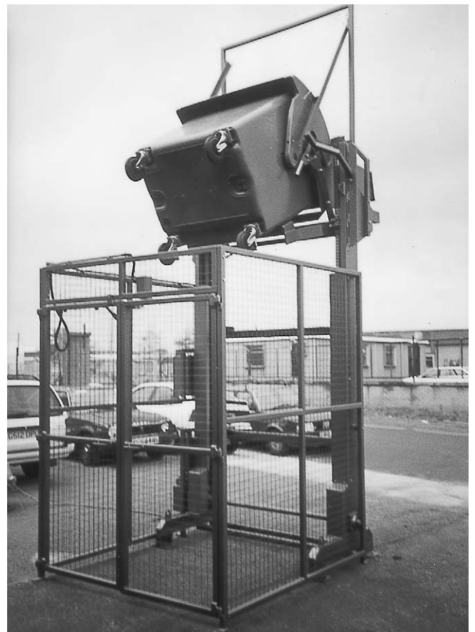
Figure 2.44 Device for tipping 1100 litre bins into compactor.
