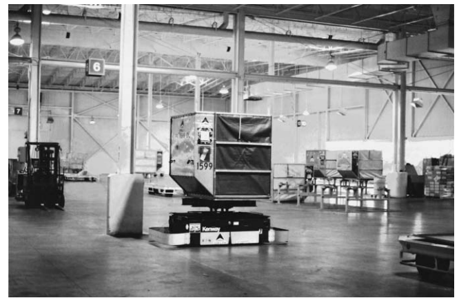
Figure 5.44 AGV with container – note transfer P&D stations at right.
