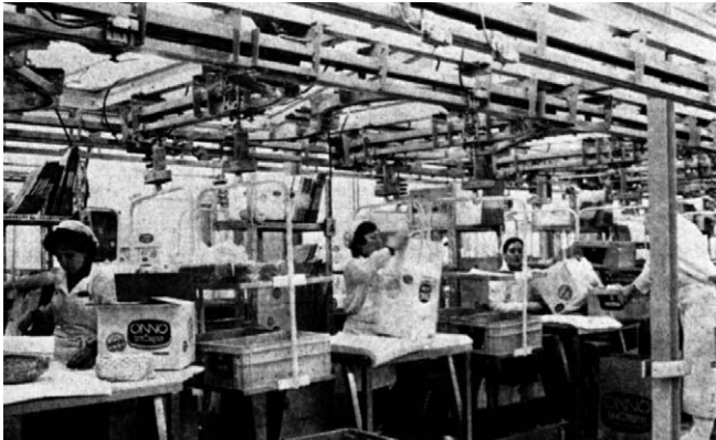
Figure 4.65 Manual packaging with overhead conveyor.
