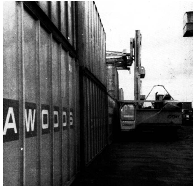
Figure 3.20 Sideloader stacking containers in parallel.
