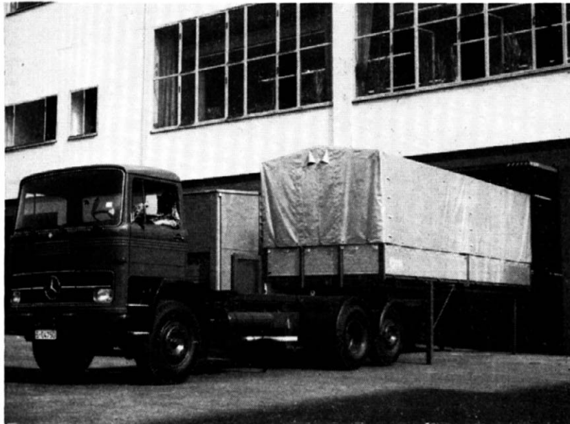
Figure 1.11 This lorry is leaving its swap body on mounted legs at loading bay, and is now ready to receive another.
