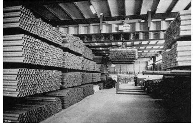
Figure 4.160 Gantry crane using special stillages for storing pipes on for tree racking.
