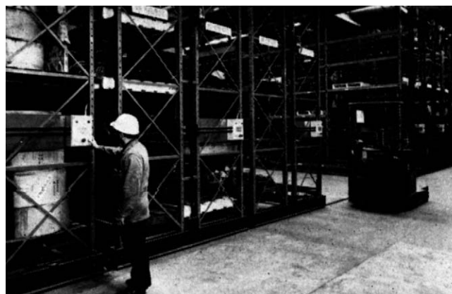
Figure 4.110 Manually-operated rack opening mechanism.
