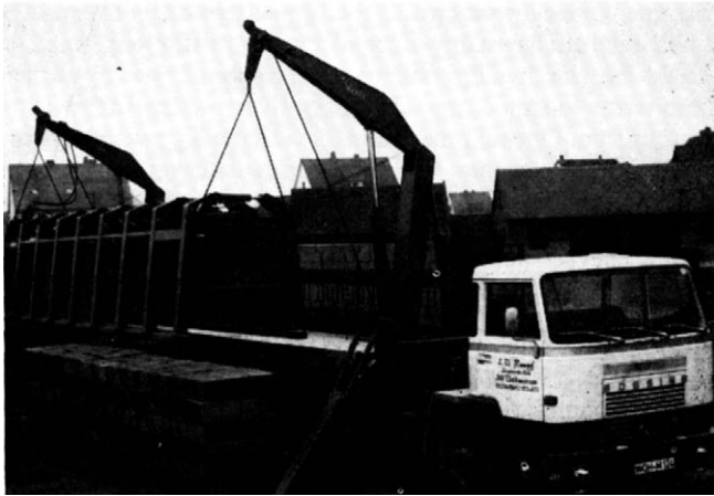
Figure 1.9 Hydraulic clamp covering whole length of semi-trailer's platform, for handling bricks.
