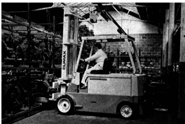
Figure 4.62 4500 kg capacity forklift working in assembly plant buffer store.
