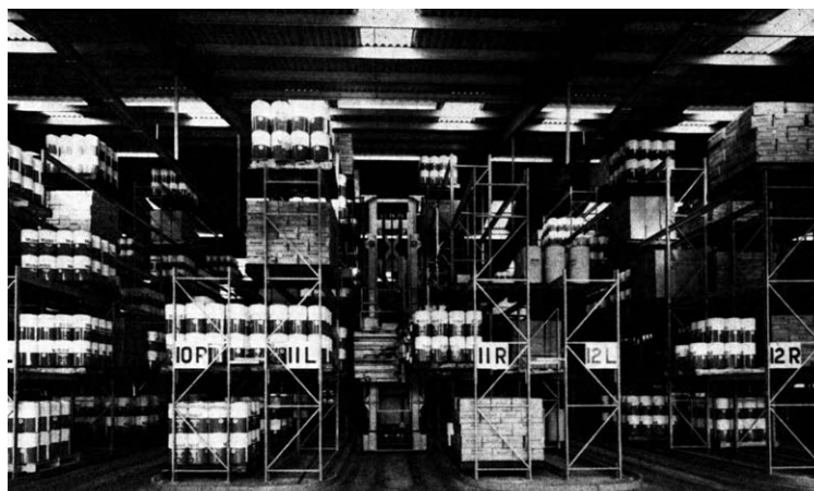
Figure 4.47 The roof structure of a warehouse can cause a pallet position to be lost throughout the length of a whole aisle at each turn position.
