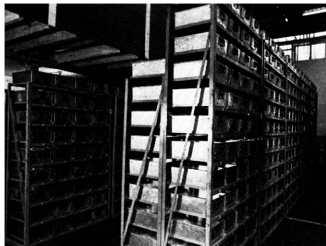
Figure 4.76 Simple steel shelving for metal tote boxes.
