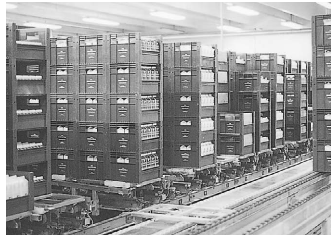
Figure 4.200 Manually propelled system that both transports and acts as inter-process storage medium. By depressing a foot pedal units can change direction of travel from one set of rails to another at 90°. Stacks of crates on accumulation conveyors (left) are transferred by a special handling unit to the take-away chain conveyor (right).
