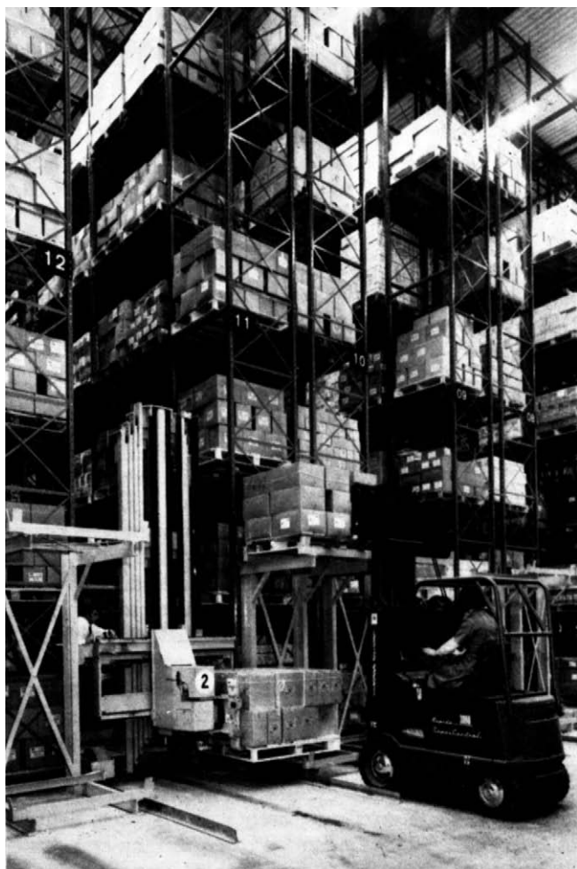
Figure 2.15 The small forklift exchanges loads with a turret truck at the buffer zone.
