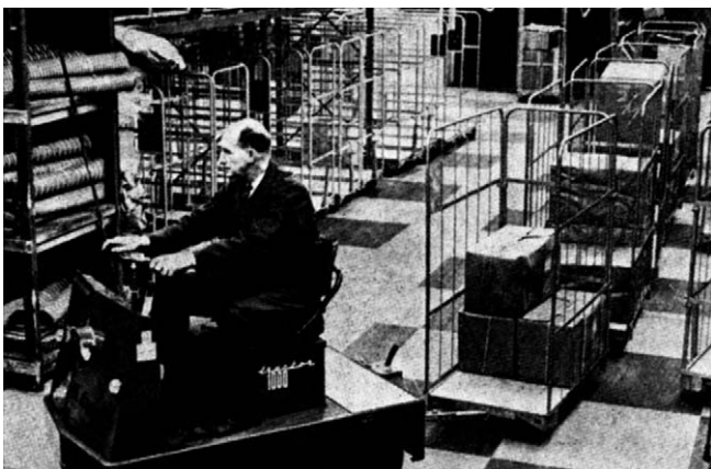
Figure 4.66 Tow tractor pulling roll pallets to sorting area.
