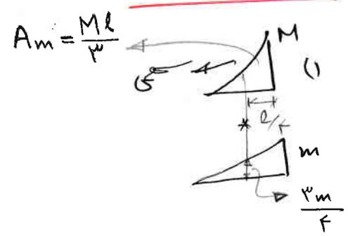
$$\int \frac{M(x)m(x)dx}{EI} = \frac{\frac{Ml}{3} \times \frac{m}{3}}{EI} = \frac{Mml}{9EI}$$
