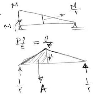
$$\Delta = \frac{l}{7EI} \left[ \frac{1}{2} M(0) + \frac{1}{2} \frac{M}{r} \times \frac{l}{r} + M \left( \frac{l}{r} \right) + \frac{1}{2} \frac{M}{r} (0) \right]$$
