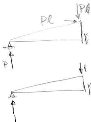
$$1 \times \Delta_B = \int \frac{M(x)m(x) dx}{EI} = \frac{Pl \times l \times l}{3EI} = \frac{Pl^3}{3EI}$$
