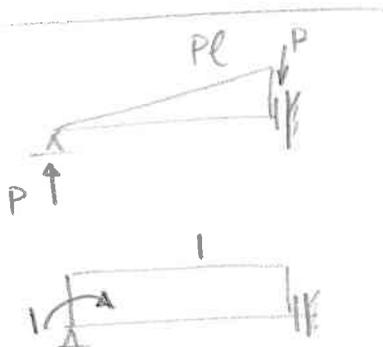
$$1 \times \theta_A = \int \frac{M(x)m(x) dx}{EI} = \frac{Pl \times l \times l}{2EI} = \frac{Pl^2}{2EI}$$
