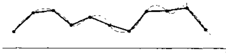
Figure 7.9 Linear interpolation between sample points. The dashed curve represents the original signal and the solid curve the linear interpolation.
