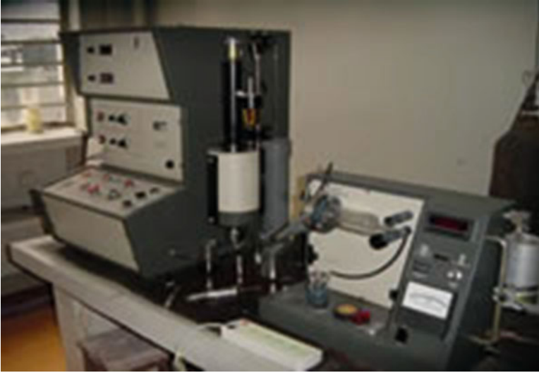
Fig. 4.16 Automatic mercury analyzer AUTOSCAN 60
