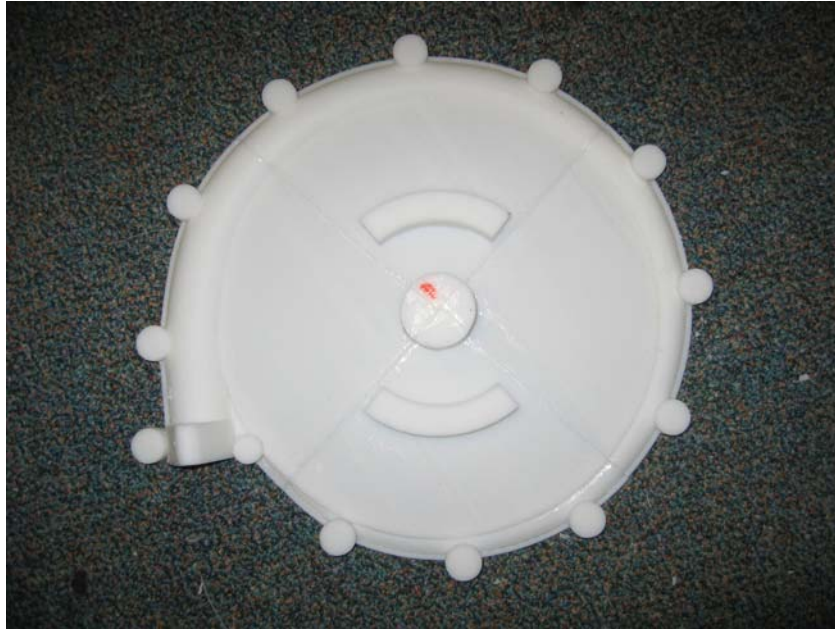
Figure 18 The FDM-ABS pattern as fabricated
