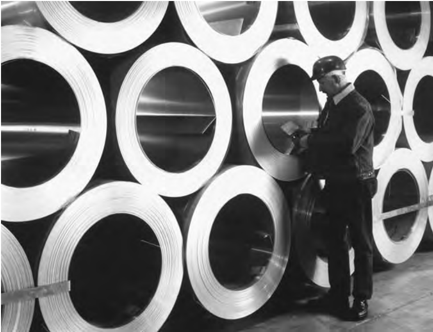
Figure 3.13 Aluminum sheet may be purchased in coil form. This allows pieces to be cut or nested to suit fabrication requirements, thereby reducing waste. (Courtesy of Temcor)
